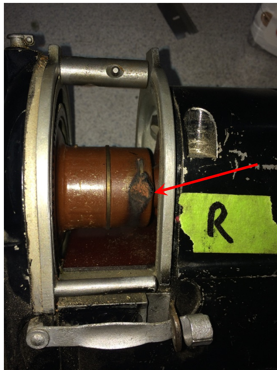
Photograph 8: Right Magneto (note burn spot)
