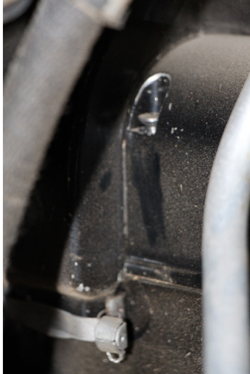
Photograph 3: Left Magneto Top Cover Retaining Screw
