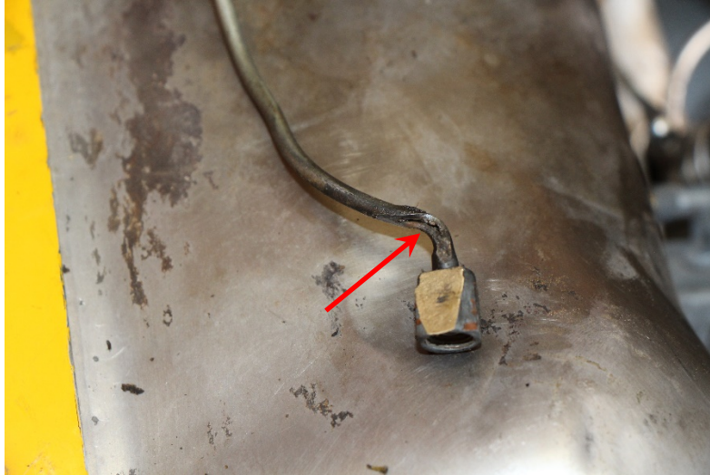
Photograph 7: Cylinder No. 1 Fuel Primer Line (note tear)
