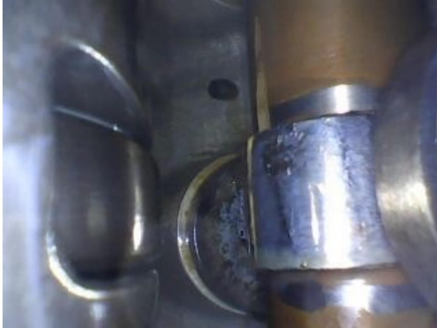
Photograph 3 – Intake Valve Camlobe from Cylinder no. 6
