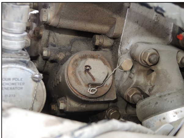
Figure 7-Right engine oil screen cap and safety wire.
