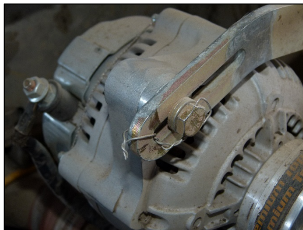
Figure 8-Right engine alternator safety wire.
