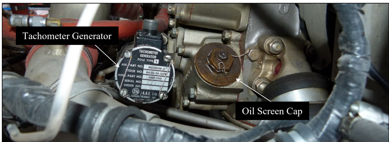
Figure 6-Left Engine tachometer generator and oil screen cap safety wire.
