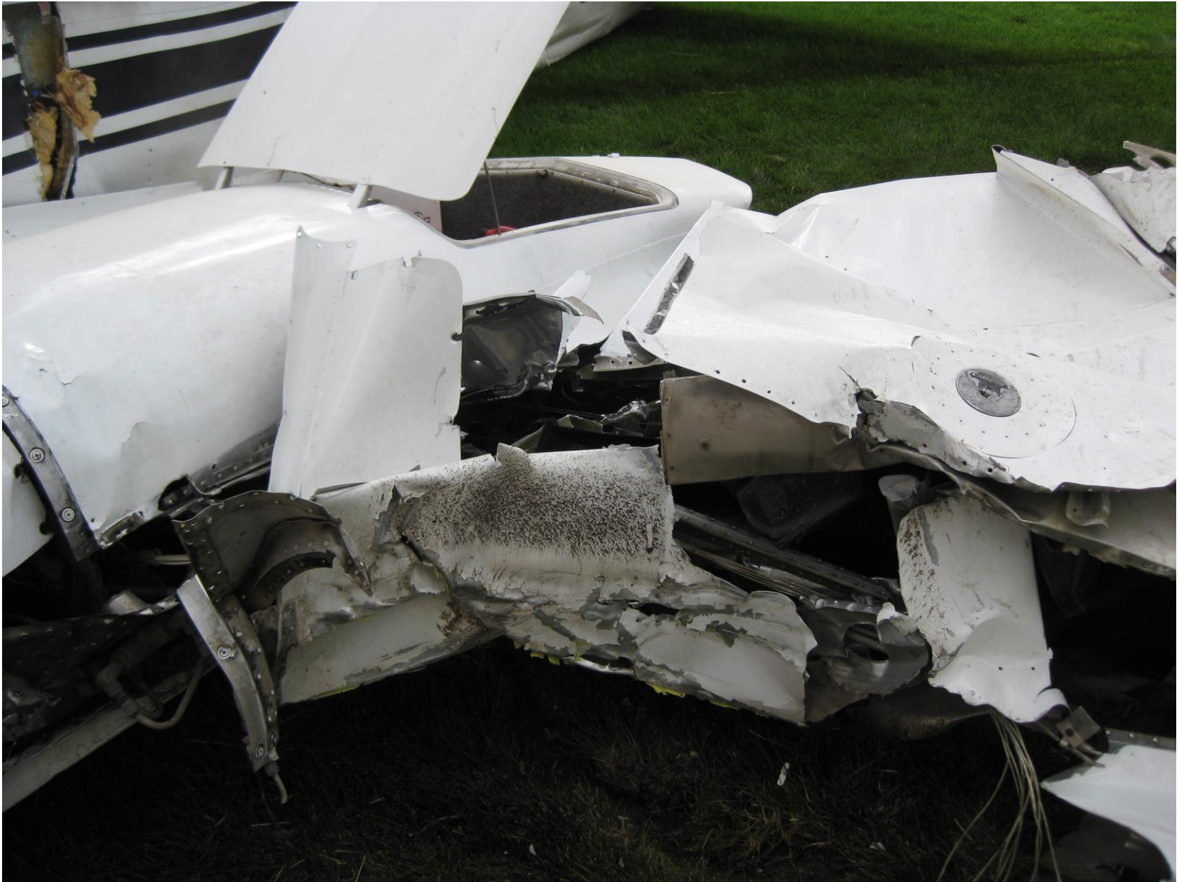
Photo 17 – Left wing damage.
