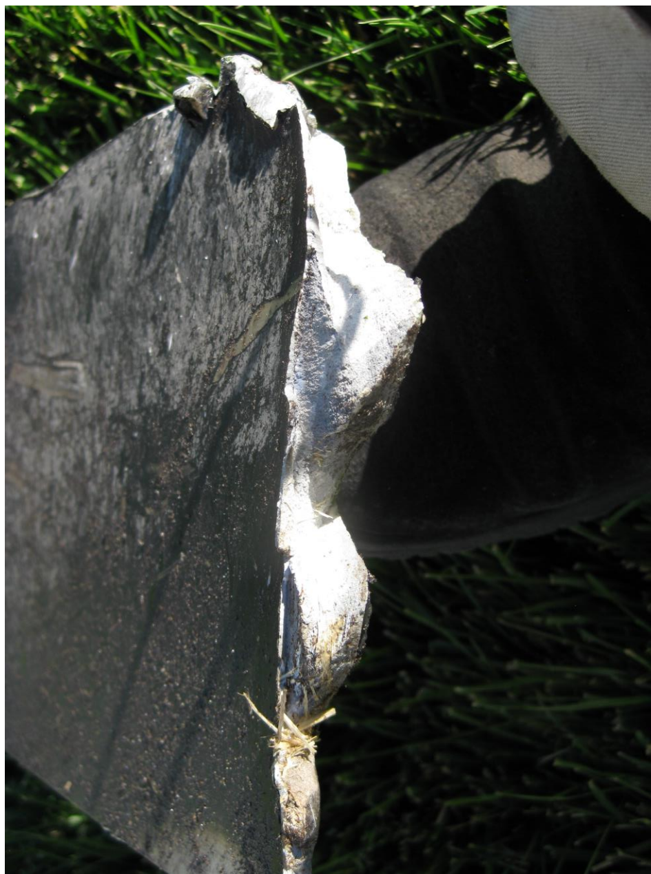
Photo 18 – Right propeller blade separation.
