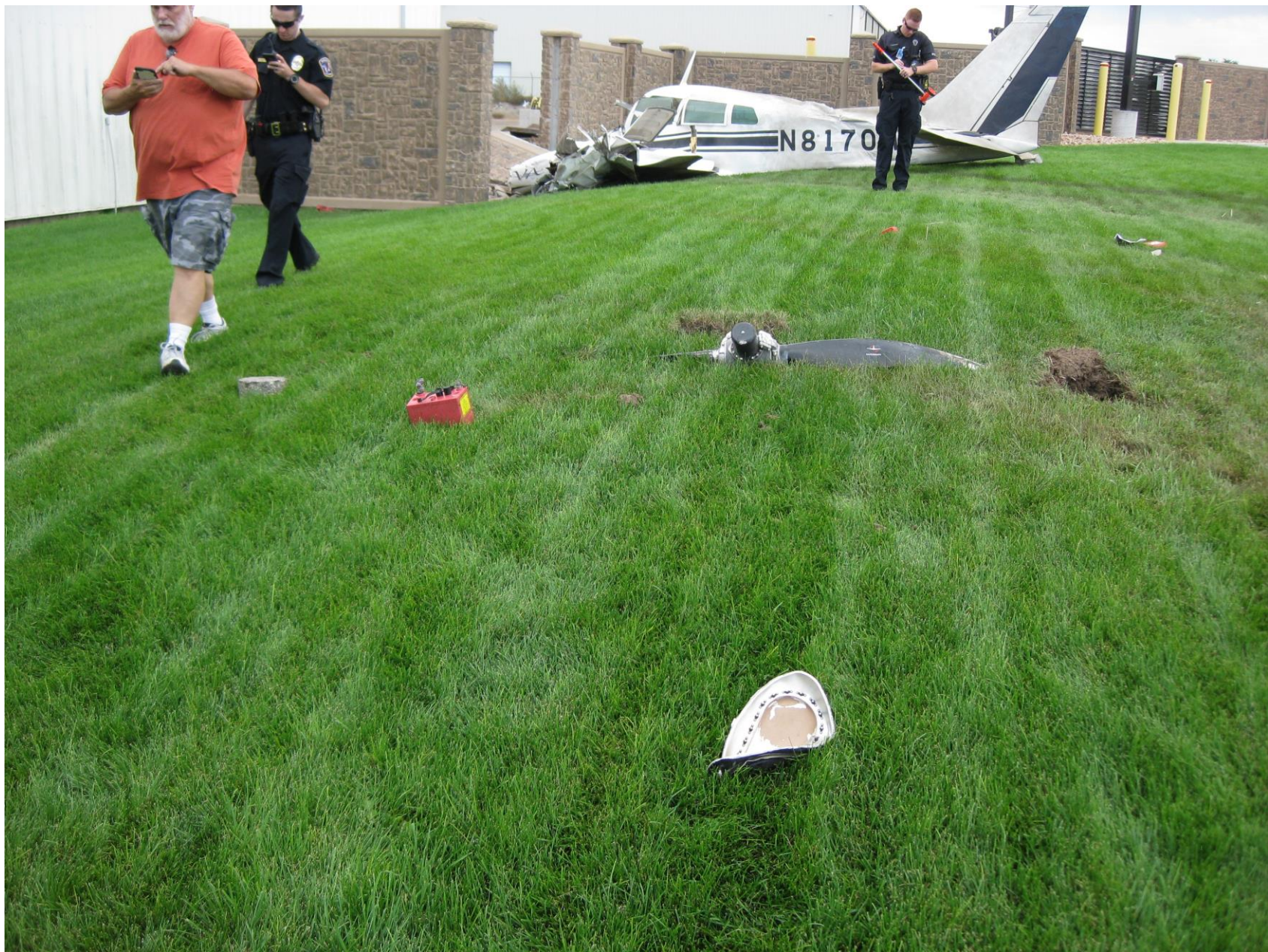
Photo 9 – Left propeller assembly and main wreckage.
