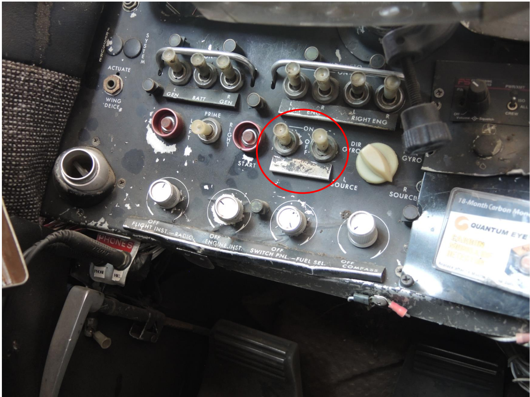
Photo 2 – Auxiliary fuel pump switches (centered).
