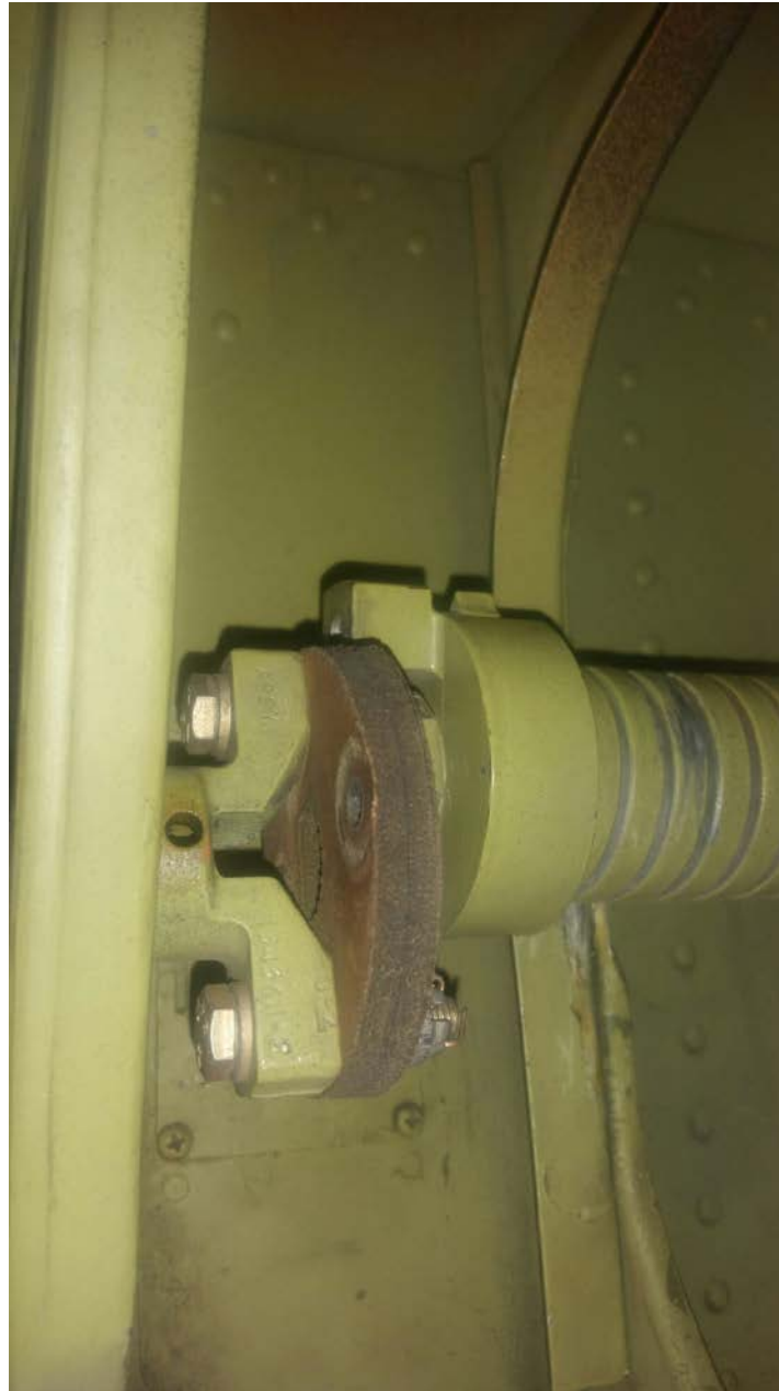
Photo 2 – Left Hand Varicam Drive Stop Coupling and Yoke (Courtesy of Neptune Aviation)
