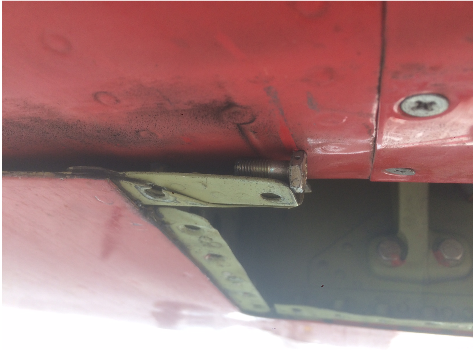
Photo 4 – Missing Left Hand Varicam Drive Stop Coupling AN174H7A Bolt (Courtesy of Neptune Aviation)
