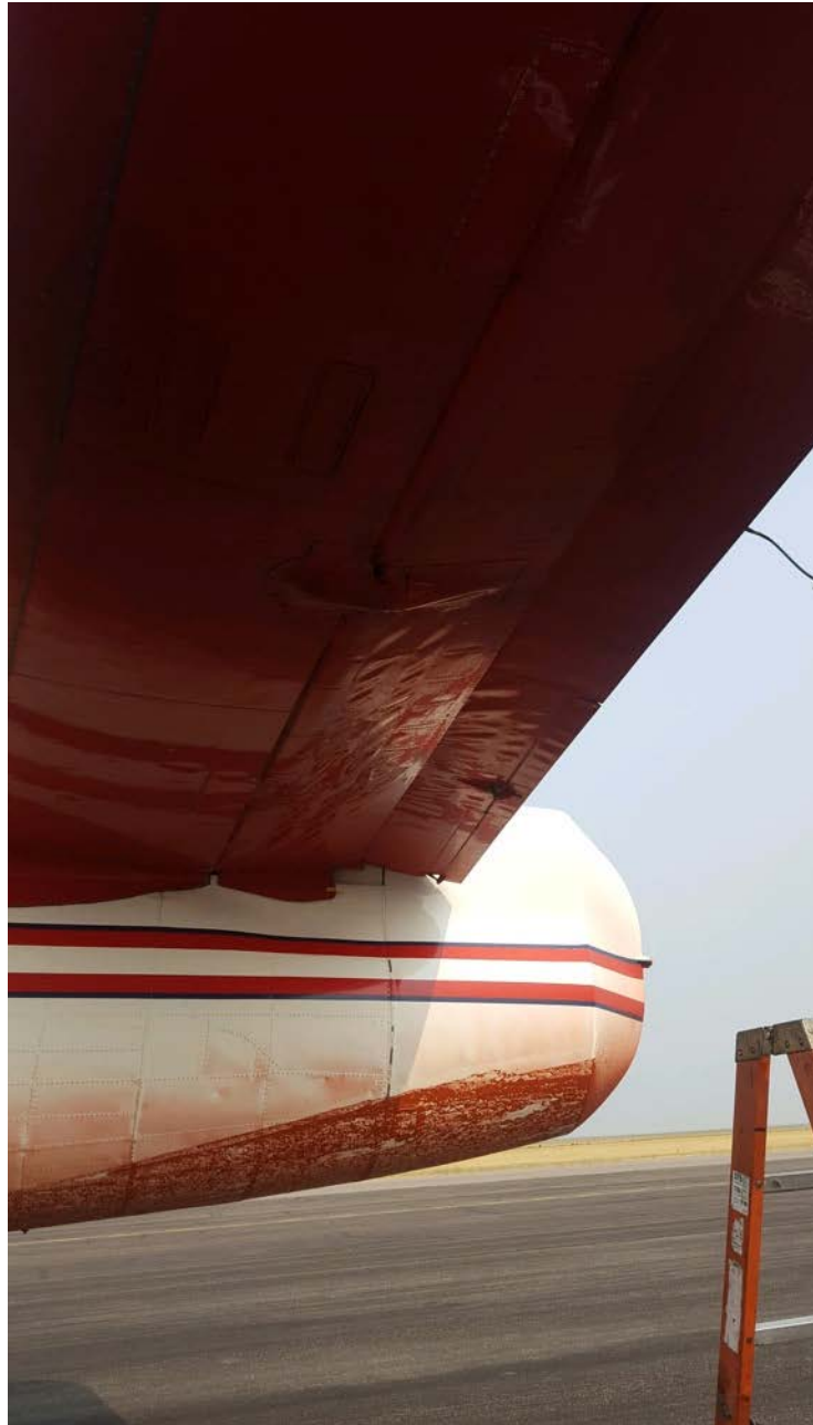
Photo 1 – View of Lower Left Hand Varicam (Courtesy of Neptune Aviation)
