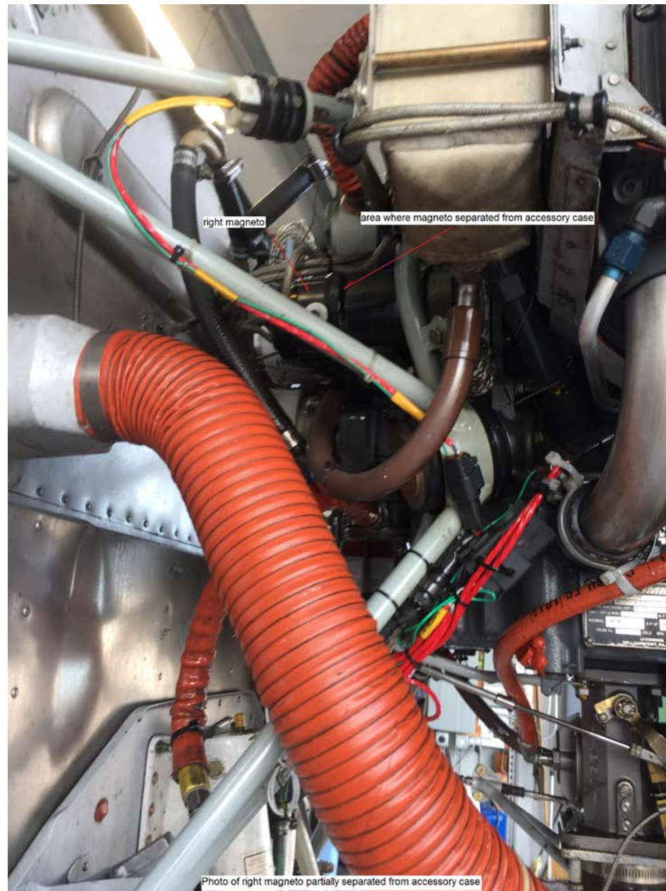
Photo 3 – photo of right magneto partially separated from accessory case mount
