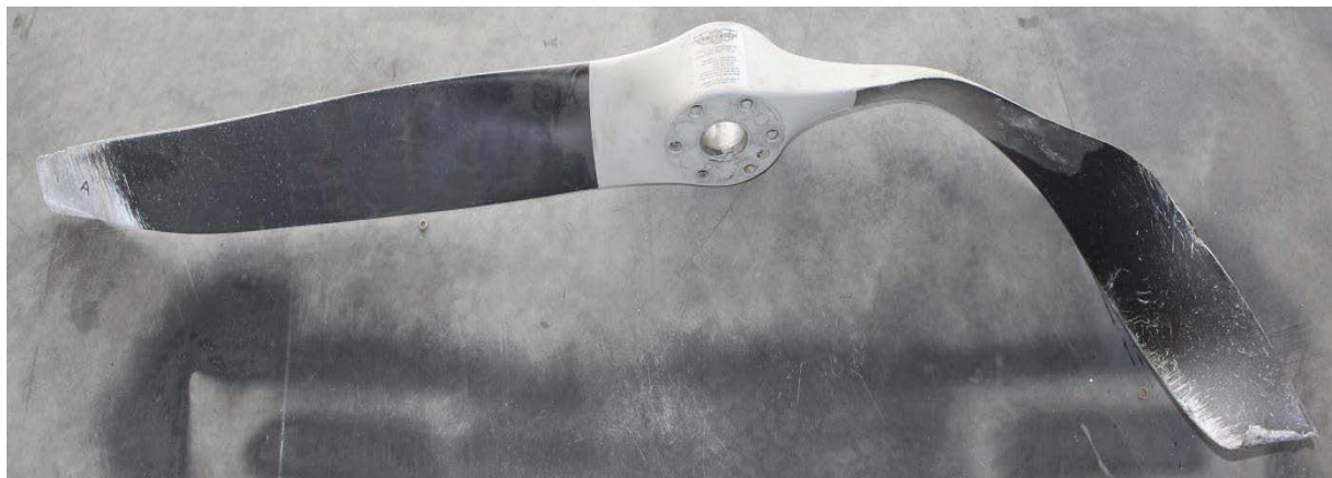
Figure 2 - damaged propeller blades
