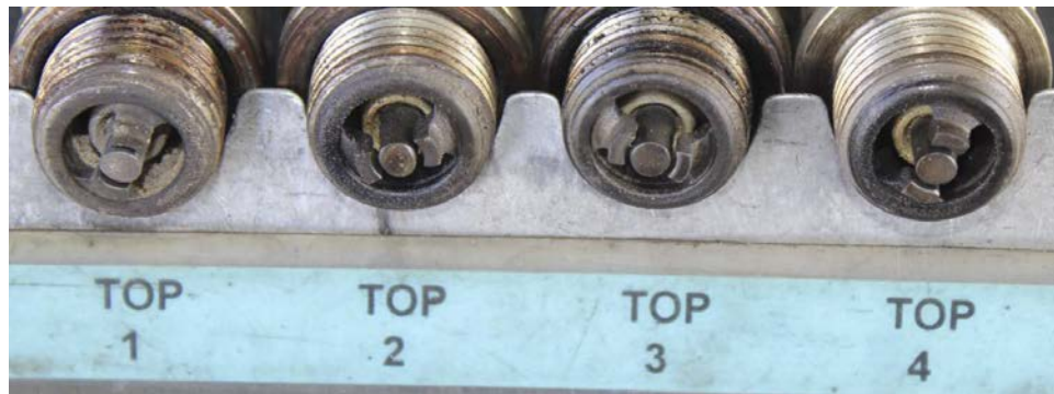
Figure 3 - condition of upper spark plugs
