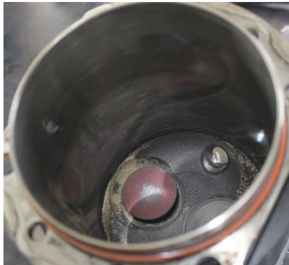
Figure 5 - view 1 of number 3 cylinder and stuck exhaust valve
