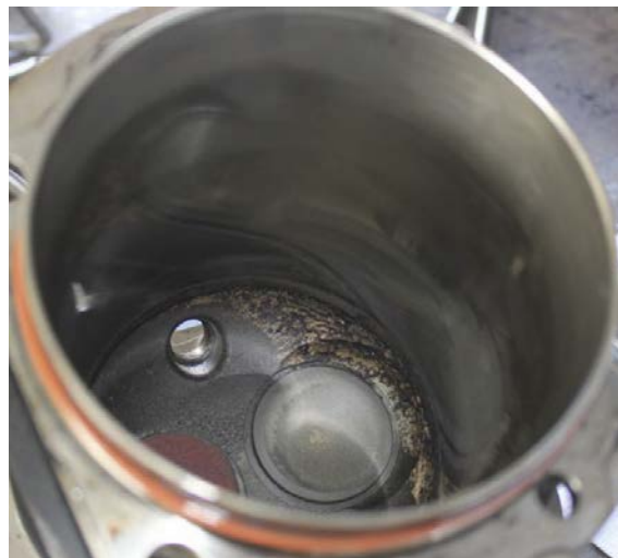
Figure 6 - view 2 of number 3 cylinder and stuck exhaust valve
