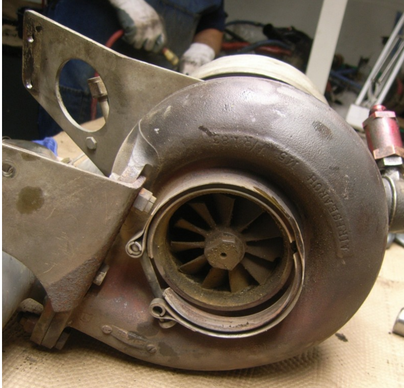
Figure 13 - Turbocharger (turbine outlet)
