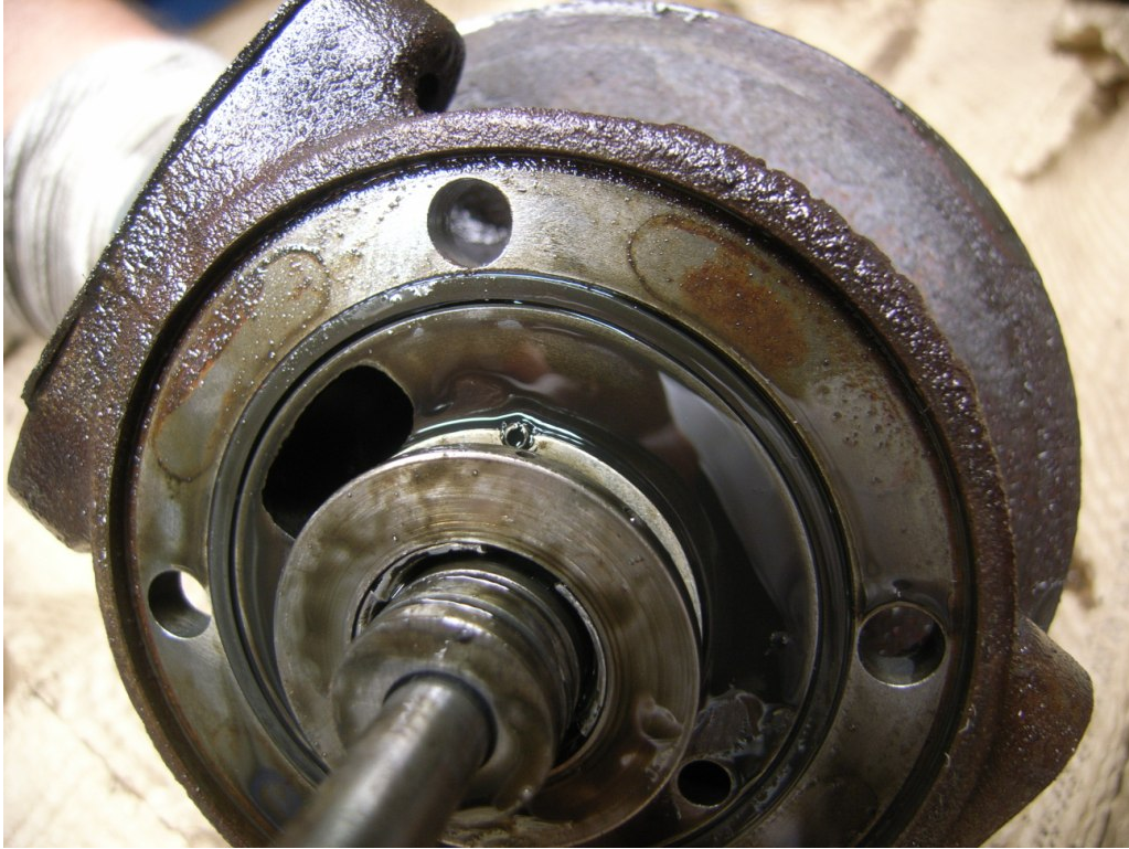
Figure 19 - Bearing Housing (compressor side)
