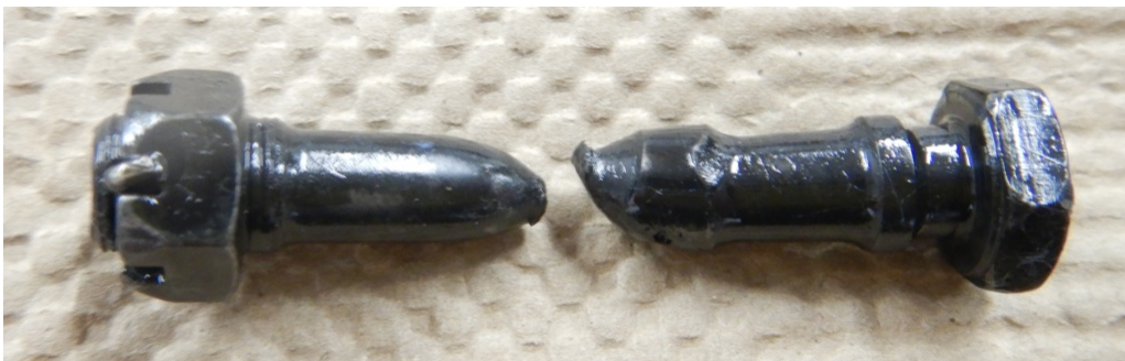
Figure 12 - Necked Connecting Rod Bolt
