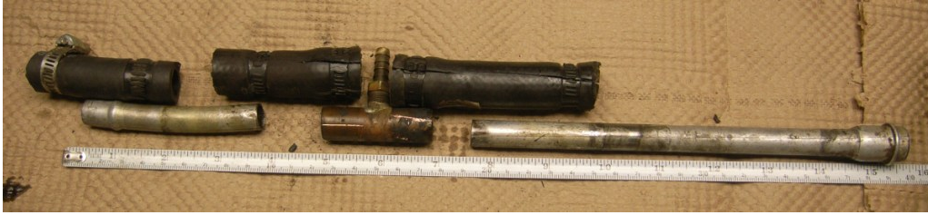
Figure 2 - Oil Rod Disassembled
