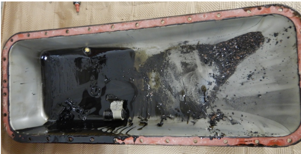
Figure 3 - Oil Sump with Debris
