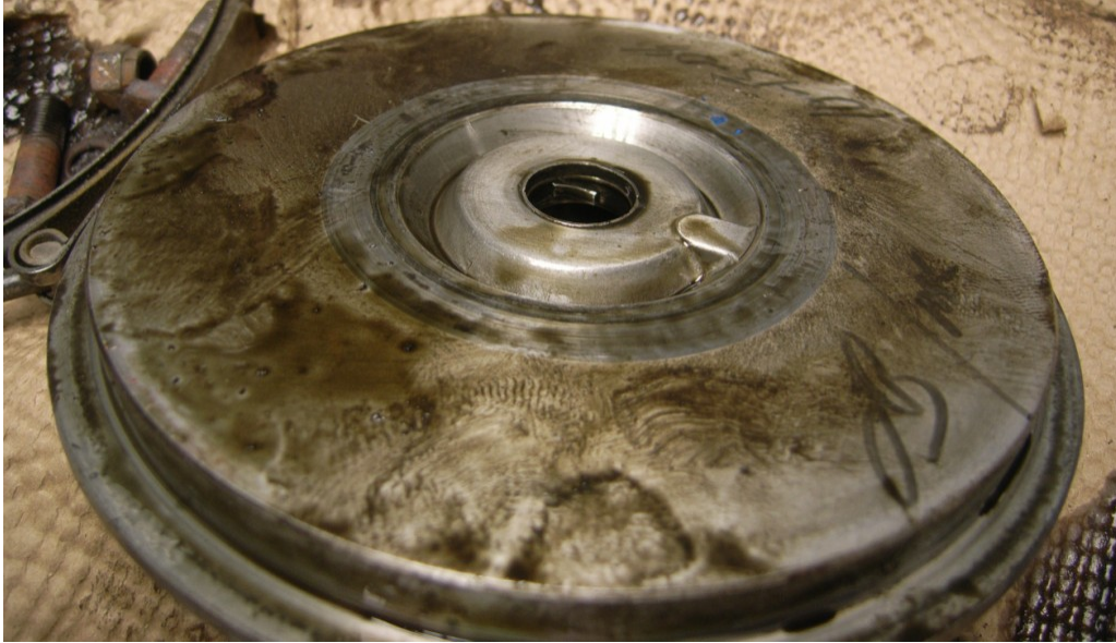
Figure 21 - Compressor End Plate
