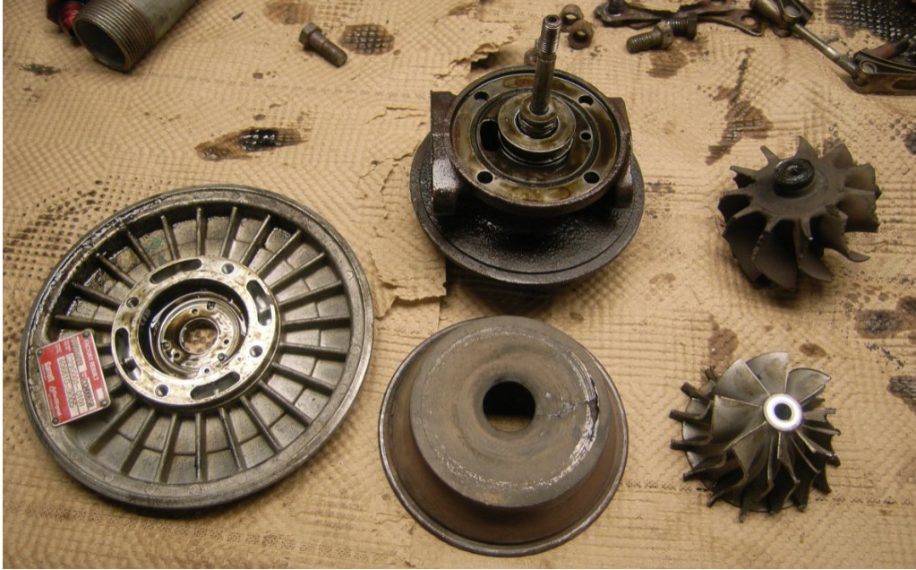
Figure 23 - Turbocharger Components for Detailed Examination
