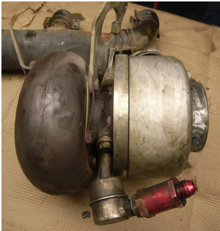
Figure 14 - Turbocharger with Oil System Components
