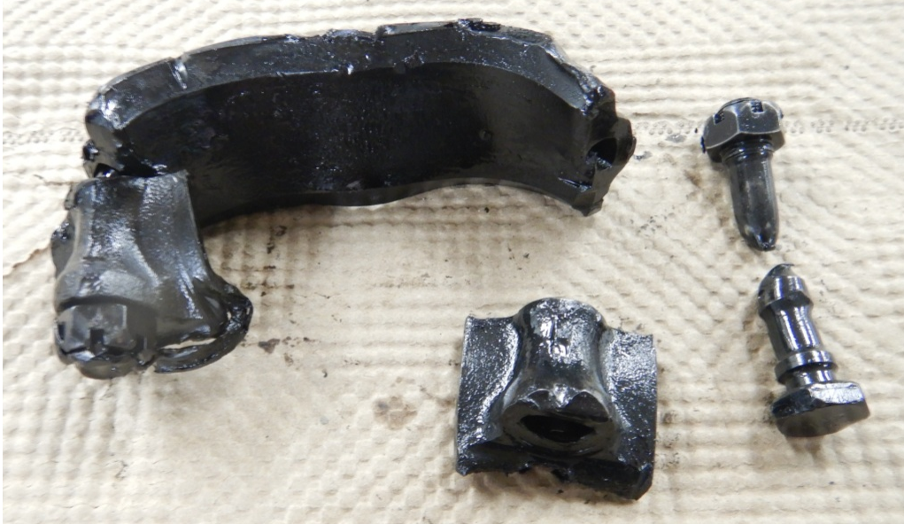
Figure 11 - No. 1 Connecting Rod End Cap
