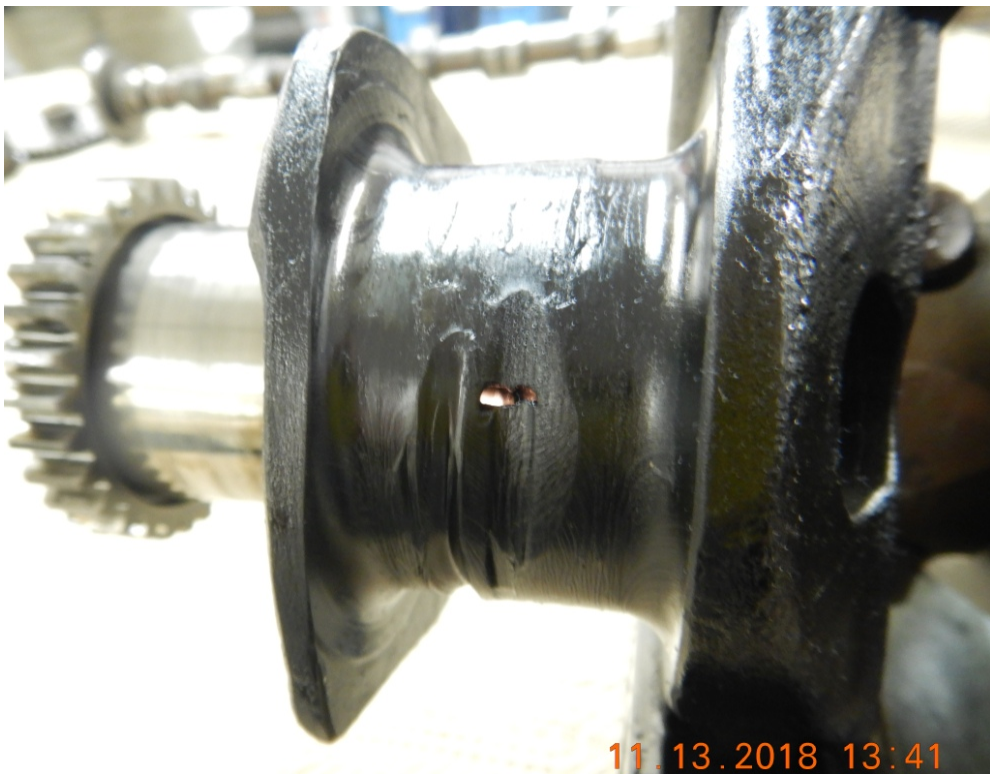
Figure 8 - No. 1 Connecting Rod Journal on Crankshaft
