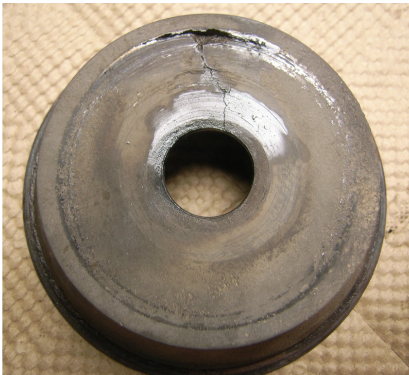
Figure 18 - Turbine End Plate (after cleaning)
