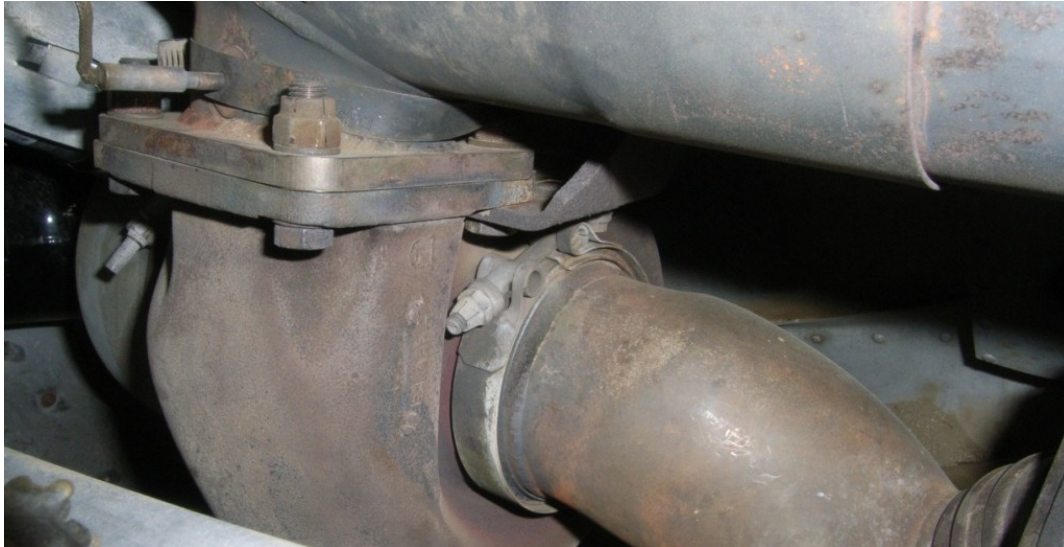
Figure 39 - Non Safety-Wired Clamp
