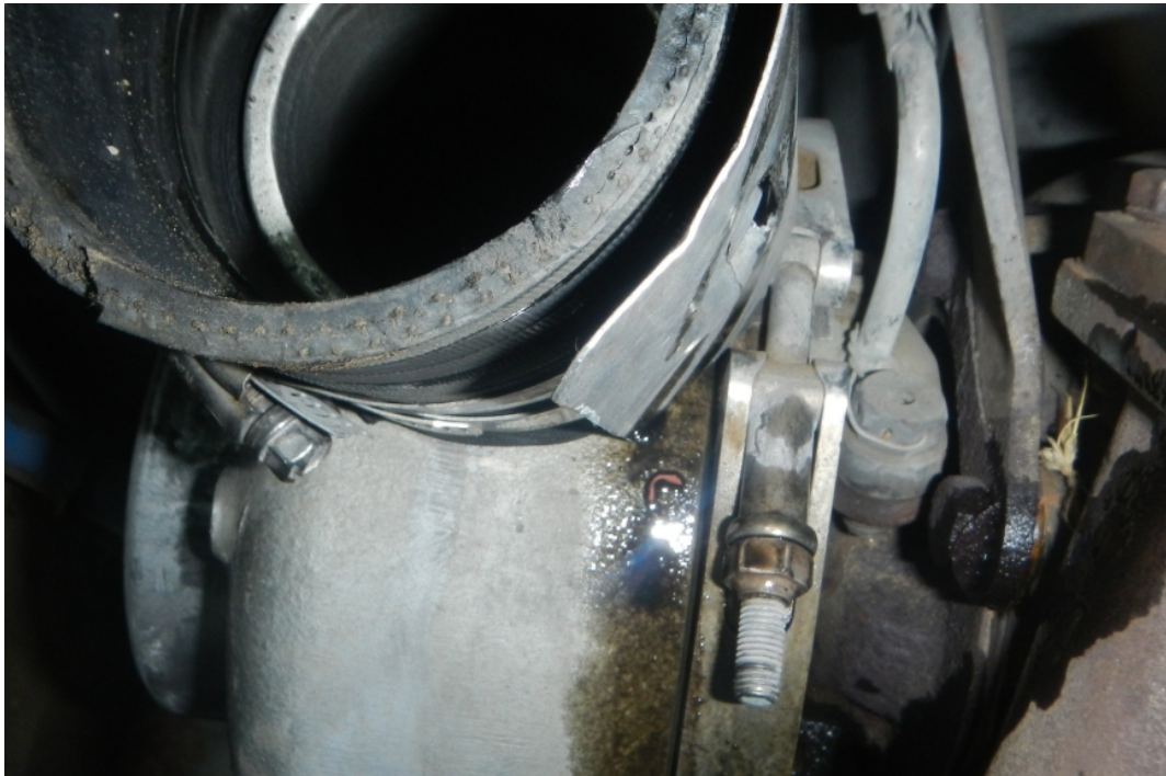
Figure 40 - Non Safety-Wired Clamp
