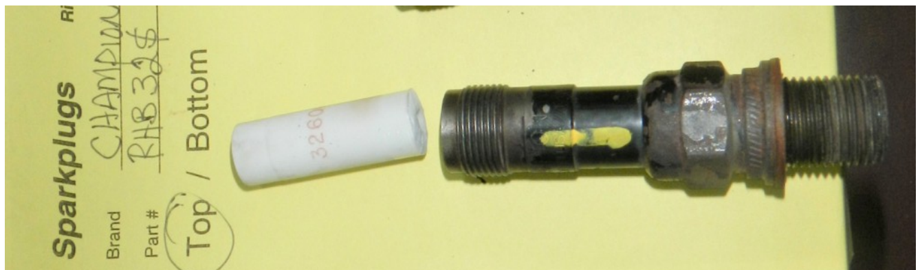
Figure 20 - Fractured Insulator, Top No. 1 Cylinder
