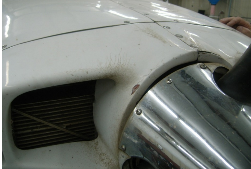
Figure 7 - Trace Oil Residue on Inlet
