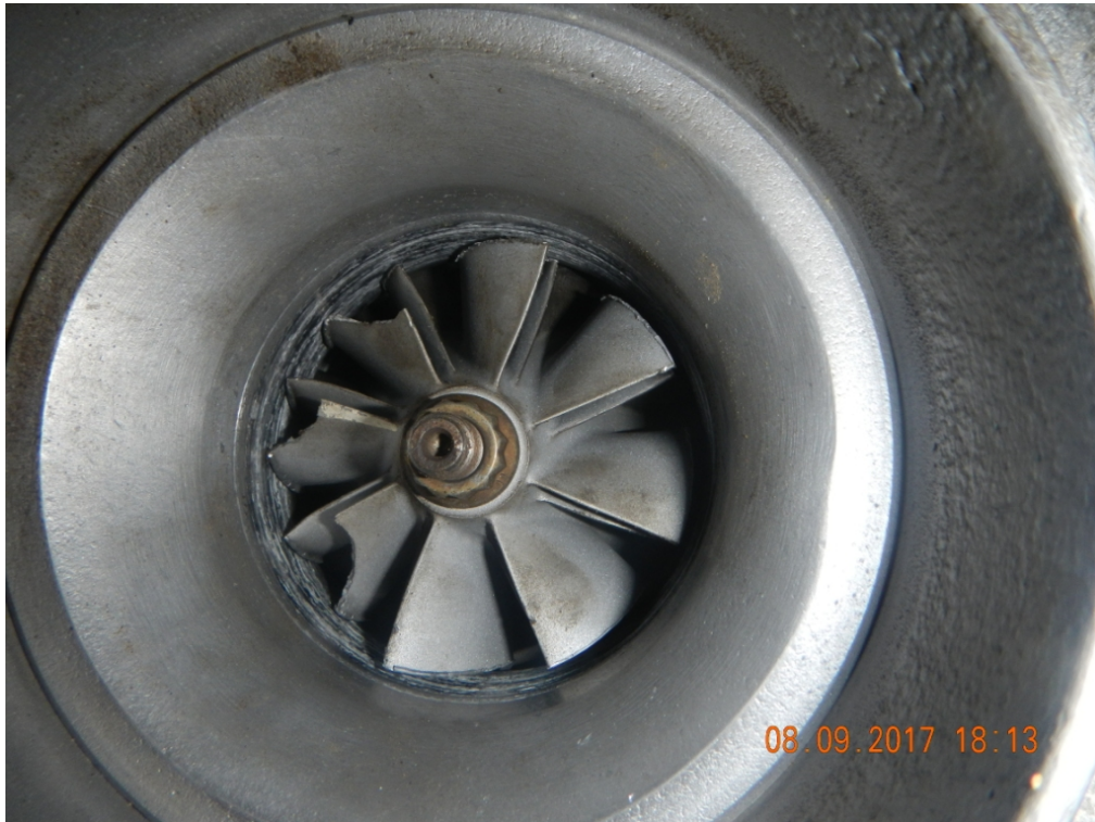
Figure 41 - Fractured Turbocharger Compressor Blades
