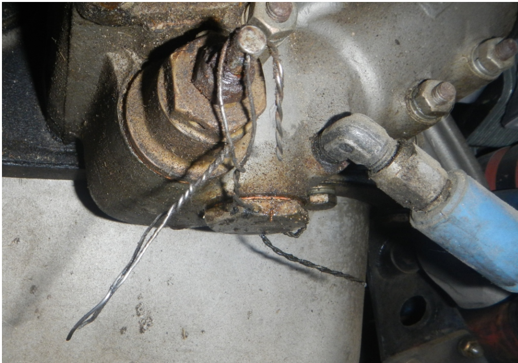
Figure 38 - As-Found Cut Safety Wire
