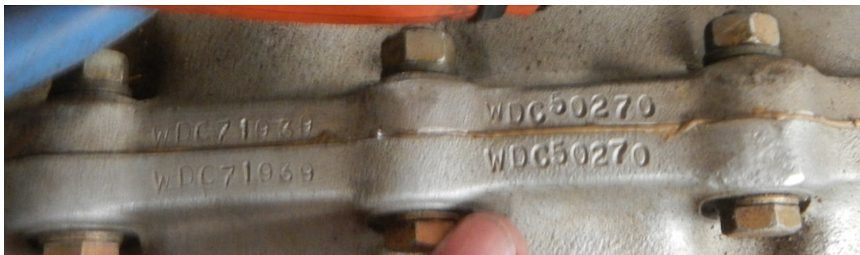
Figure 16 - Engine Case Half ID Stampings
