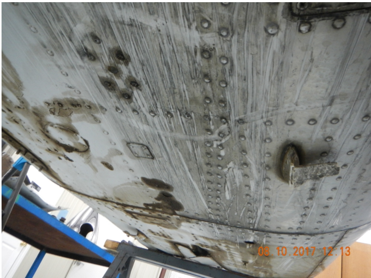
Figure 1 - Oil on Airplane Underside (view forward)
