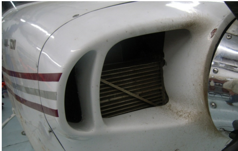
Figure 8 - Trace Oil Residue on Inlet
