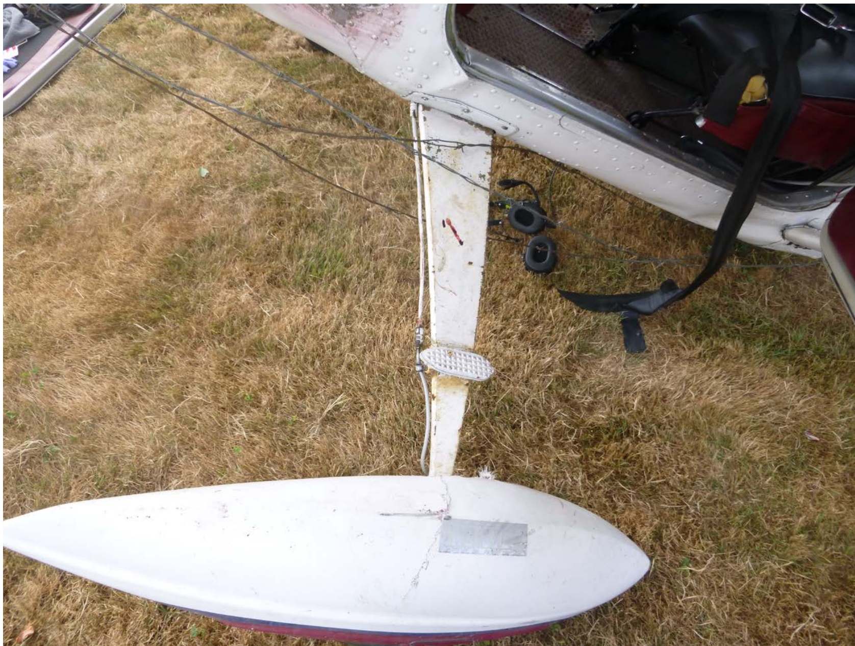
Photo 4 - Barbed wire wrapped around the landing gear strut
