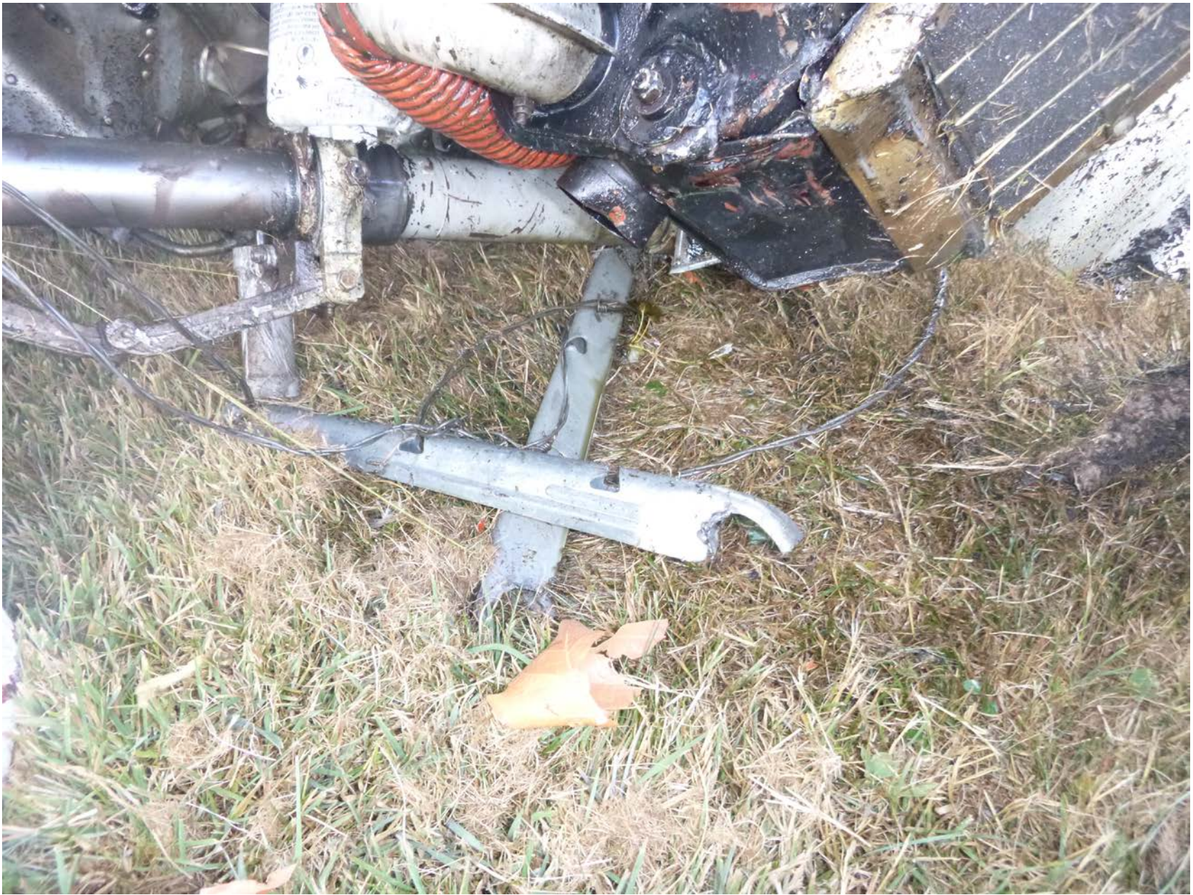
Photo 3 – Barbed wire and fence post wrapped around the engine
