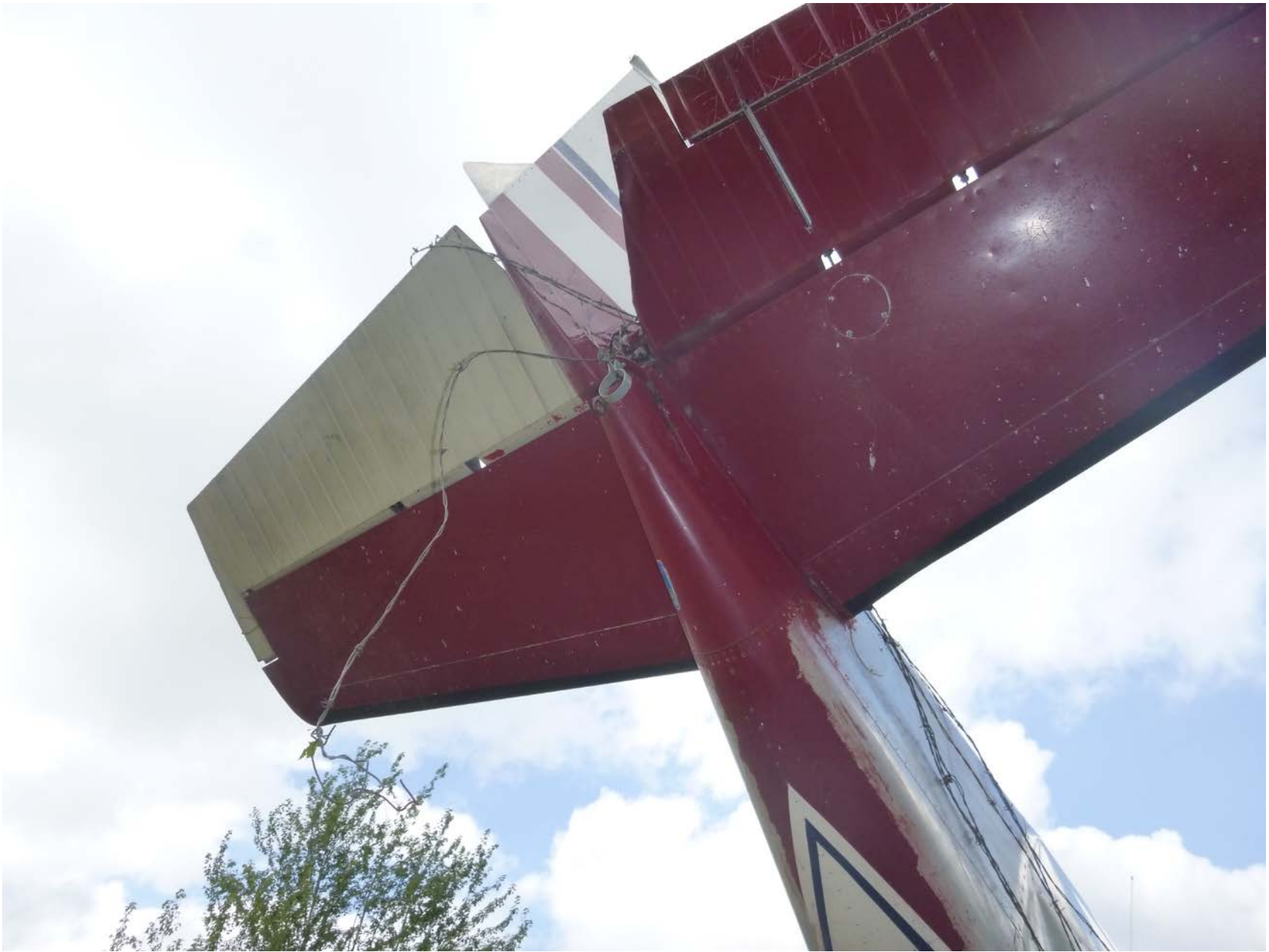
Photo 5 - Barbed wire wrapped around the elevator
