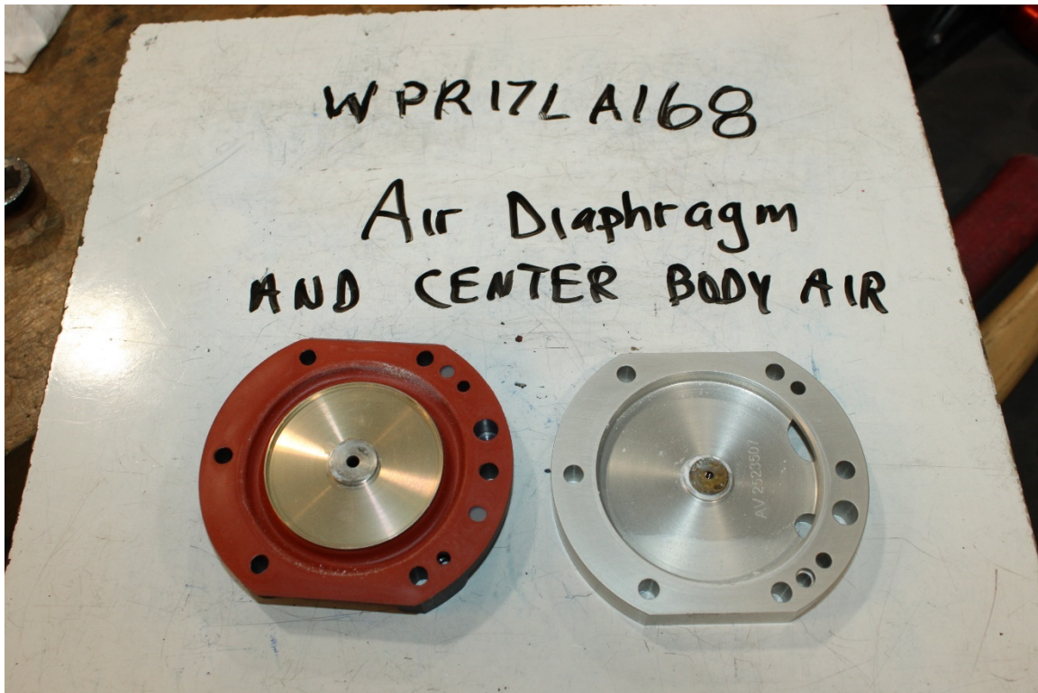
Figure 6: Air Diaphragm and Air Side of the Center Body Showing Contamination and Line.
