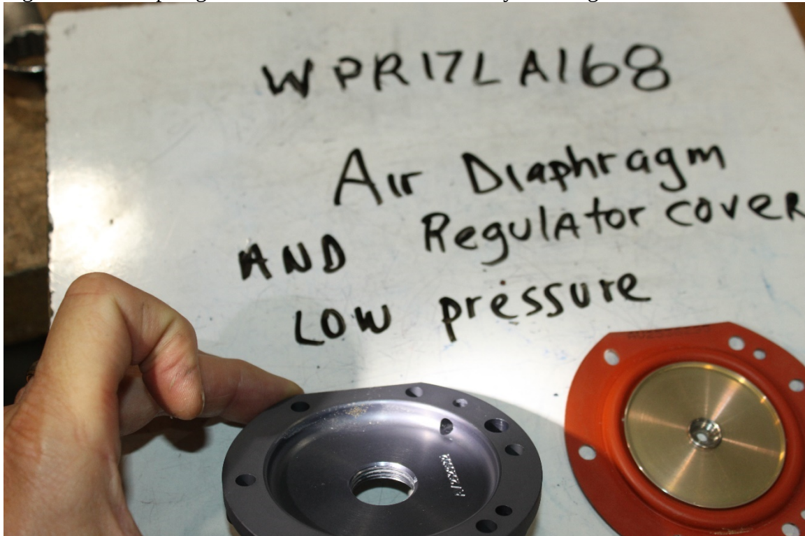
Figure 7: View Showing the Slight Contamination in the Regulator Cover and Air
