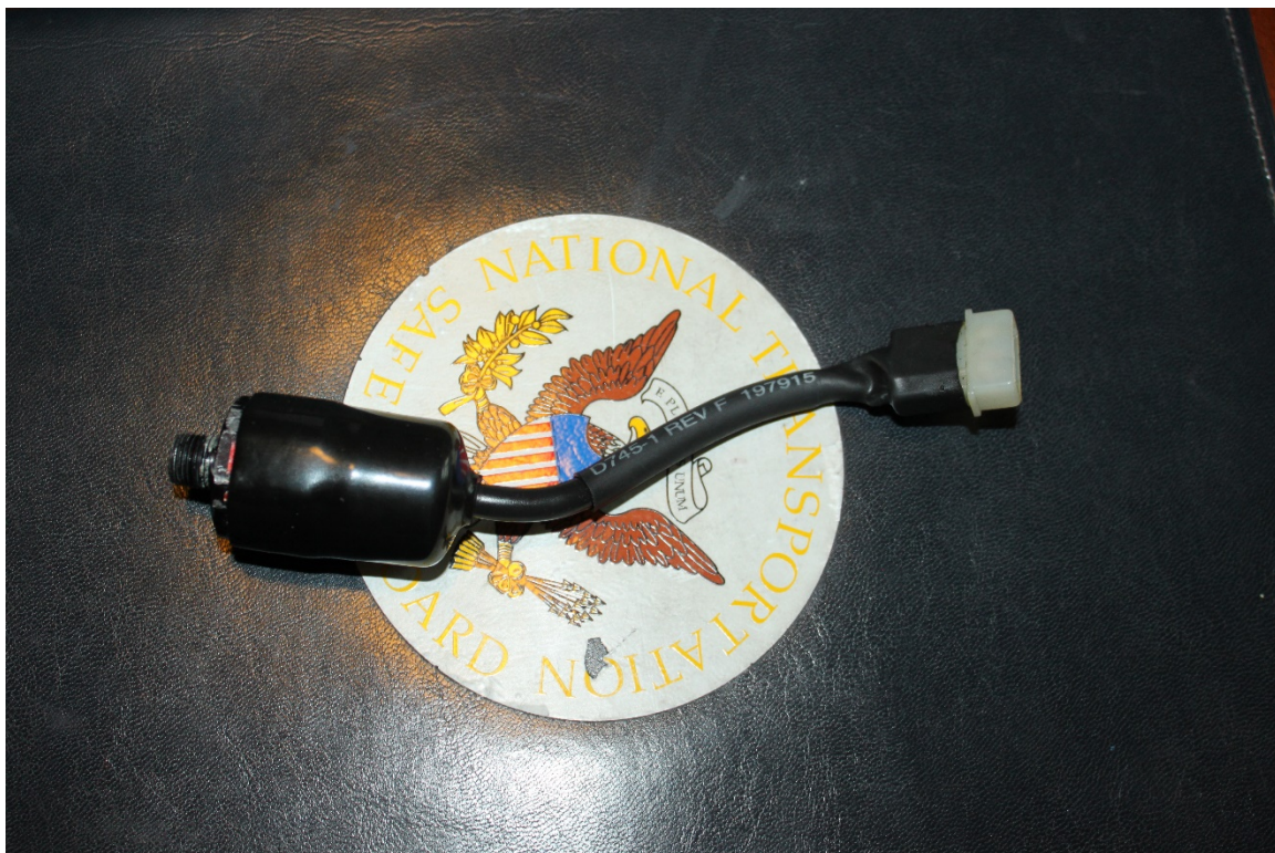
Figure 11: View of the Wasco Pressure Switch and attached Electrical Lead
