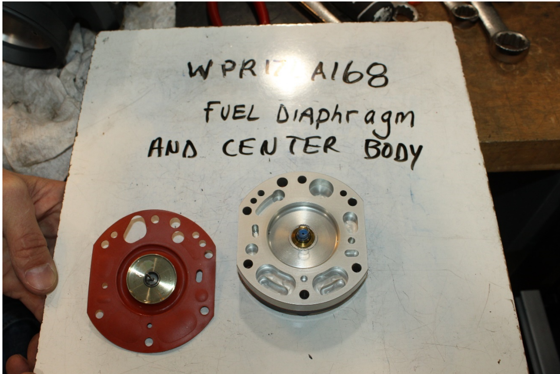
Figure 4: Fuel of the Fuel Diaphragm and Fuel Side of the Center Body
