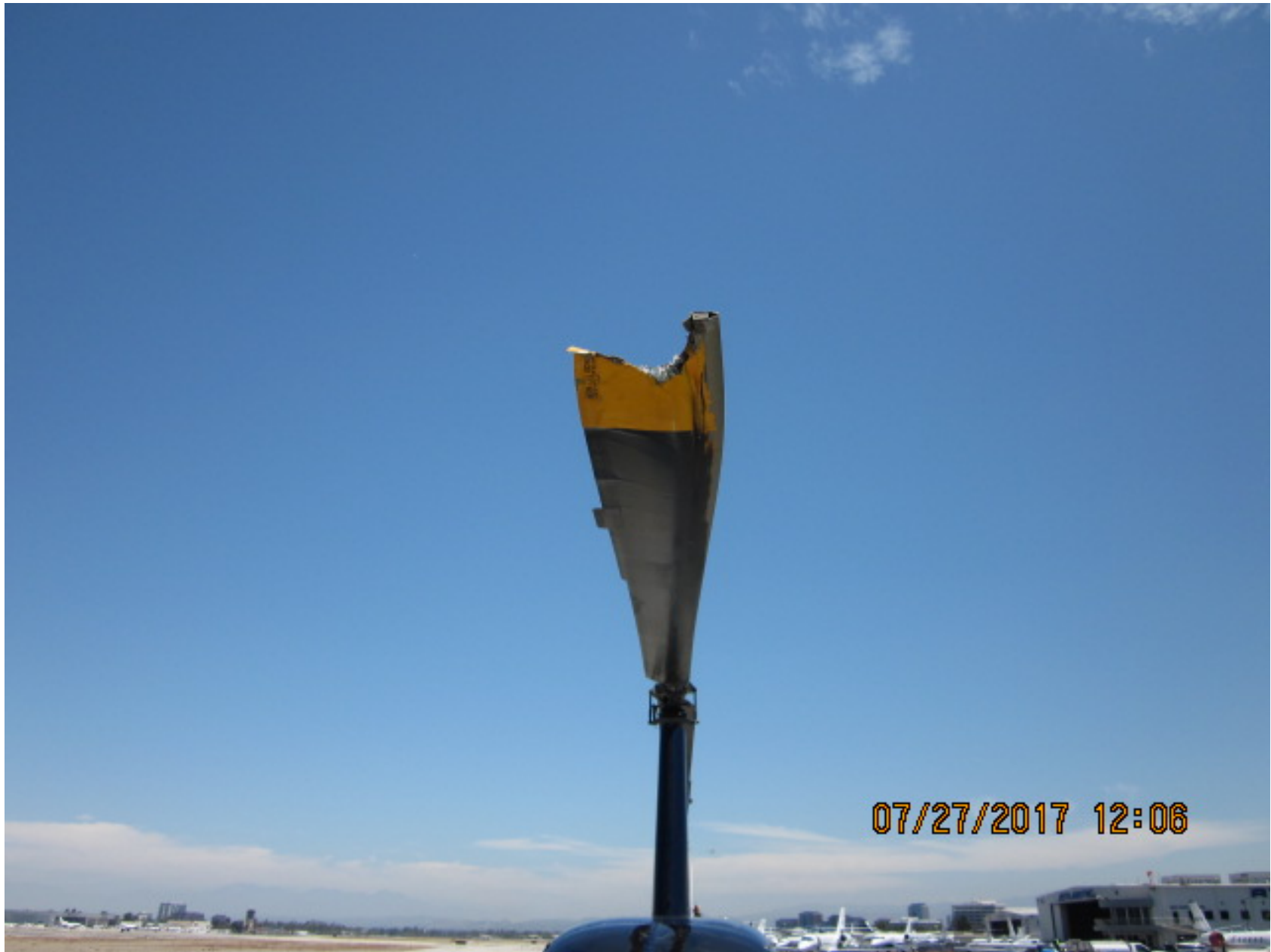
Photo 2 – Damaged main rotor blade
