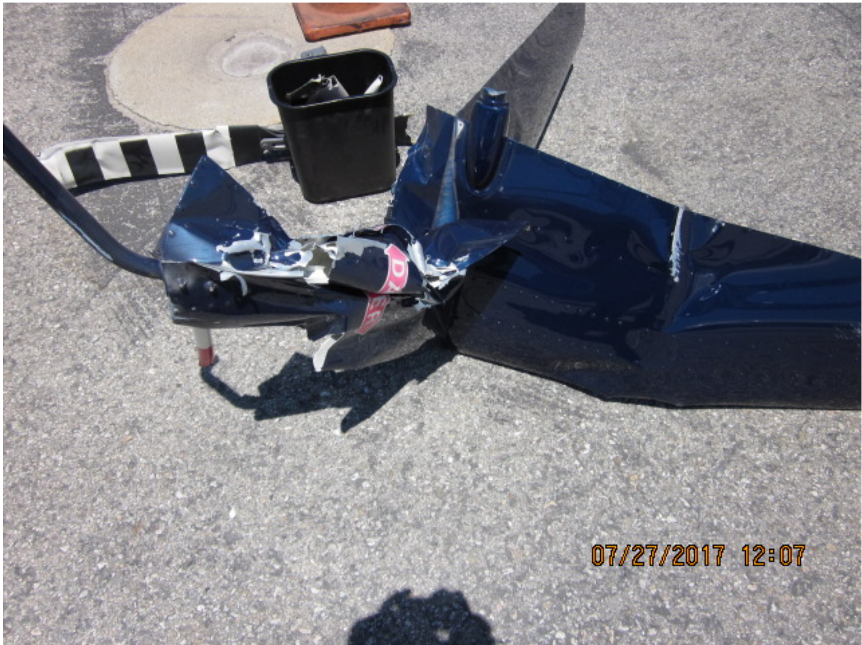
Photo 3 – Damaged tail rotor/tailboom
