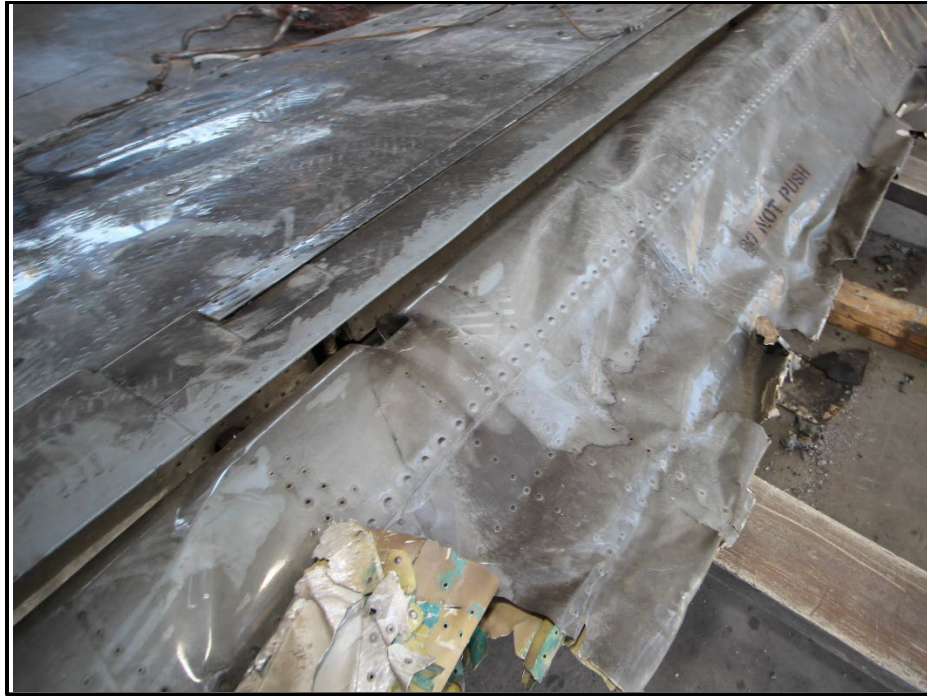
Figure 2: Right wing prepared for examination as viewed from the rear.
