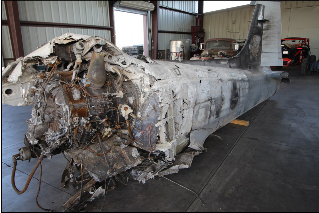
Figure 1: Airplane wreckage prepared for the examination as viewed from the left side.
