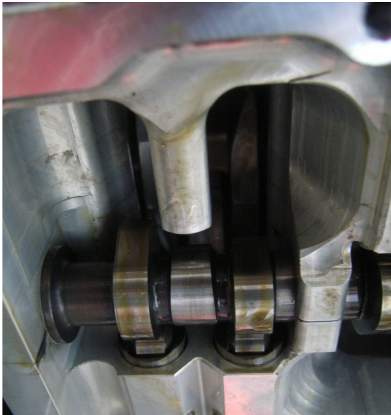
Figure 22 - EDP Pushrod Cam on Crankshaft
