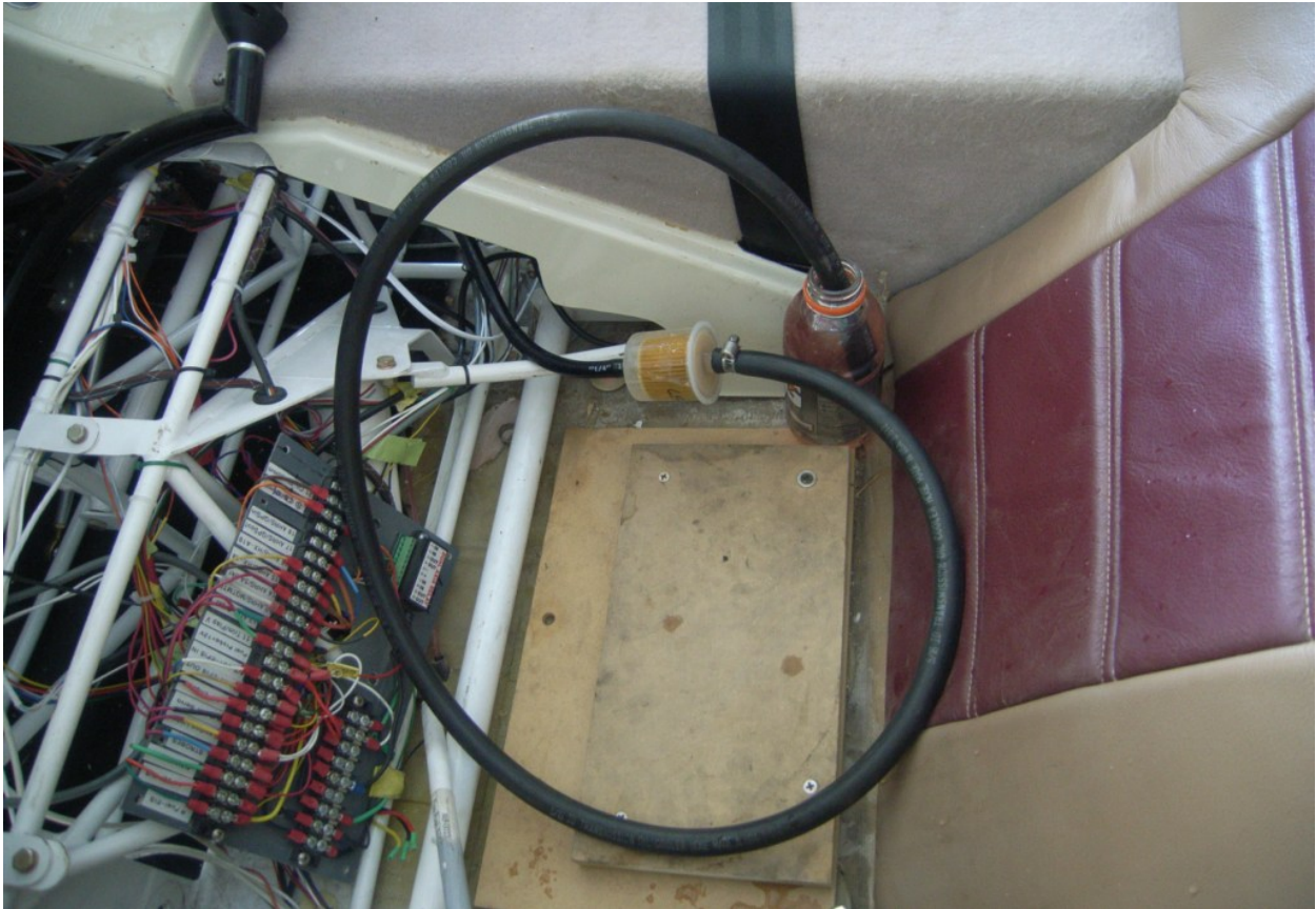
Figure 8 - Setup to Test Electric Fuel Pump
