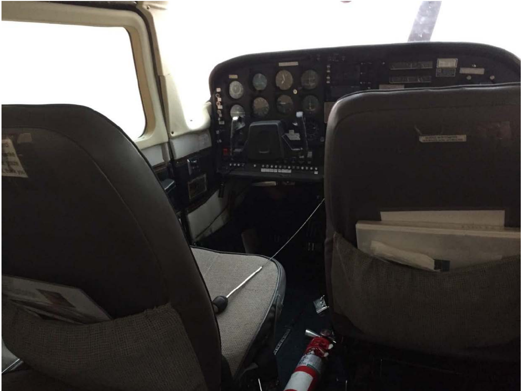
Figure 1: Throttle Control and Cable within Cockpit
