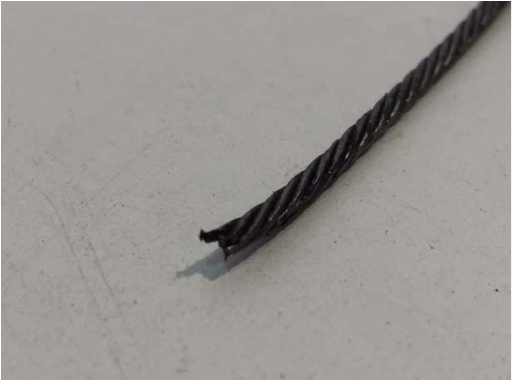
Figure 2: Throttle Cable Fracture
