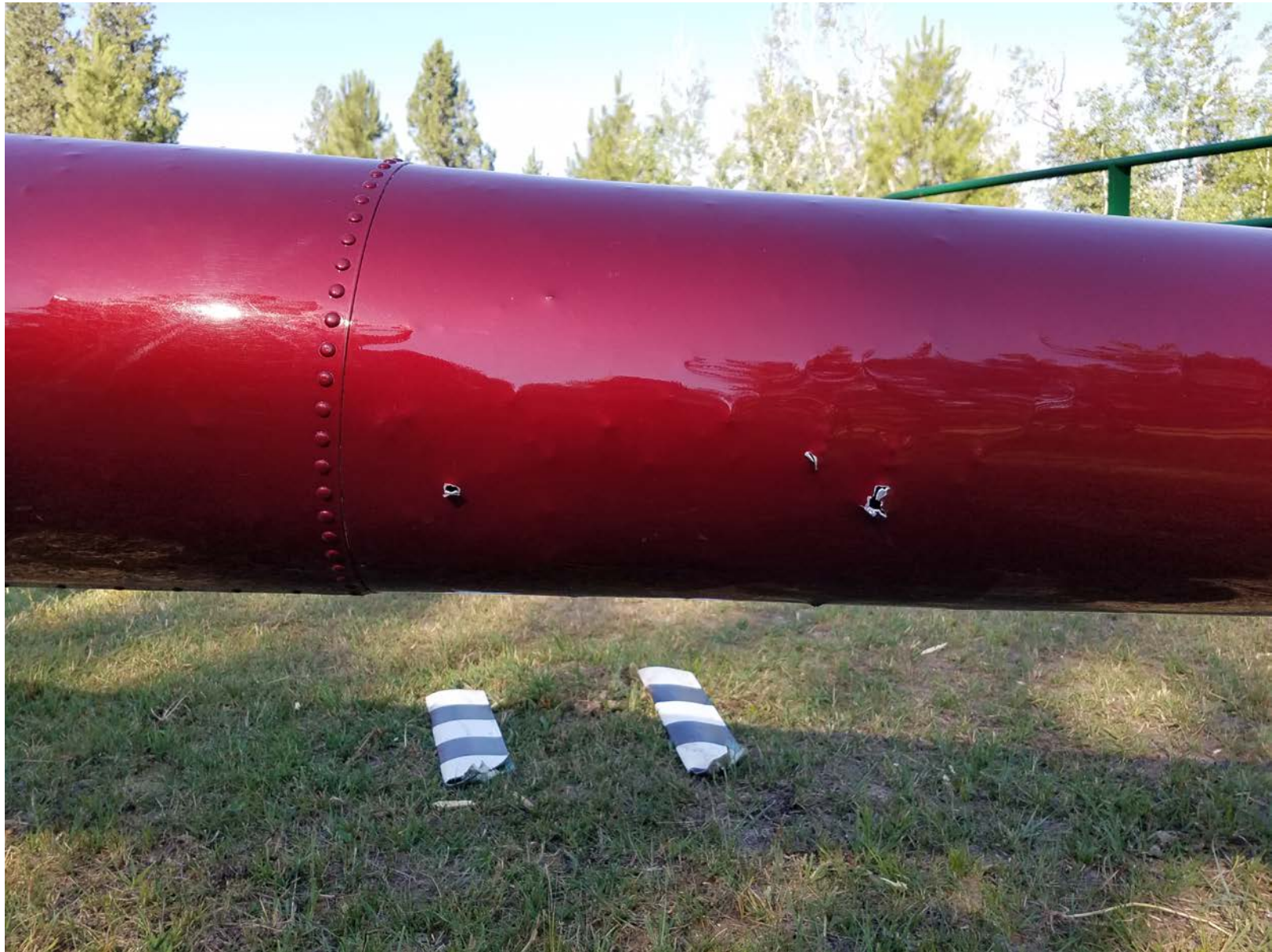
Photo 3 – Tailboom with Dents and Protrusions (Courtesy of Federal Aviation Administration)
