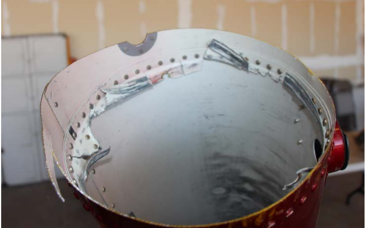
Figure 4 – Inside Diameter of Tailcone, No. 6 Bulkhead
