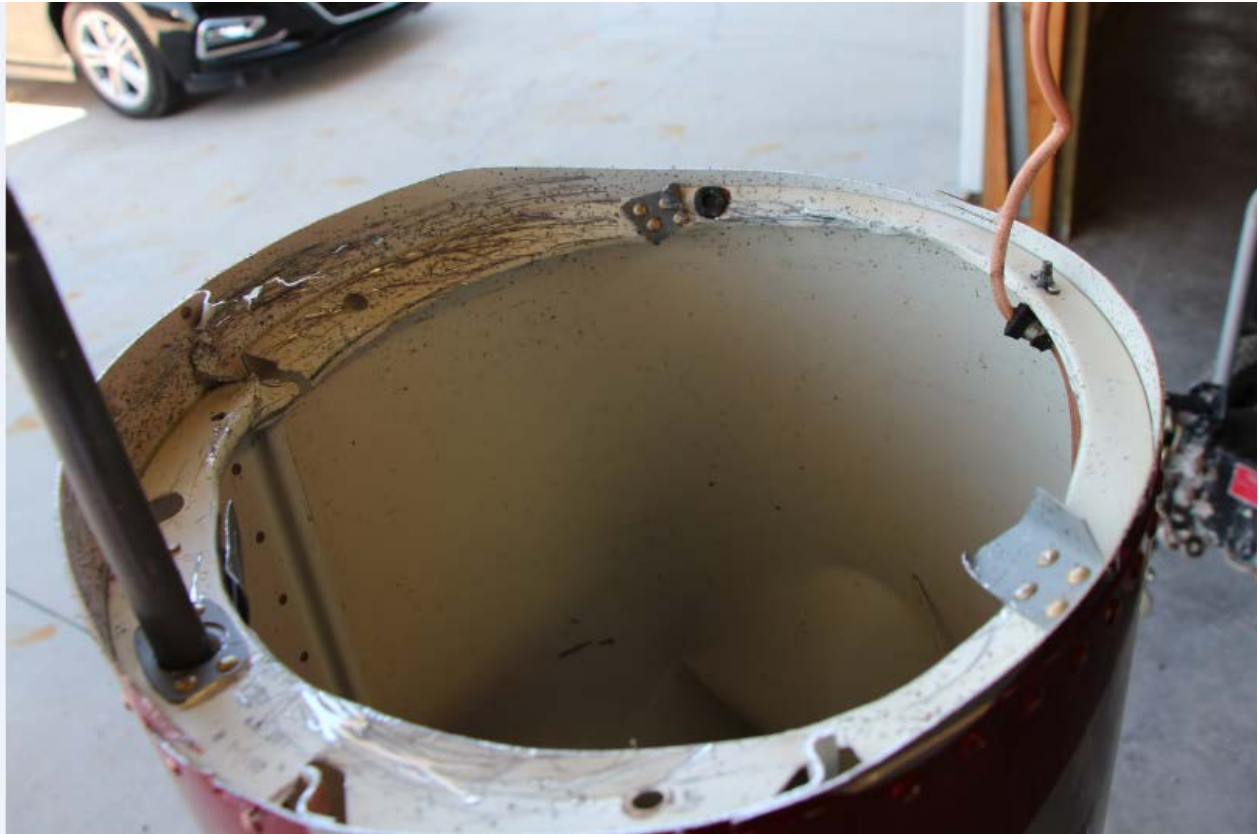
Figure 3 – Inside Diameter of Tailcone, No. 3 Bulkhead
