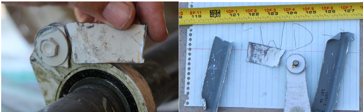
Figure 7 – Broken Hangar Bearing Support Bracket
