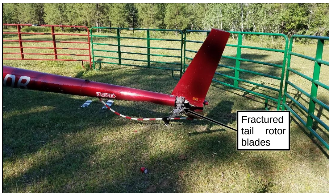
Figure 1. Views of the helicopter on scene showing the bent tail boom (upper left image), scorched vegetation near the exhaust (upper right image), and left side of the tail assembly (lower image). Images were provided courtesy of the FAA.
