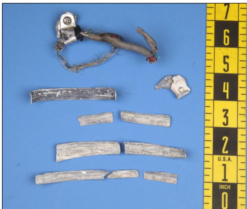
Figure 6. Overall view of the aft sides of the submitted pieces of the number 3 bulkhead, damper bearing support bracket, damper bearing, and drive shaft piece. The pieces are displayed in their approximate relative positions as installed on the helicopter, where the drive shaft is aligned directly below the upper vertical support bracket.
