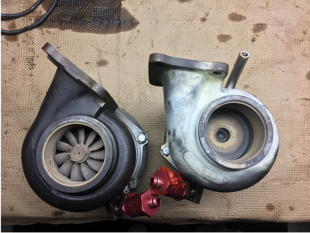
Figure 3 Turbine Side of Turbos
