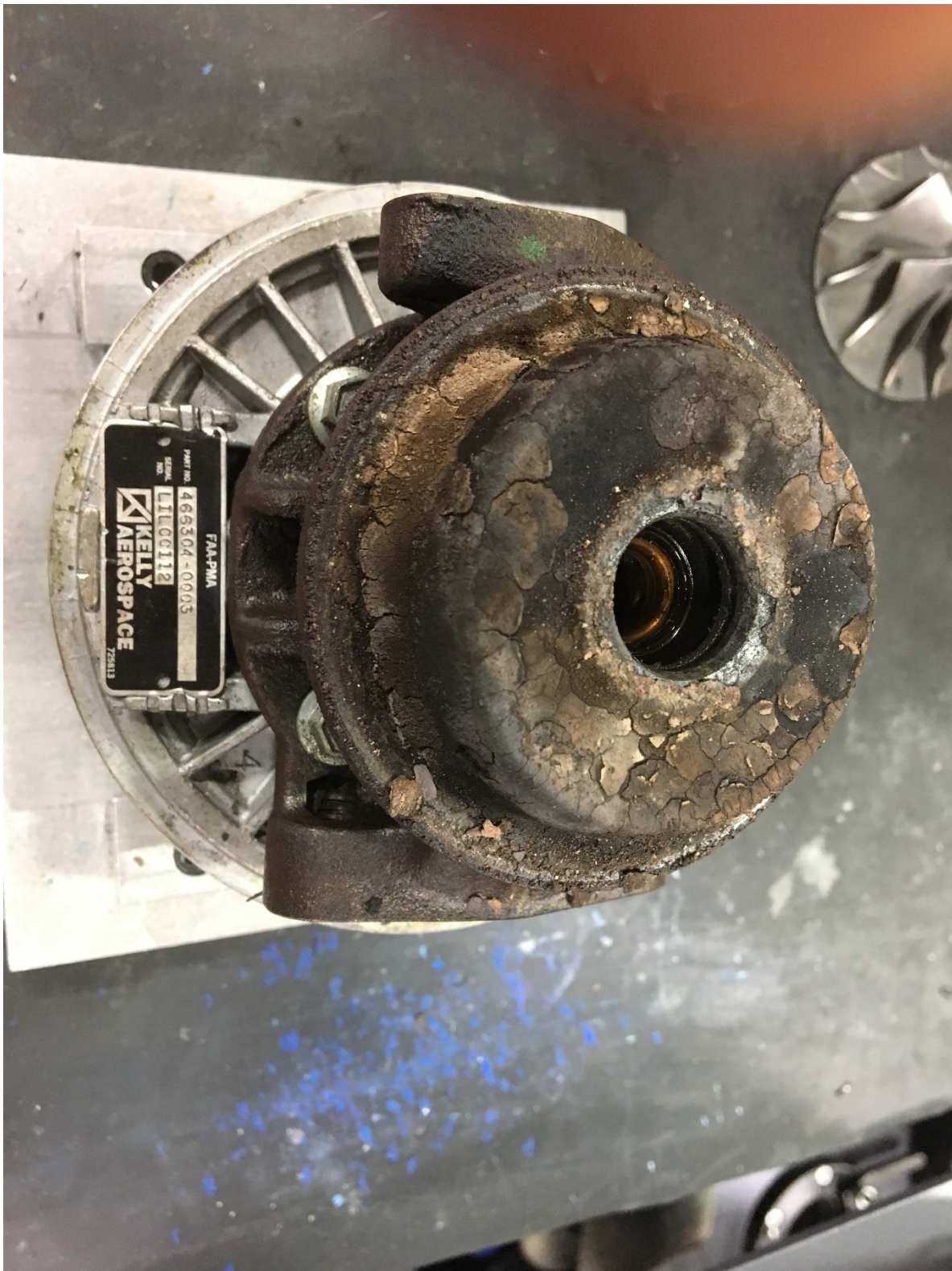
Figure 5 Left CHRA Assembly Nose Coking
