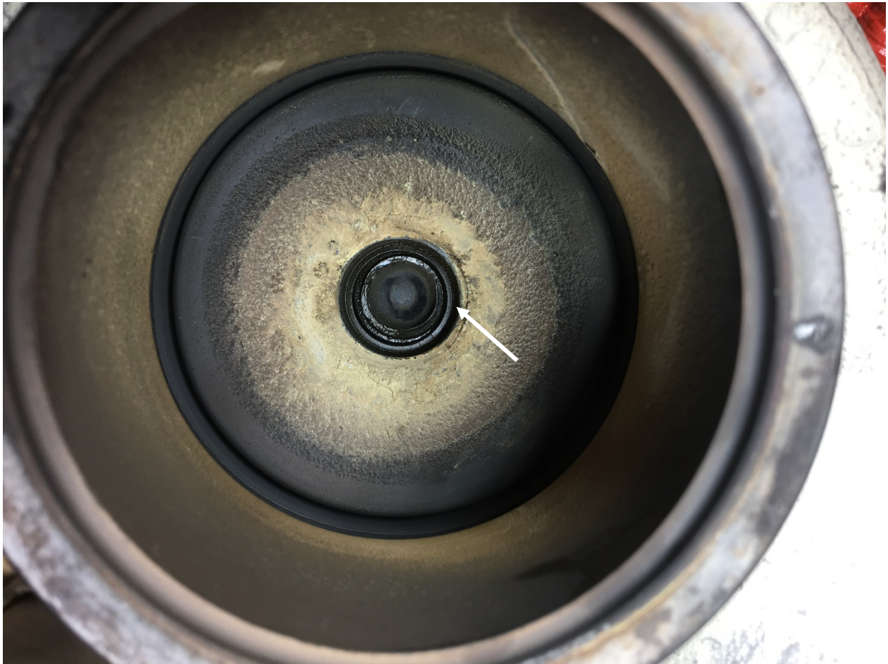
Figure 8 Right Center Housing Bore with White Arrow Pointing at Fractured Piston Ring Groove
