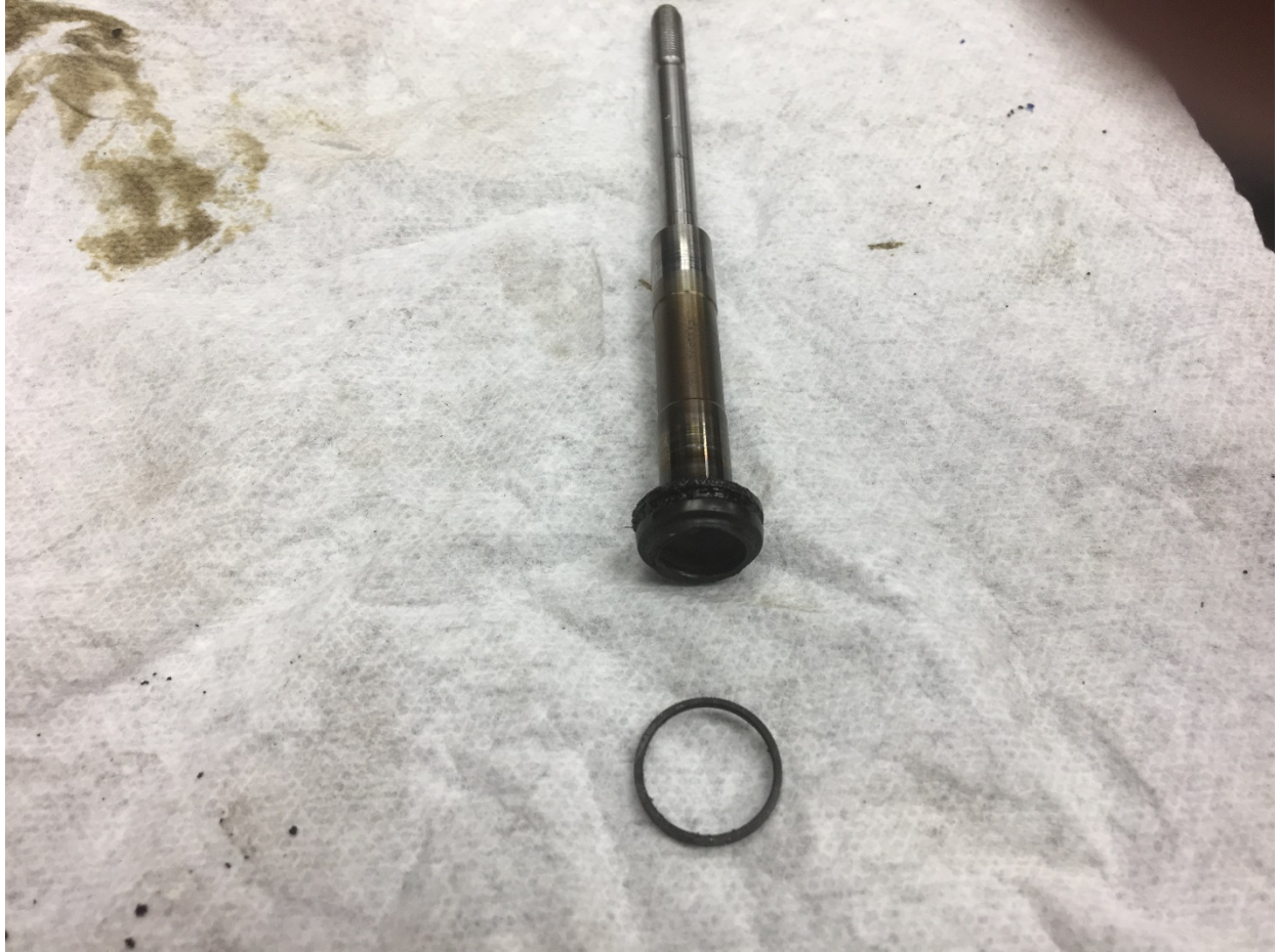
Figure 9 Turbine Shaft Fractured End
