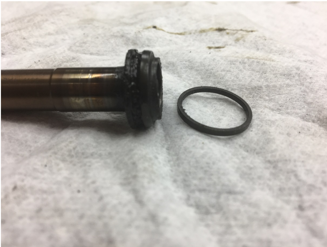
Figure 11 Close-up of Fractured End
