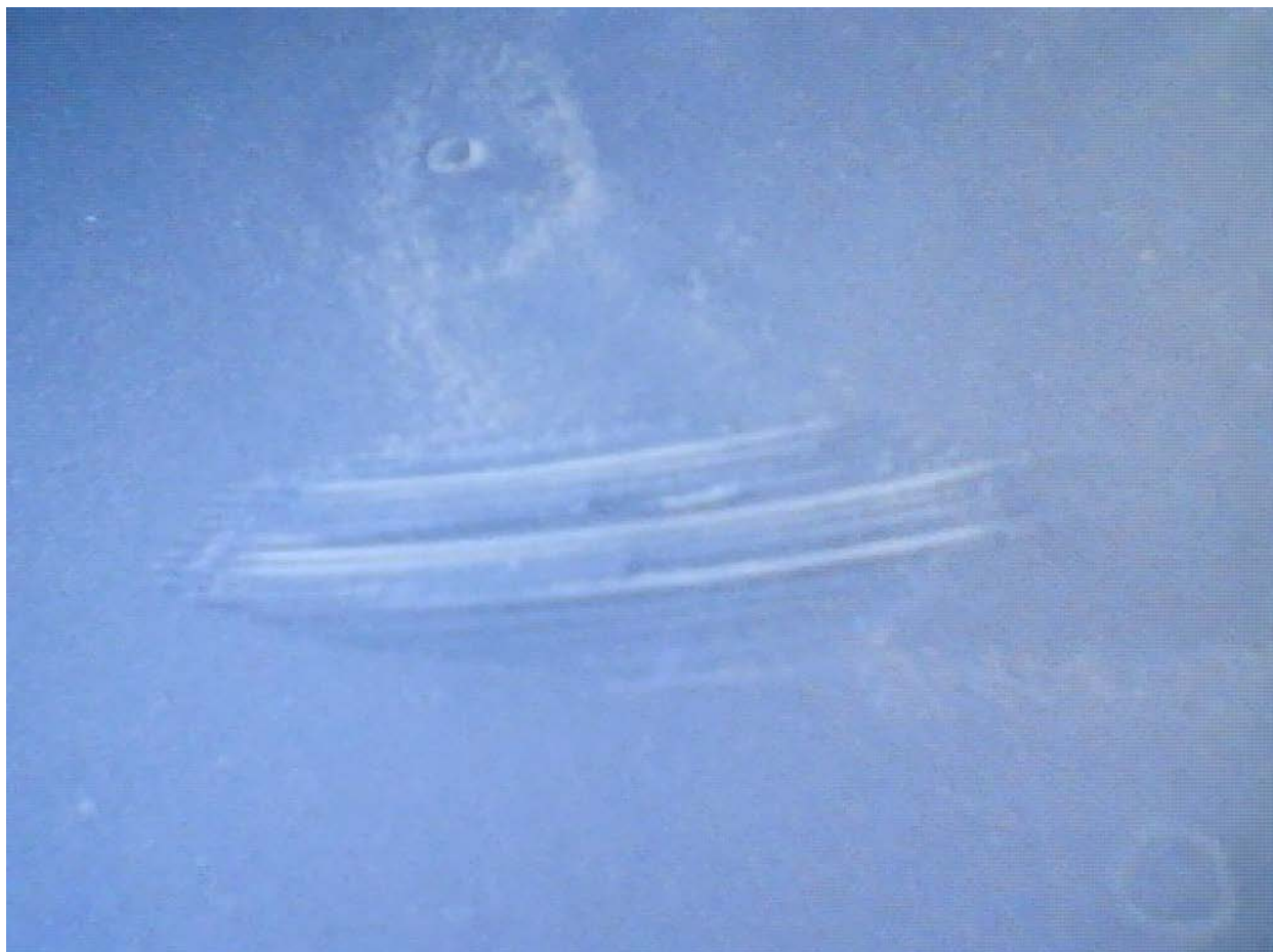
Figure 18 Scrape Mark 6 Inside Right Exhaust
