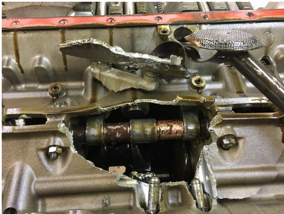
Figure 9 Closeup of Displaced Oil Sump Screen
