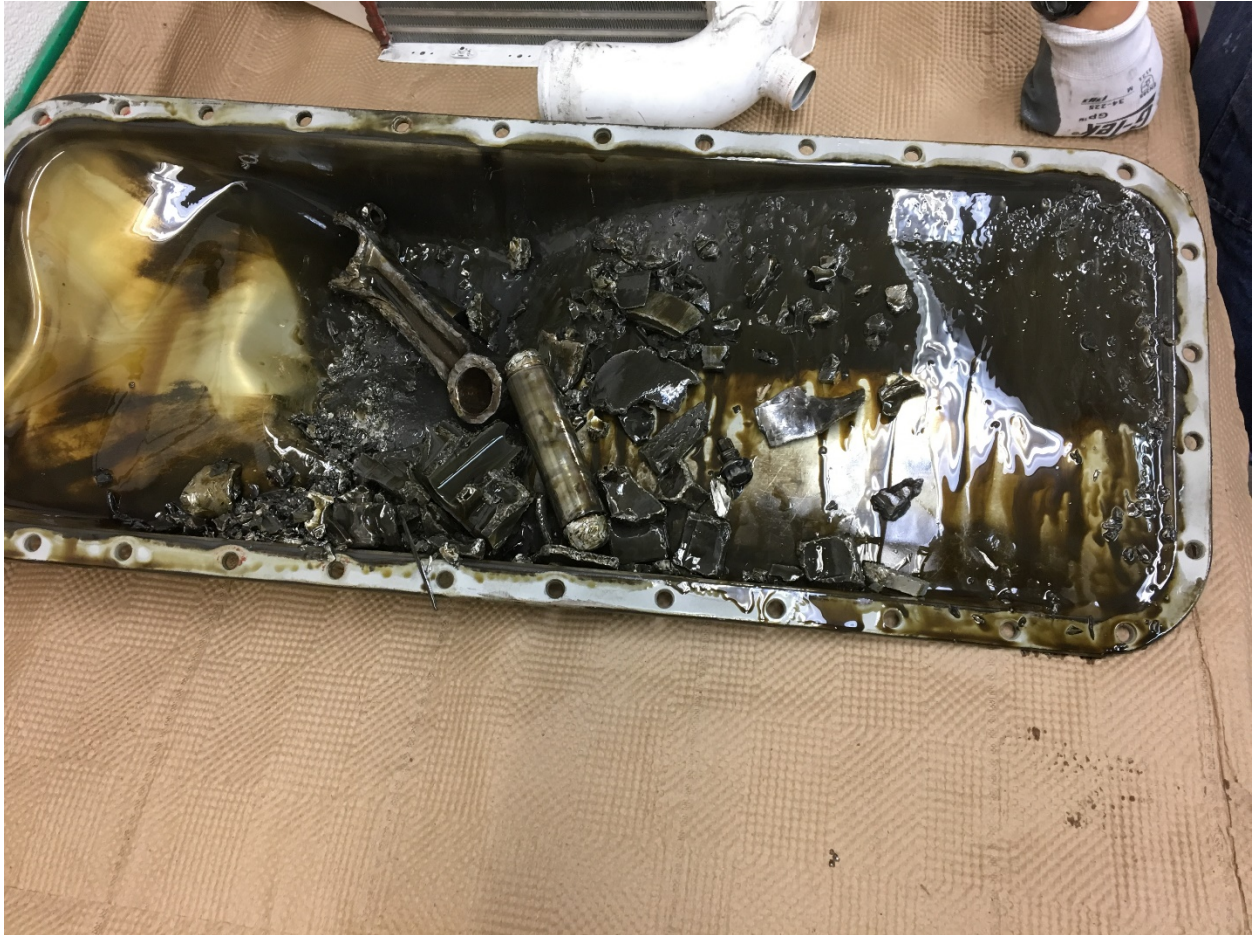
Figure 7 Oil Pan with Debris
