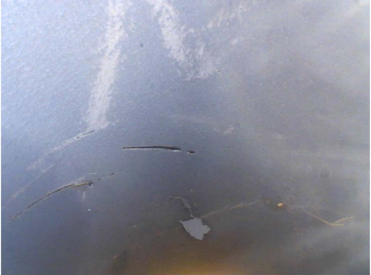
Figure 17 Scrape Mark 5 Inside Exhaust
