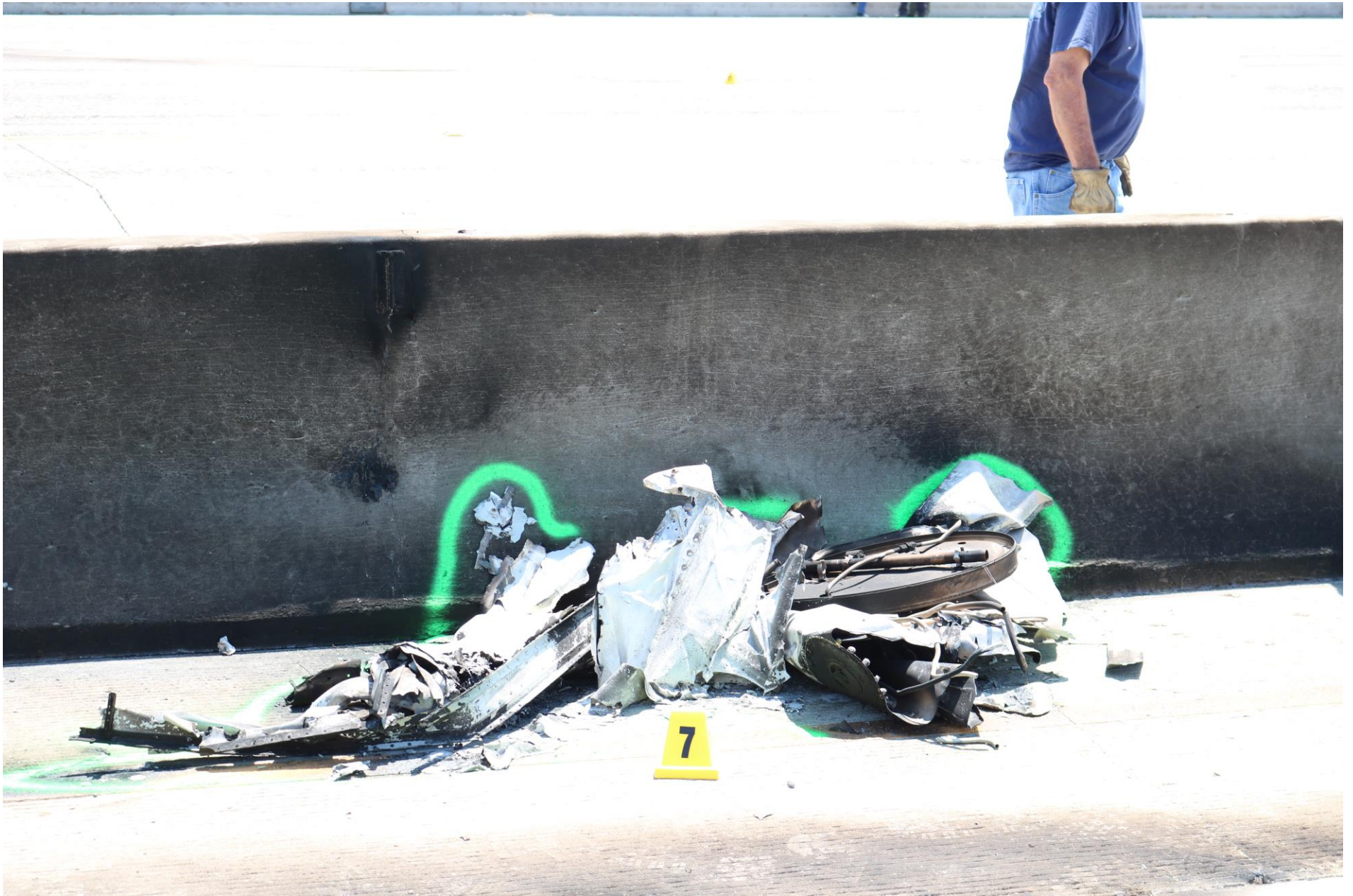
Photo 1 – Accident site, left wing tip tank, northbound freeway.
