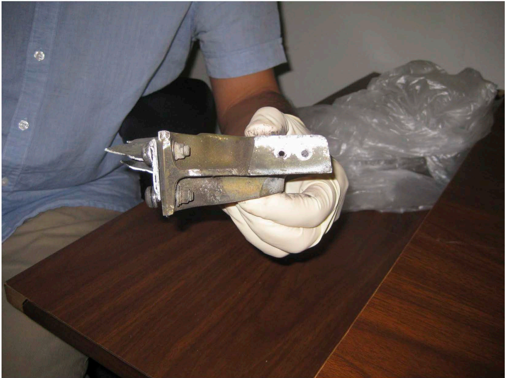
Photo 15 - Portion of the right main landing gear trunnion. Courtesy of the Federal Aviation Administration.
