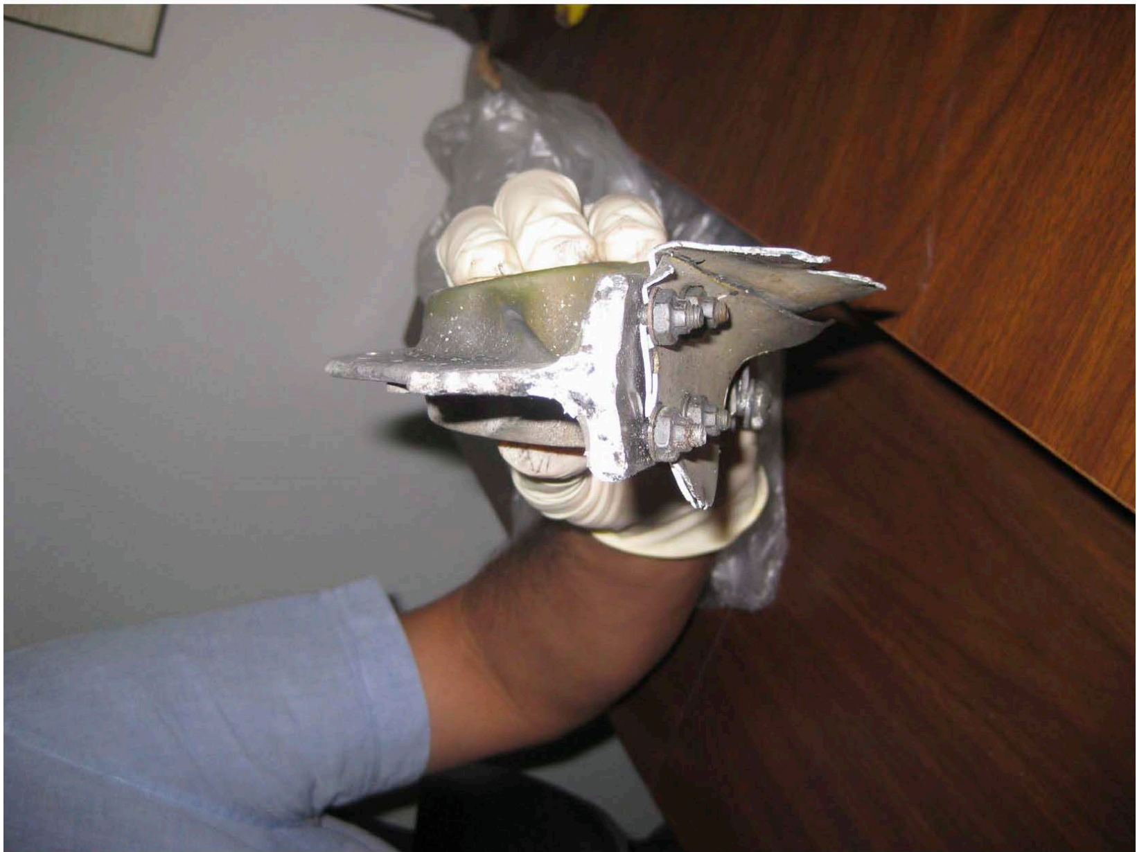
Photo 14 - Portion of the right main landing gear trunnion. Courtesy of the Federal Aviation Administration.
