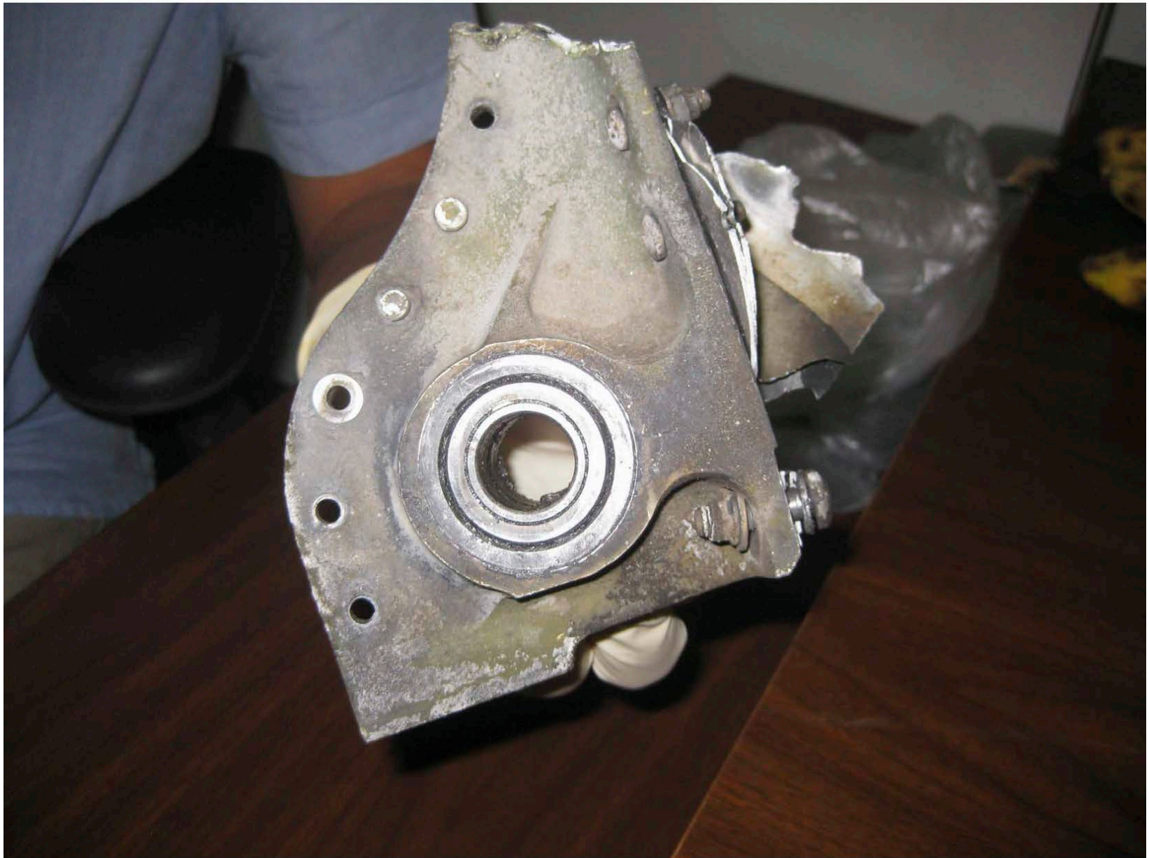
Photo 12 - Portion of the right main landing gear trunnion. Courtesy of the Federal Aviation Administration.
