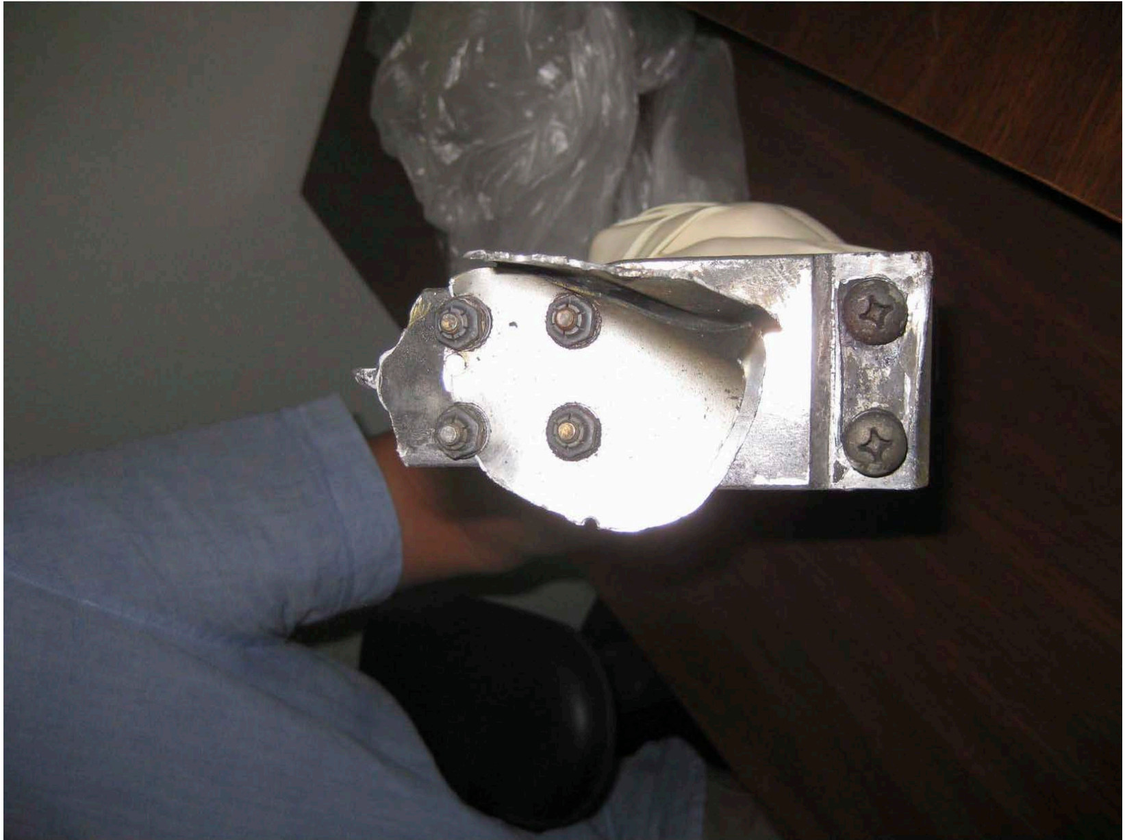
Photo 13 - Portion of the right main landing gear trunnion. Courtesy of the Federal Aviation Administration.
