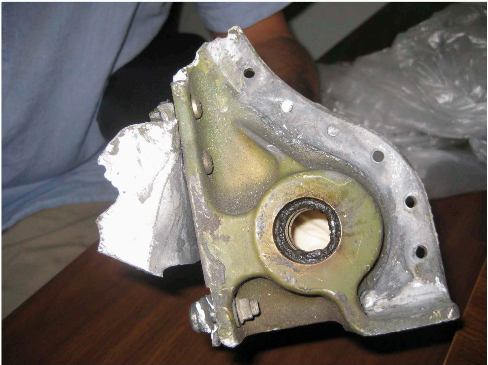
Photo 11 – Portion of the right main landing gear trunnion. Courtesy of the Federal Aviation Administration.
