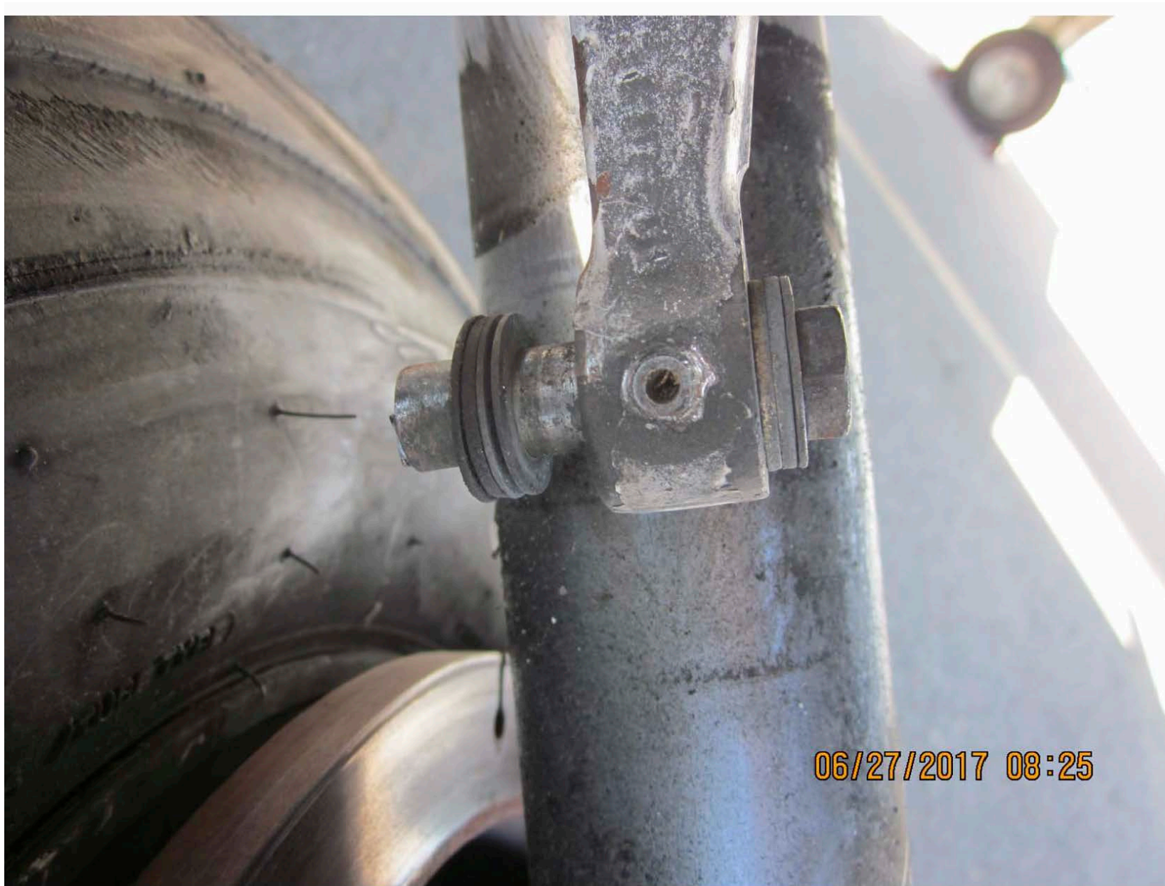
Photo 16 – Remaining right main landing gear torque link bolt. Courtesy of the Federal Aviation Administration.
