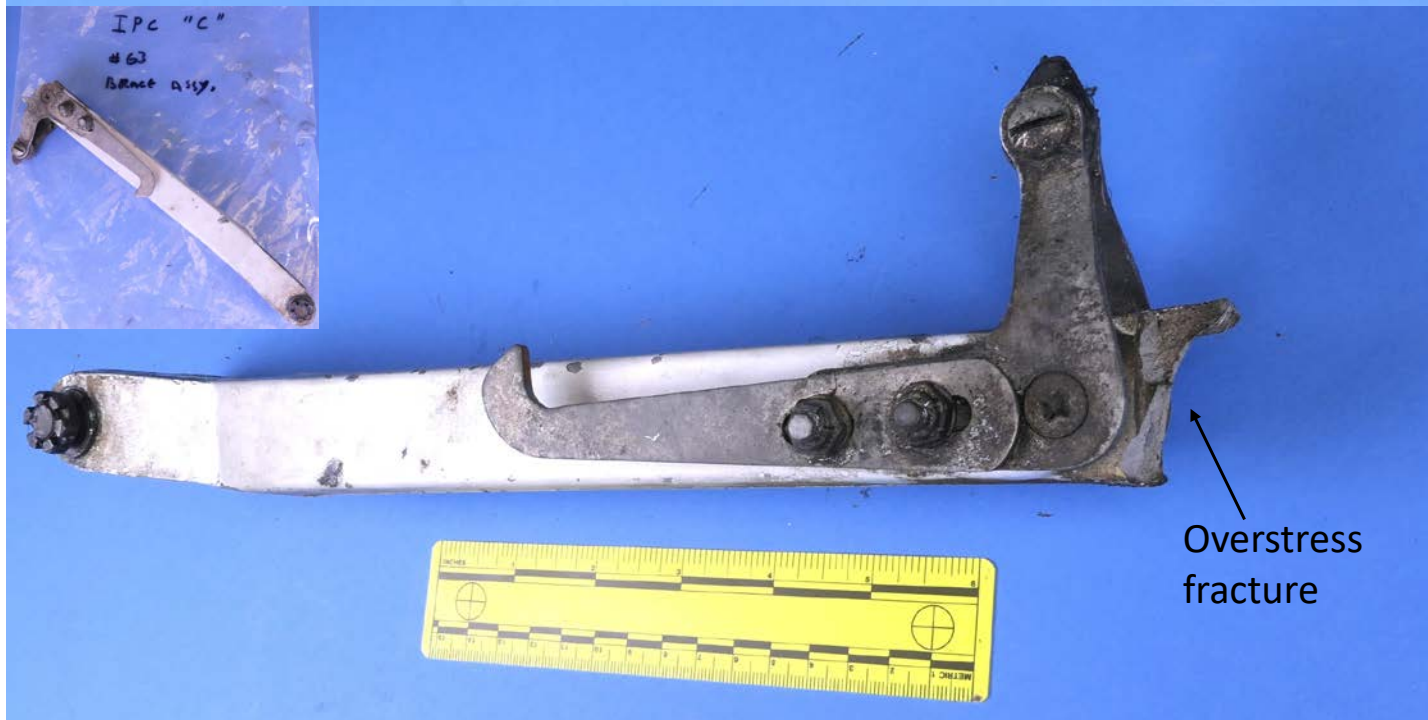
Portion of brace assembly with fracture
