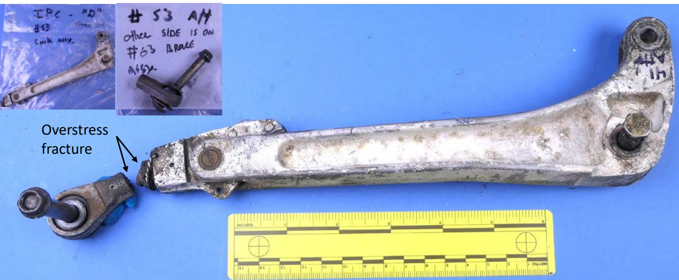
Portion of link assembly with fractured rod end
