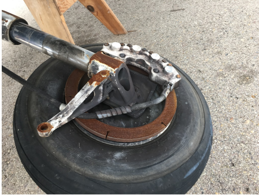
Figure 5: Right main landing gear wheel, brake, and lower link assembly.
