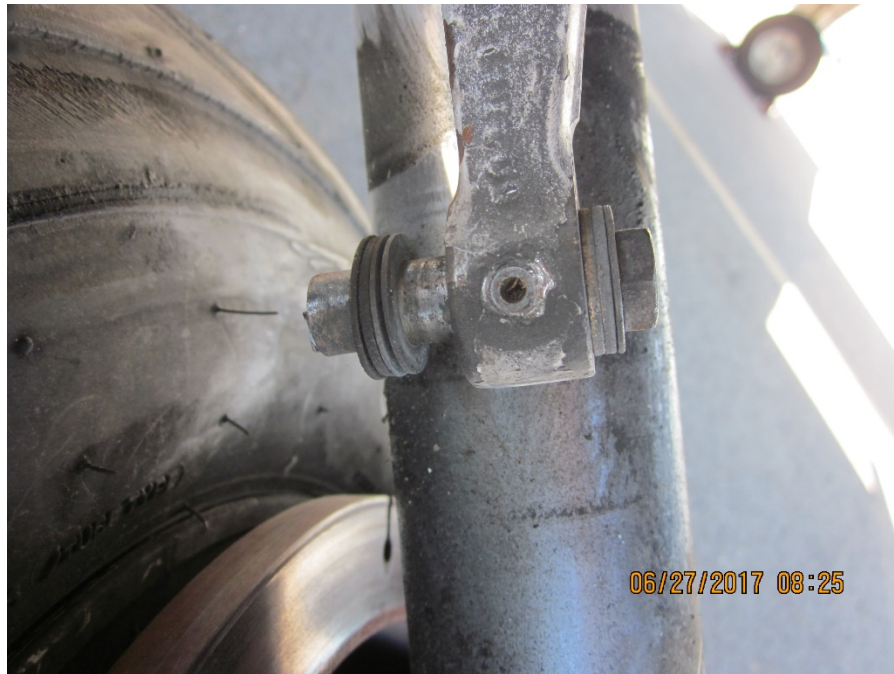
Figure 2: Right main landing gear scissor link pivot bolt. Courtesy of the FAA.
