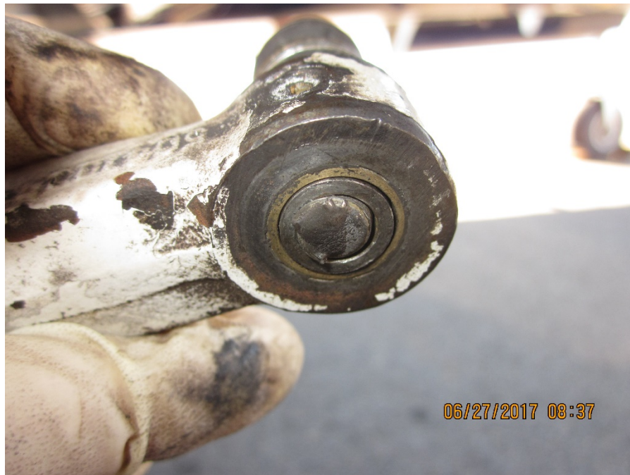
Figure 3: Right main landing gear scissor link pivot bolt. Courtesy of the FAA.
