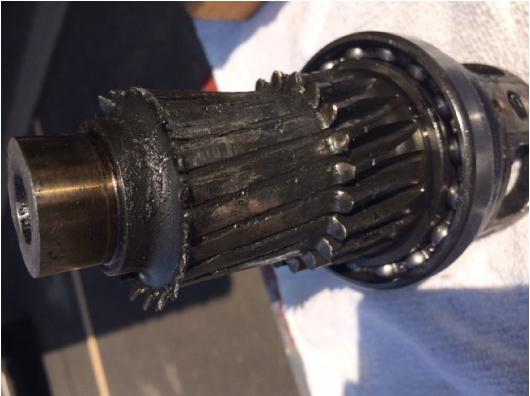
Photo 2 – Gearbox Drive Gear
