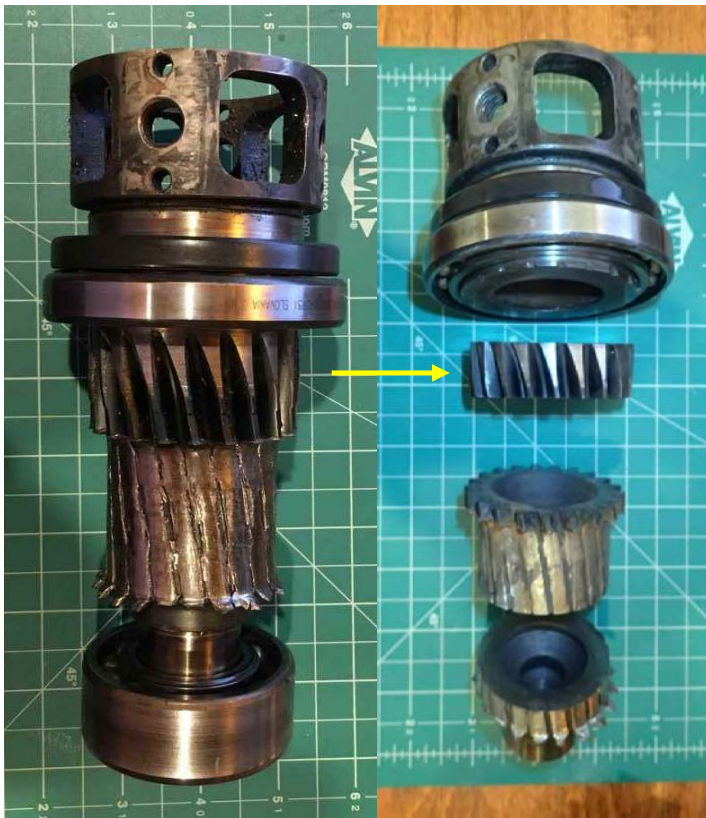
Figure 3. Actual drive gear with arrow pointing to segment received for testing.
