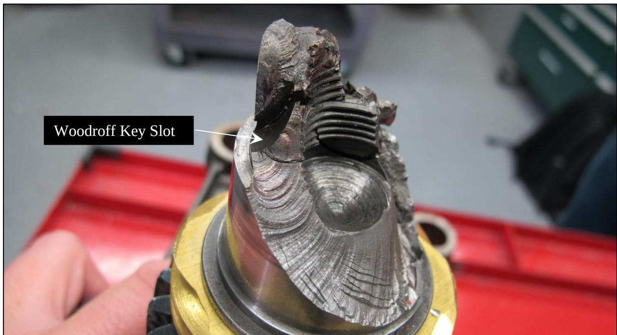
Figure 3-Crankshaft forward separation surface area.
