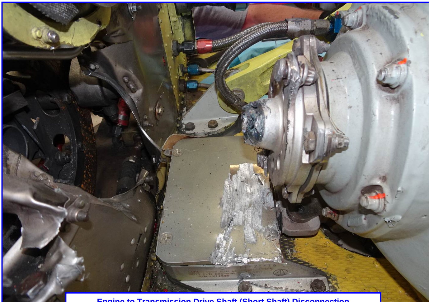
Engine to Transmission Drive Shaft (Short Shaft) Disconnection
