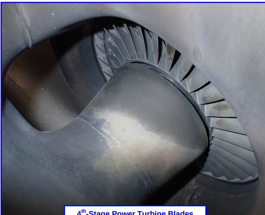
4 th -Stage Power Turbine Blades
