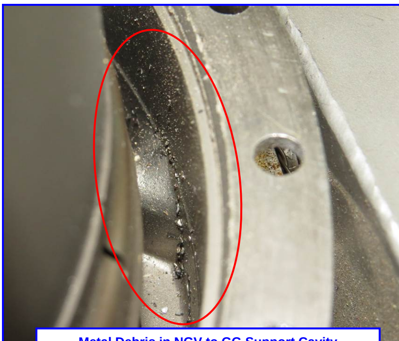
Metal Debris in NGV to GG Support Cavity
