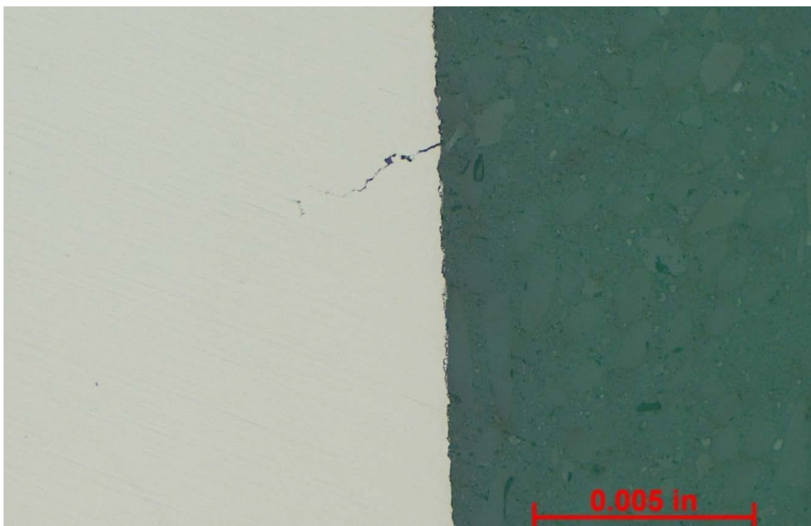
Figure 24 – BF optical micrograph showing the inside bolt hole surface of the flexure element, showing a small crack (as-polished, ~200X).
