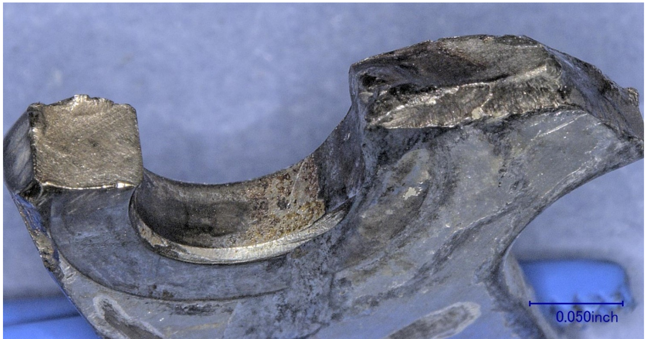
Figure 11 – An angle view of the flexure element fracture surfaces, viewed opposite Figure 8.
