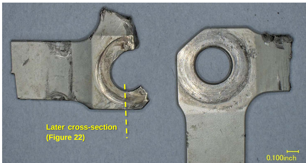
Figure 9 – The circular worn surface of the fractured flexure element (left), compared to an adjacent disassembled flexure element bolt hole, showing wear but no depression (right).
