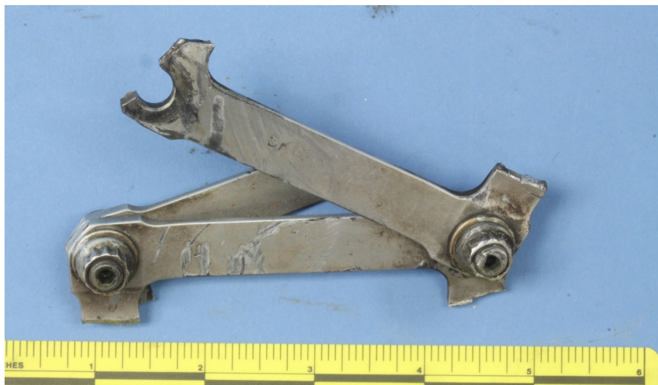
Figure 6 – The fractured flexure elements from Figure 5, viewed from the reverse side.
