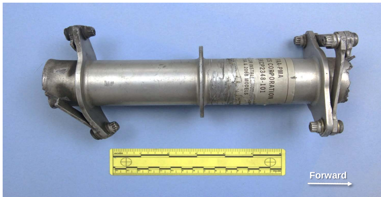
Figure 3 – Closer view of the main shaft, showing the markings and the circumferential gouge marks.
