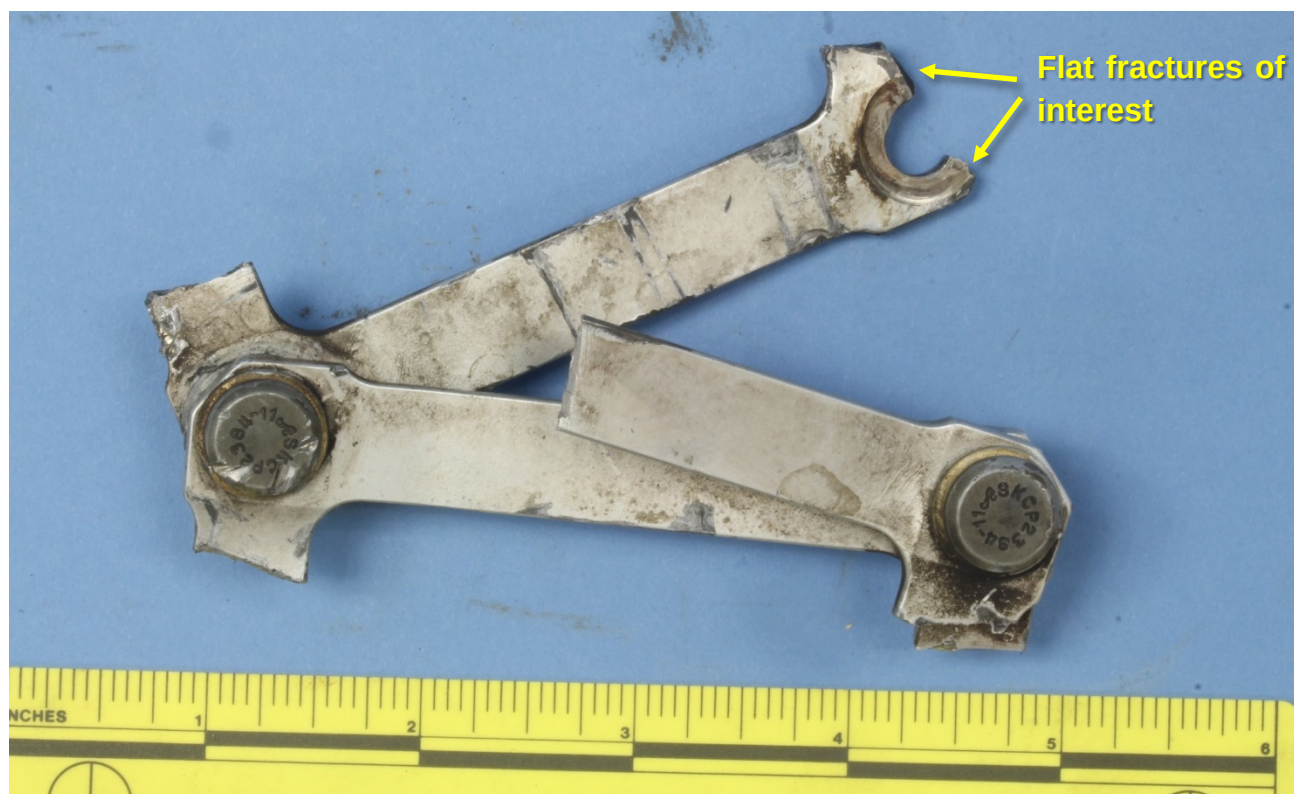
Figure 5 – Some of the fractured flexure elements, showing two flat fractures around a bolt hole of interest.
