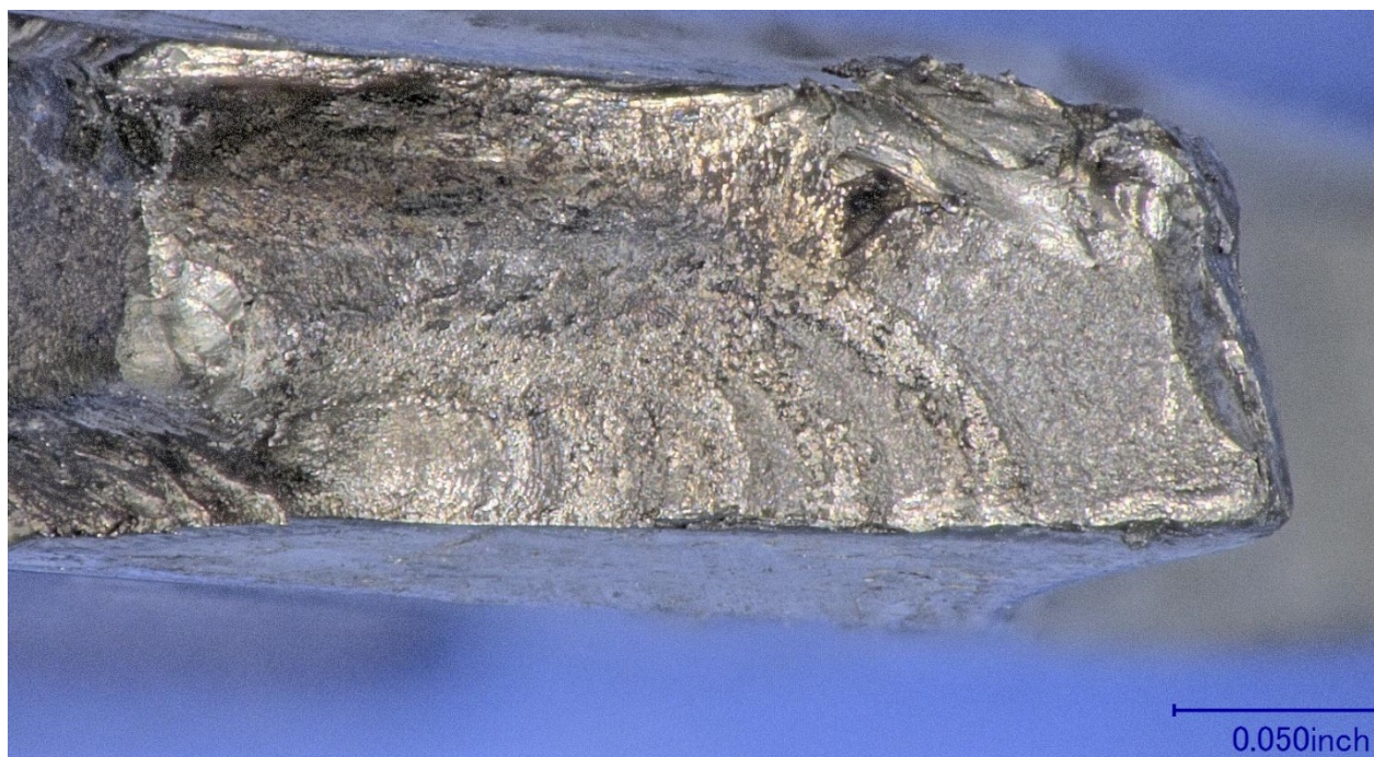
Figure 17 – The right fracture surface of the fractured flexure element in Figure 11.
