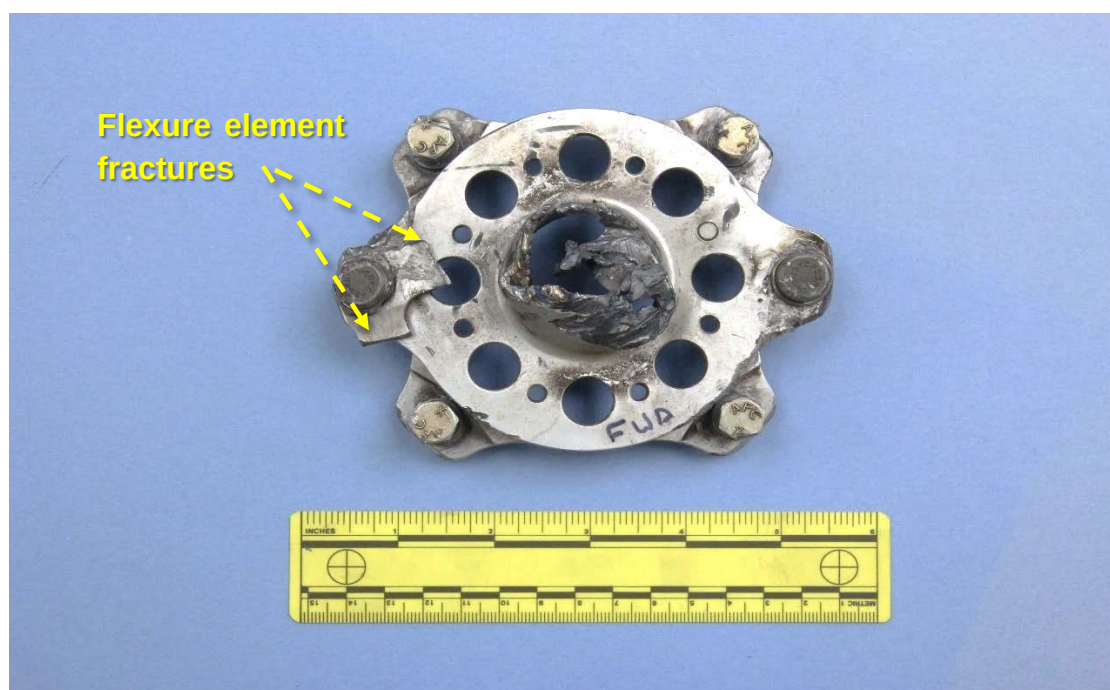
Figure 2 – Closer view of the forward transmission shaft flange, showing shaft fracture and gouging, as well as a flexure element fracture (arrows).
