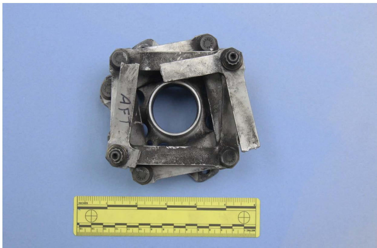
Figure 4 – The remnant of the aft engine shaft flange coupling flexure elements.
