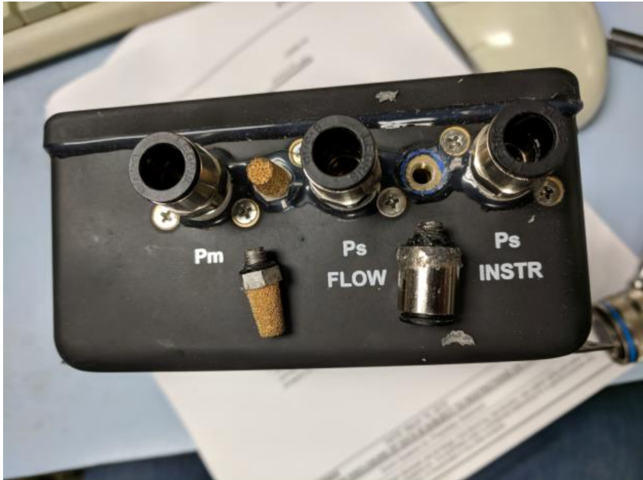
Figure 37 – Cabin air fitting used for ATP testing
