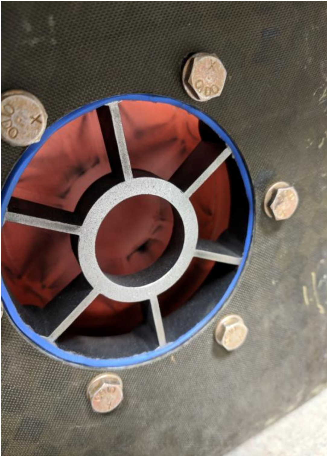
Figure 2 – Back side of outflow valve showing compressed gasket
