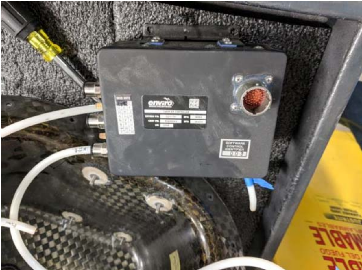
Figure 35 – Pressurization controller 52811-701 SN 05008 SCI 003
