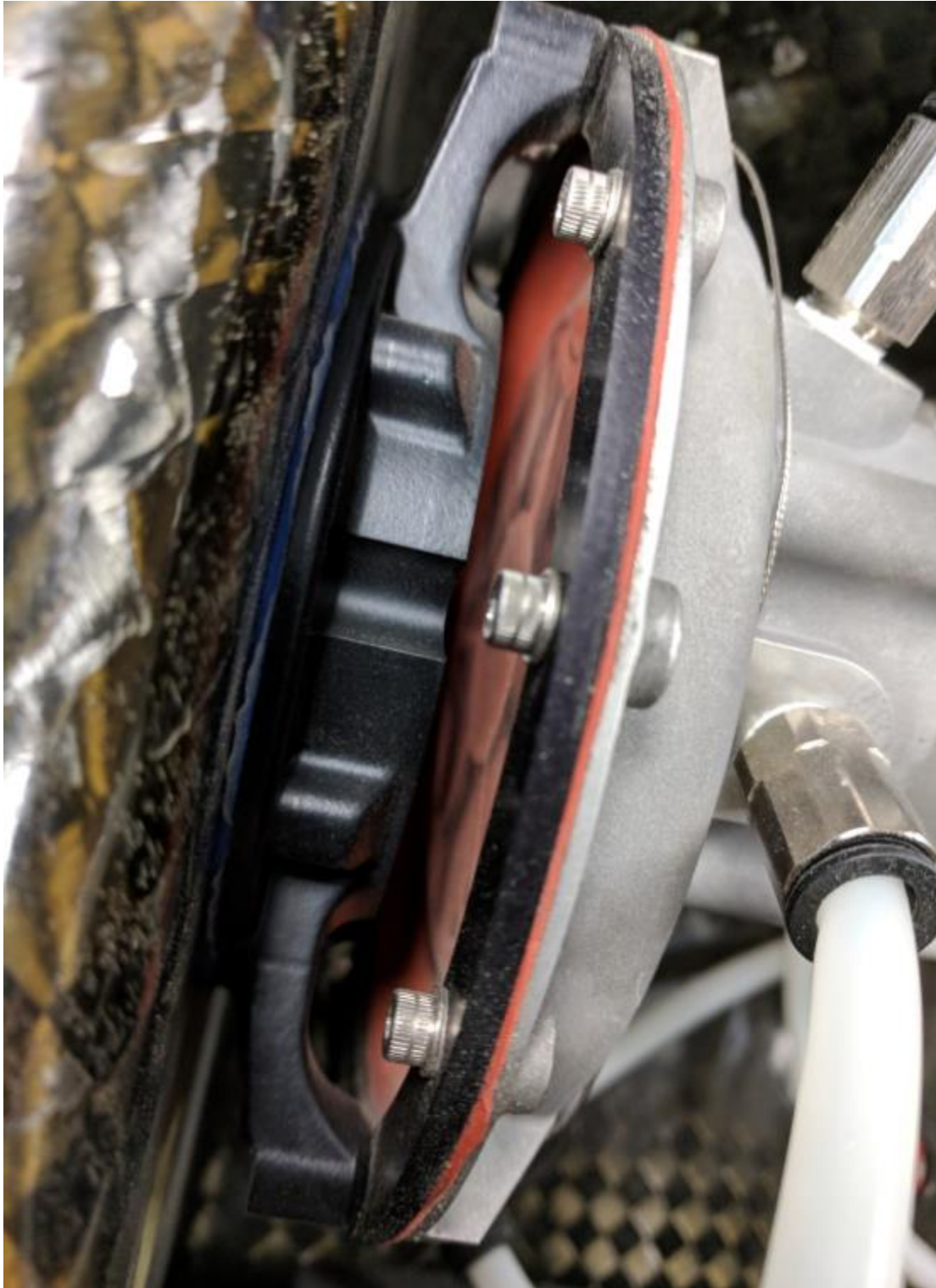
Figure 3 – Side view of outflow valve showing diaphragm in open position
