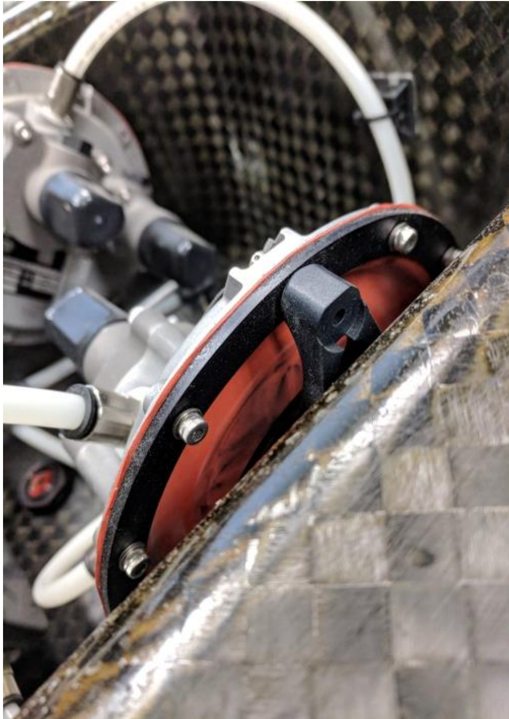
Figure 1 – Installed outflow valve showing diaphragm in open position
