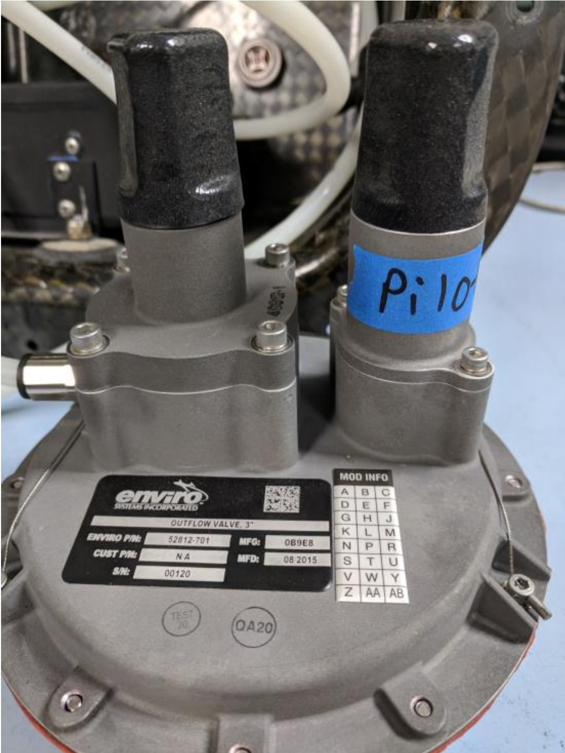
Figure 21 – Outflow valve 52812-701 SN 00120
