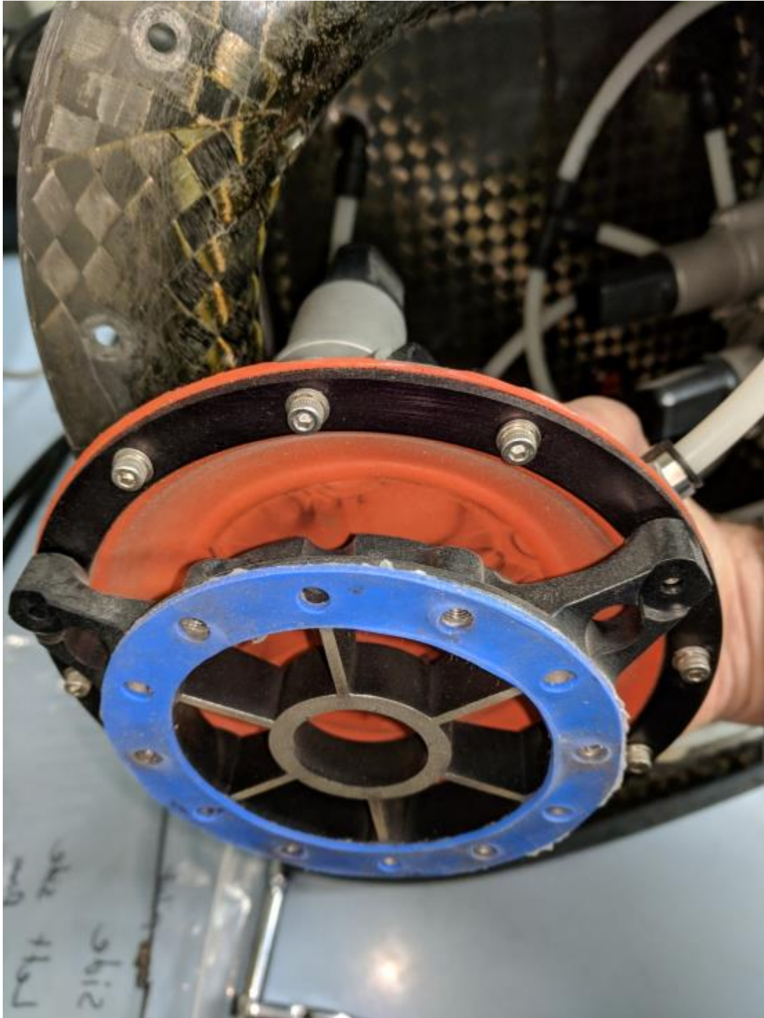
Figure 13 – Removed outflow valve showing open diaphragm
