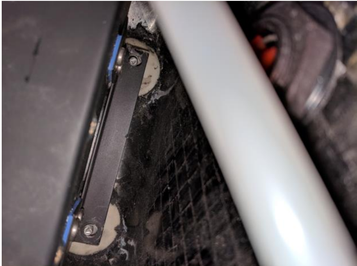
Figure 12 – Rear mounting brackets missing hardware as received
