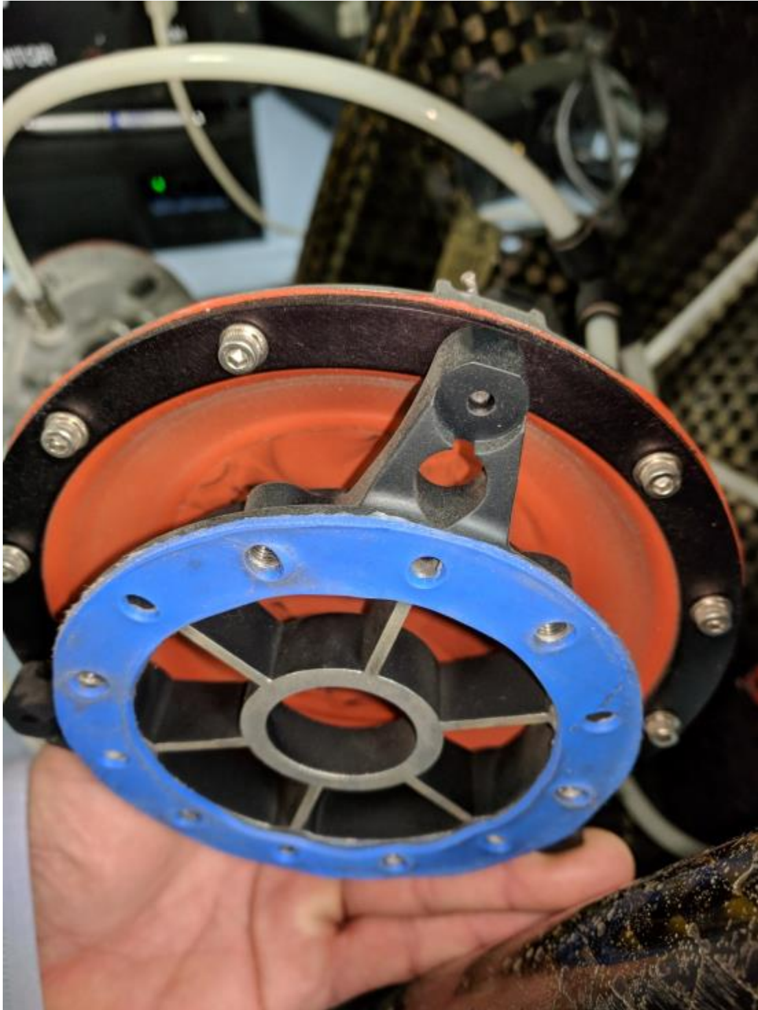
Figure 17 – Removed outflow valve
