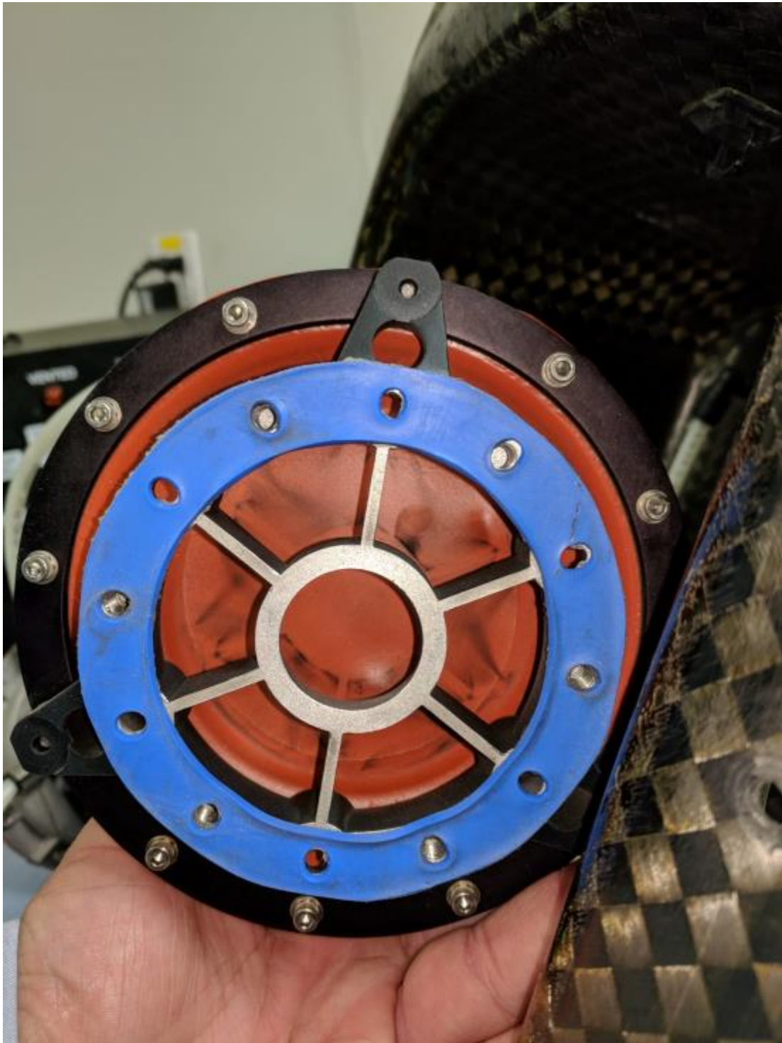
Figure 18 – Bottom side of removed outflow valve
