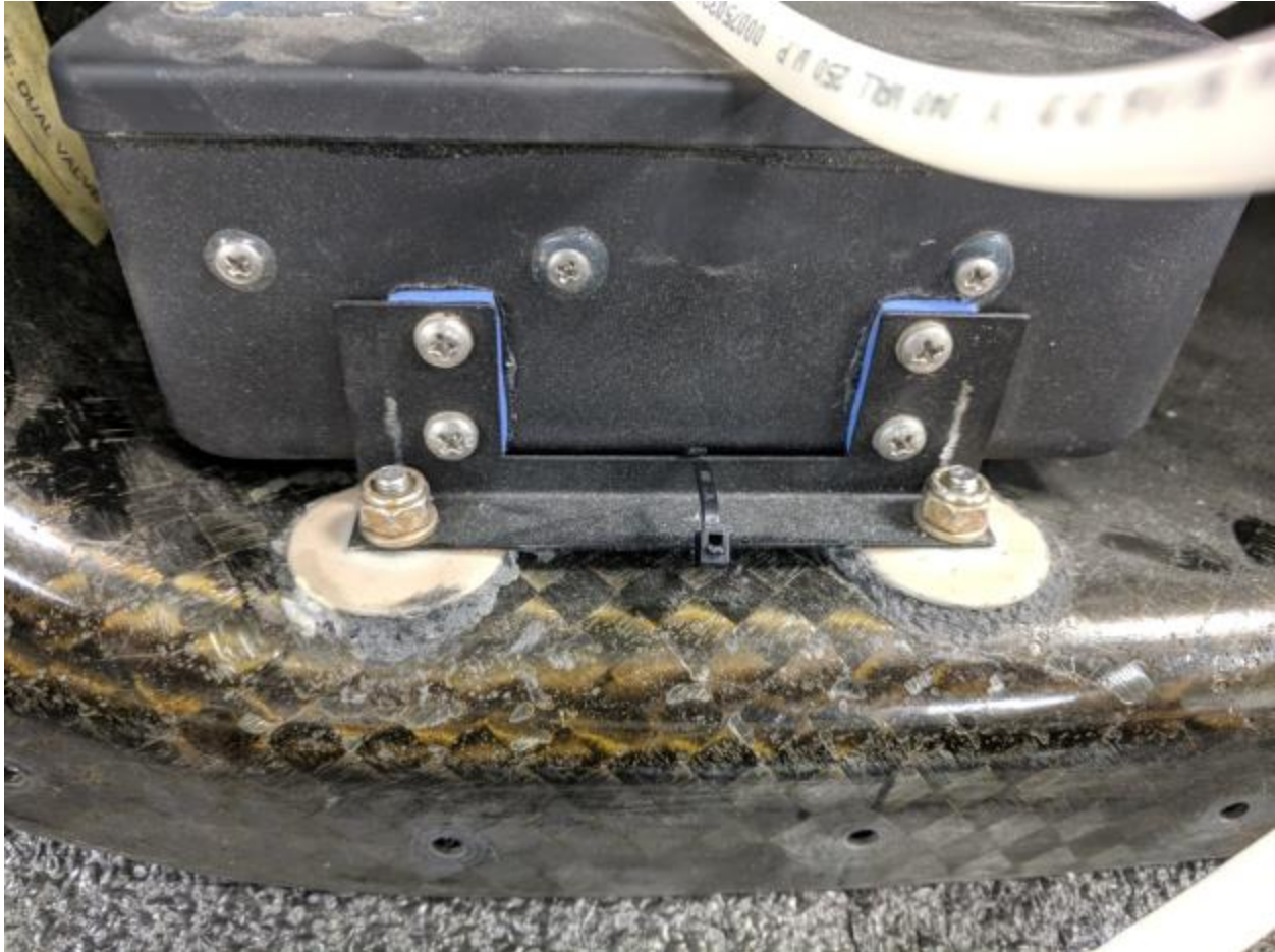
Figure 33 – Controller mounting hardware showing paint damage
