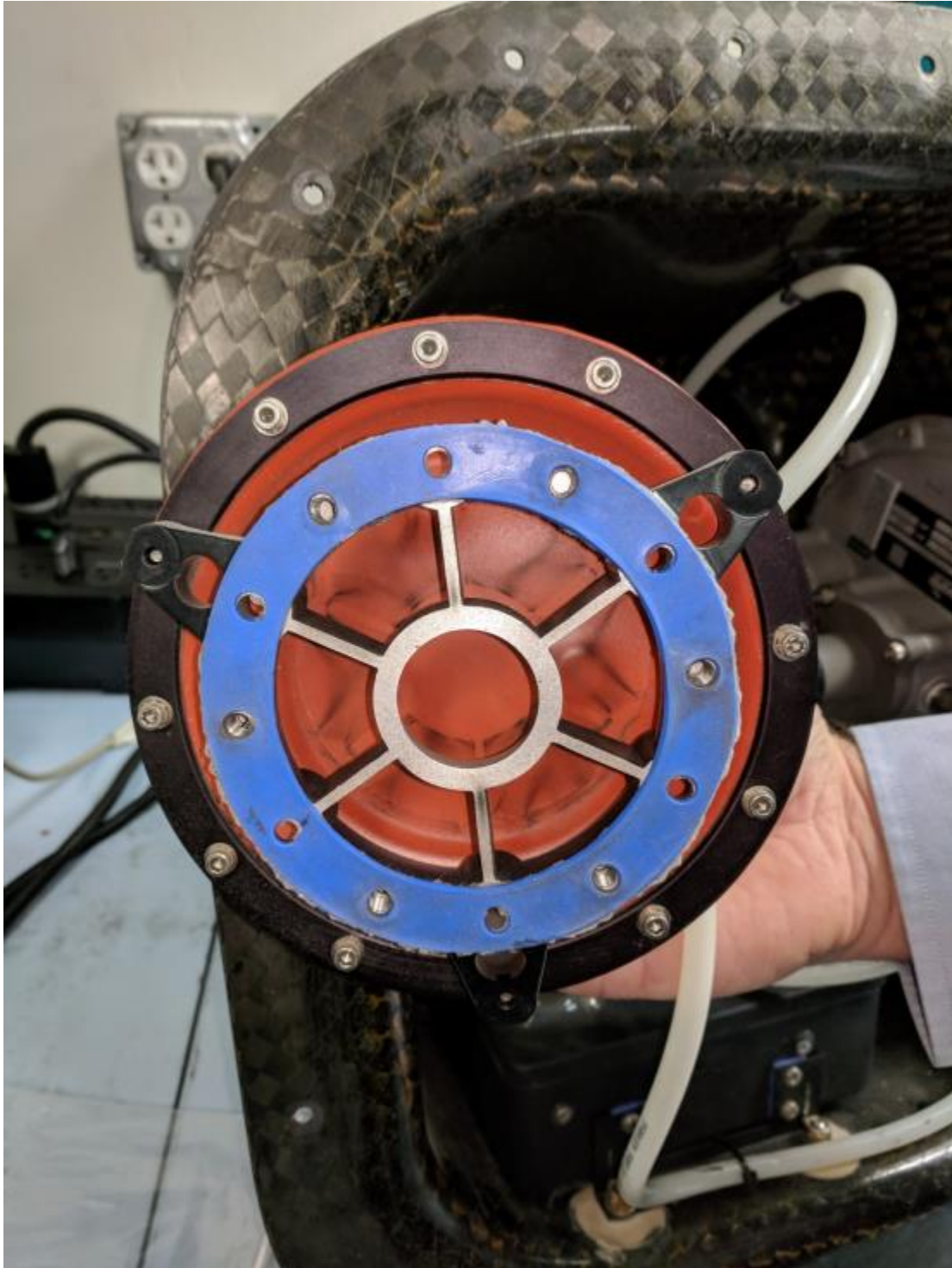
Figure 14 – Bottom side of removed outflow valve
