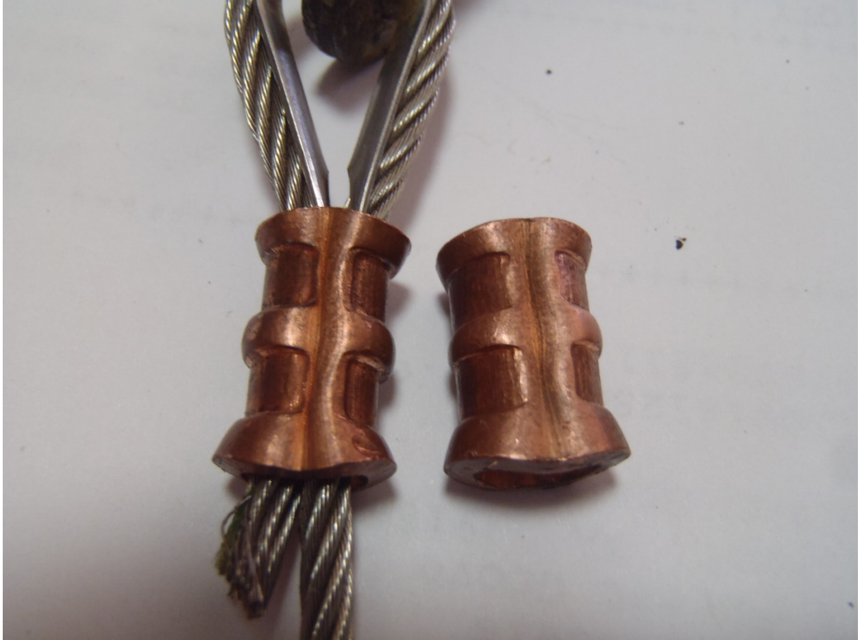
Photo 8. Crimp pressure comparison of the front seat right rudder fore (left) and aft (right) swage sleeves.
