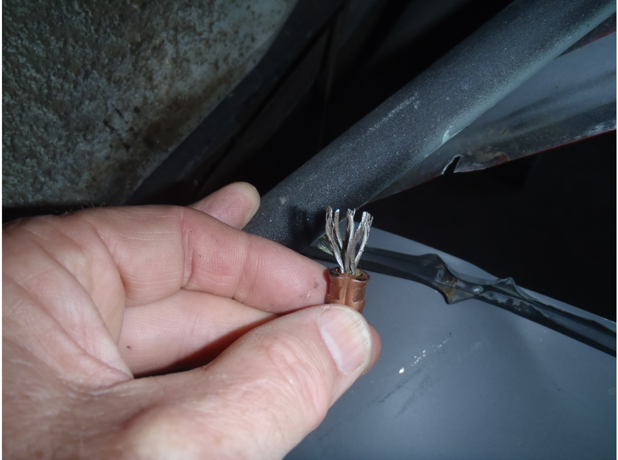
Photo 4. Front seat right rudder cable end with swage sleeve. Cable is attached at the front seat rudder pedal.
