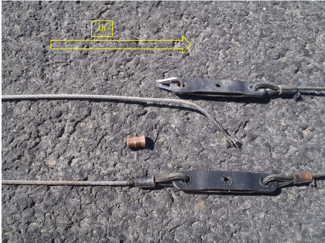
Photo 6. Rear seat left (lower) and right (upper) rudder cable assemblies.
