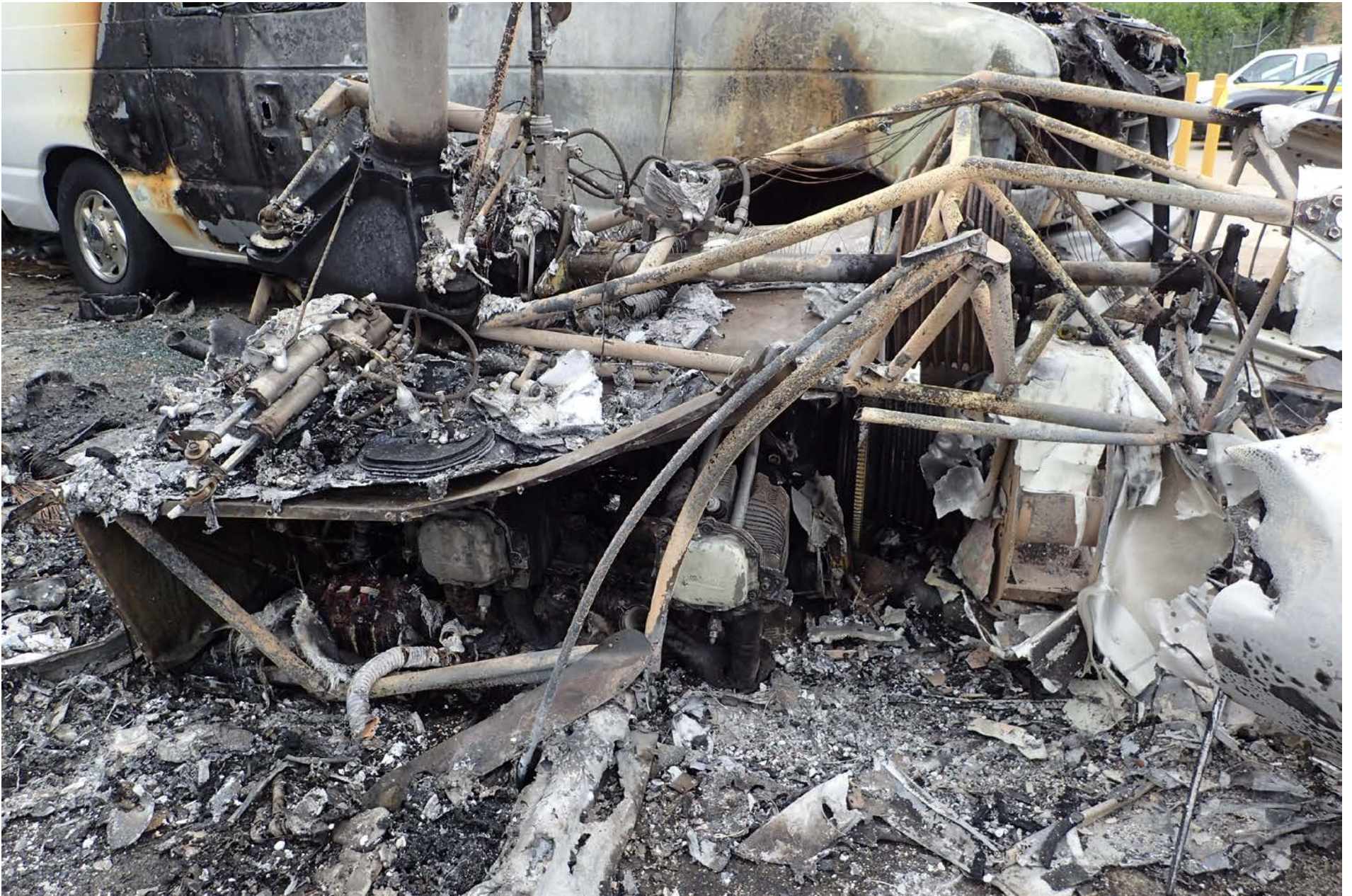
Photo 2 – Engine Bay with Cylinder #3 Absent
