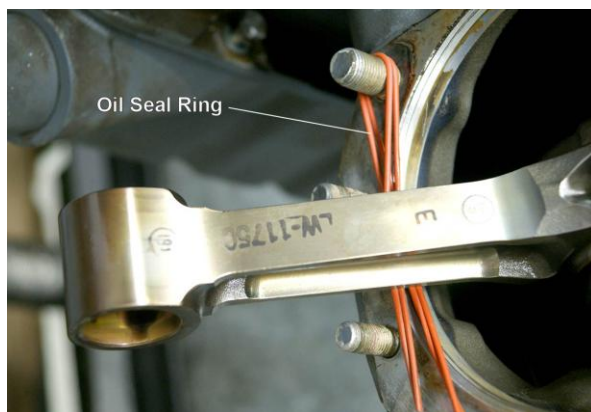
Figure 2 Oil Seal Ring Installed on the Crankcase Studs
