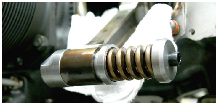
Figure 5 ST-531 Installed in the Connecting Rod
