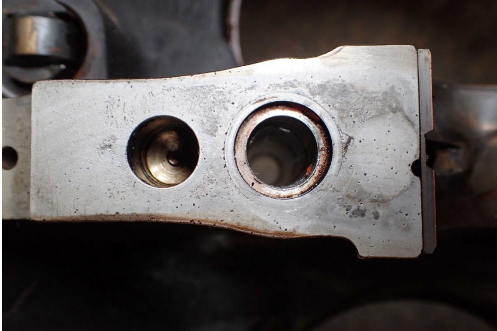
Photo 15 – Pitting at Crankcase Web
