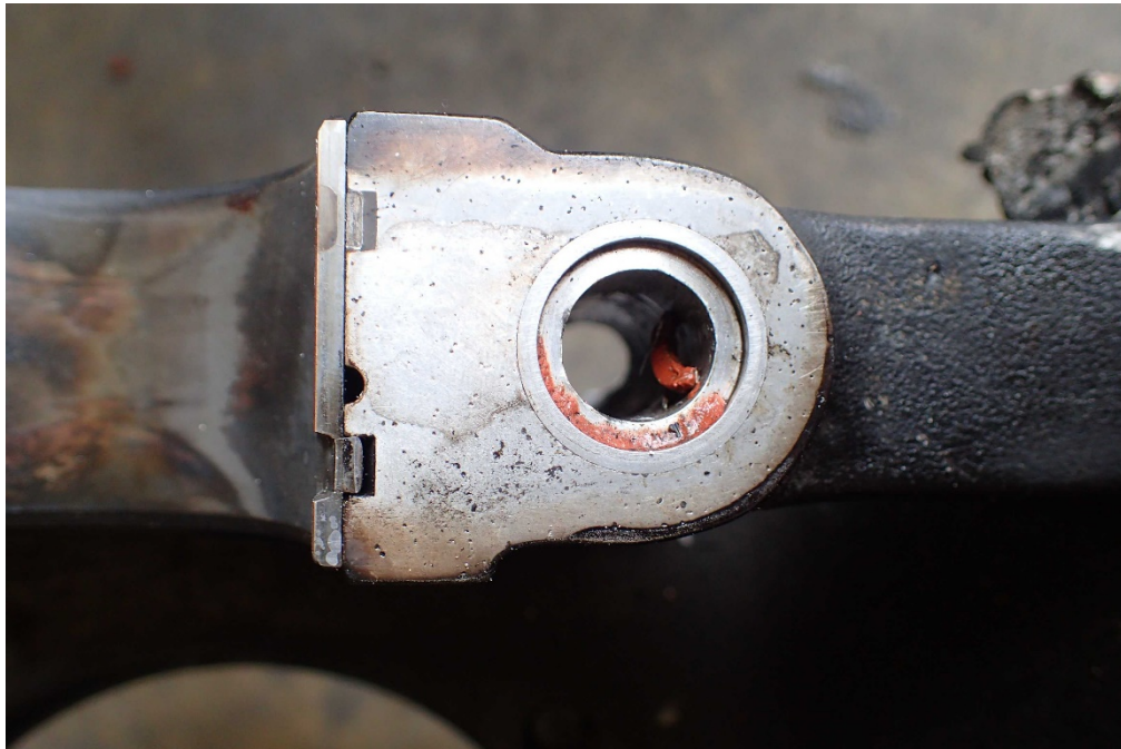
Photo 14 – Pitting at Crankcase Web
