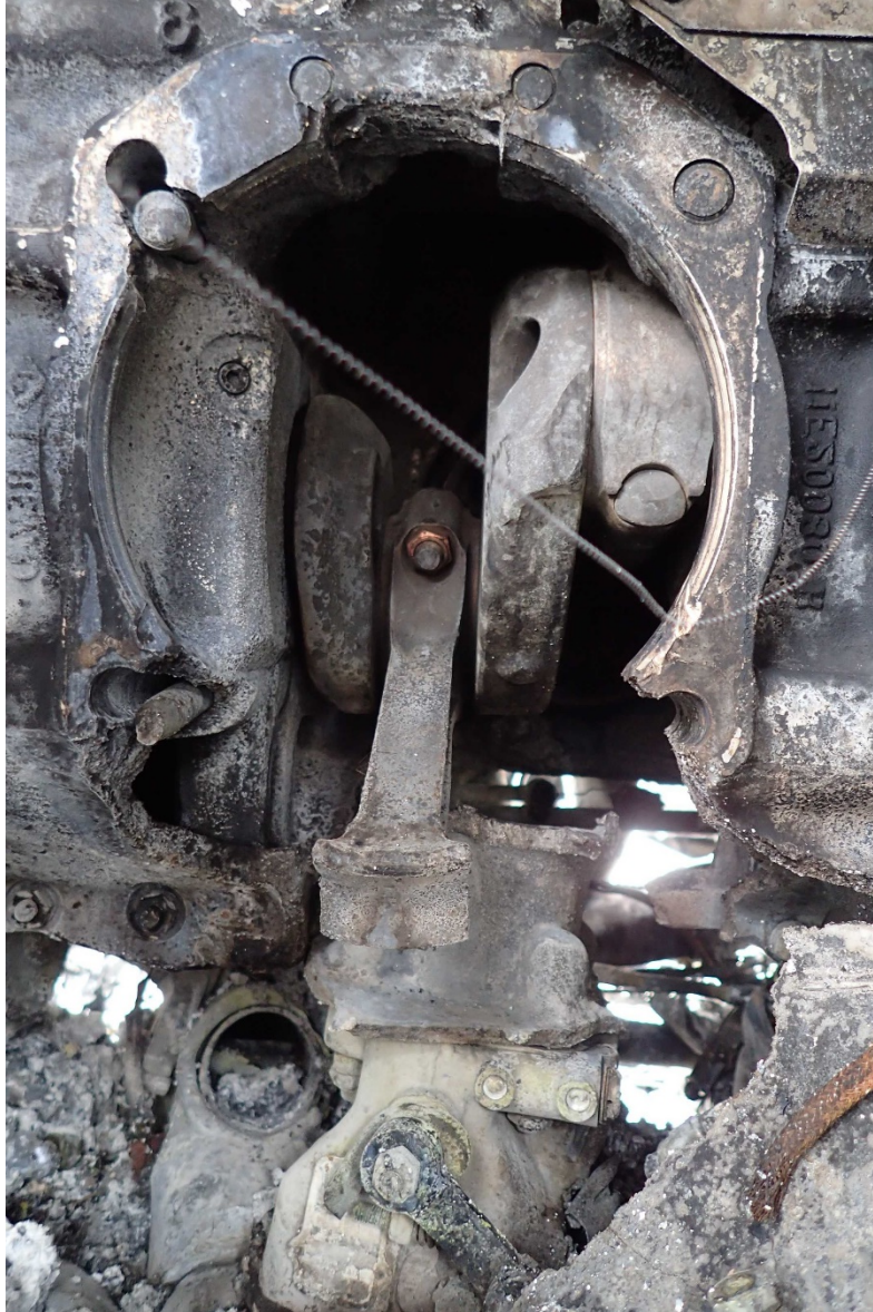
Photo 4 – Number 3 Connecting Rod
