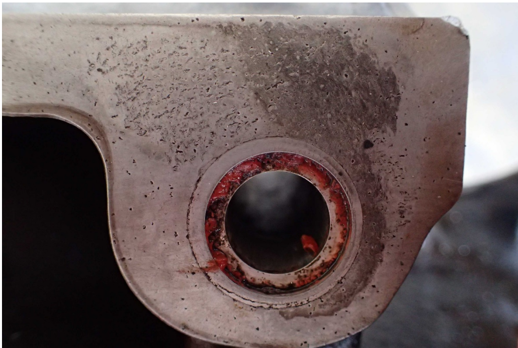
Photo 16 - Pitting at Forward Bearing Crankcase Saddle
