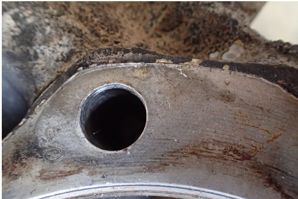
Photo 10 – Gouging on Crankcase to Cylinder Flange Deck Surface
