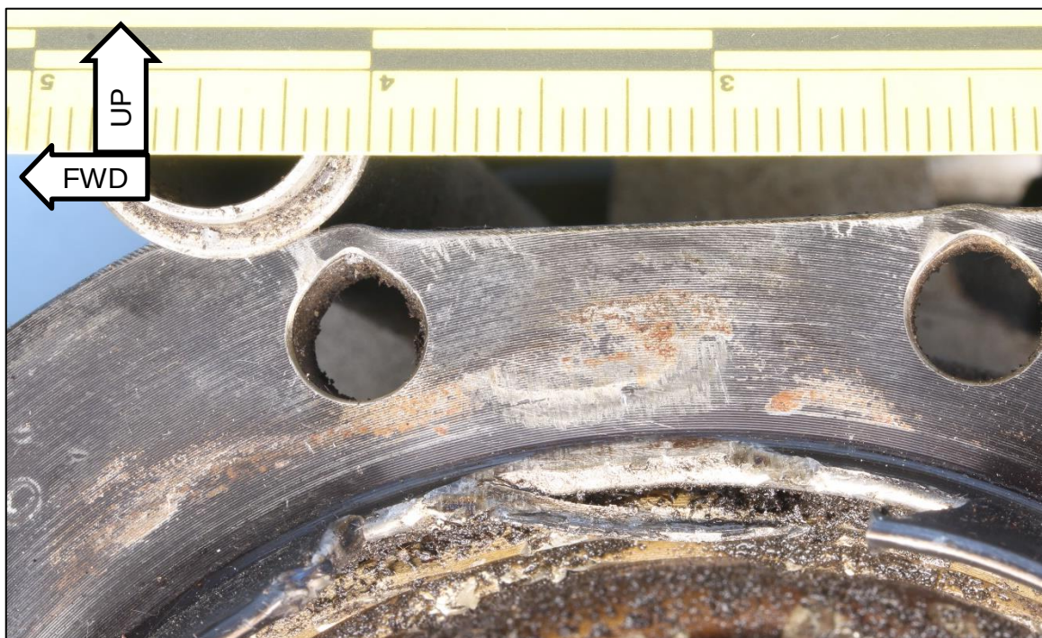
Figure 10. Elongated holes at upper side of the number 3 cylinder flange showing deformation consistent with the cylinder moving downward relative to the attachment studs.
