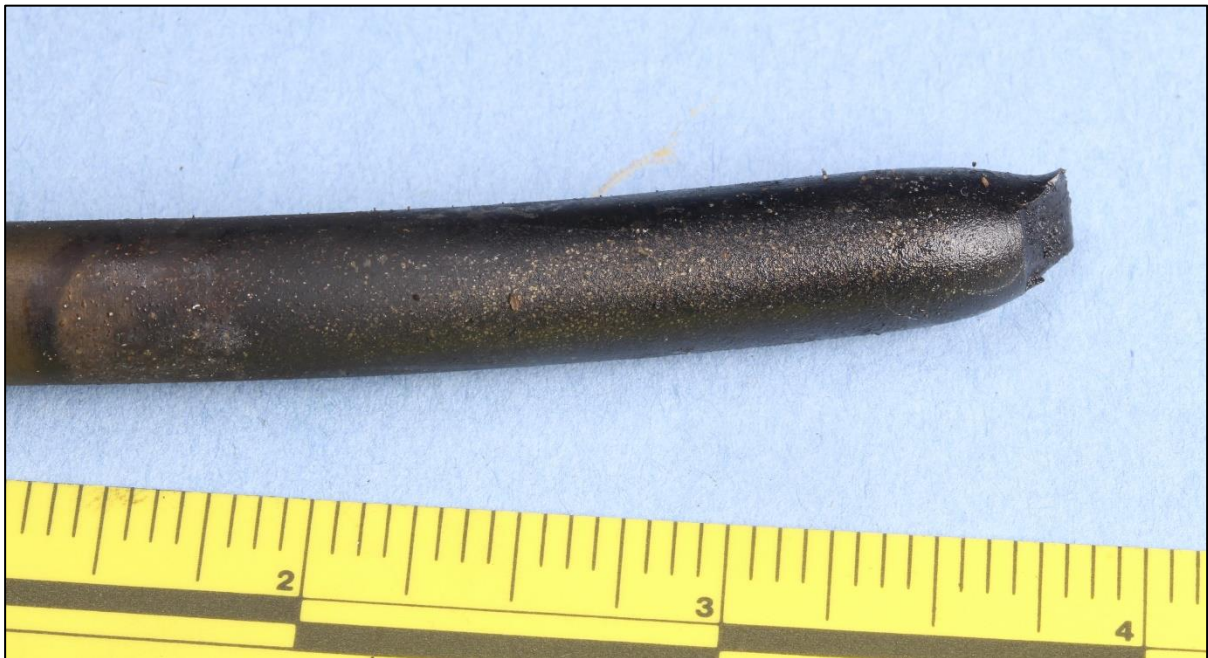
Figure 13. Overstress fracture of the lower throughbolt at the forward side of the number 3 cylinder.
