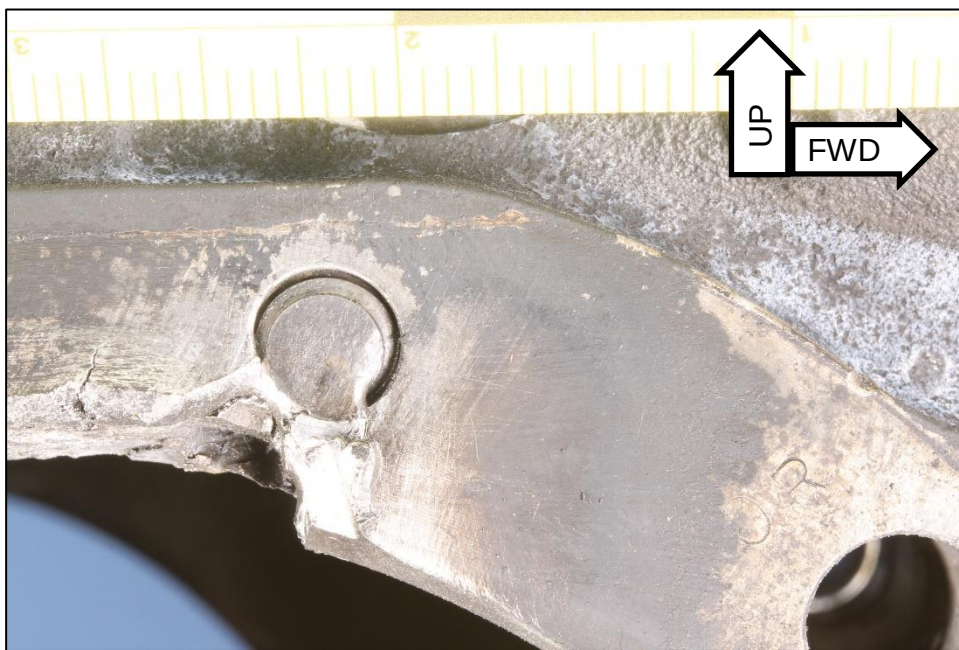
Figure 6. Close view of the stud fracture at the upper middle forward attachment location for the number 3 cylinder.
