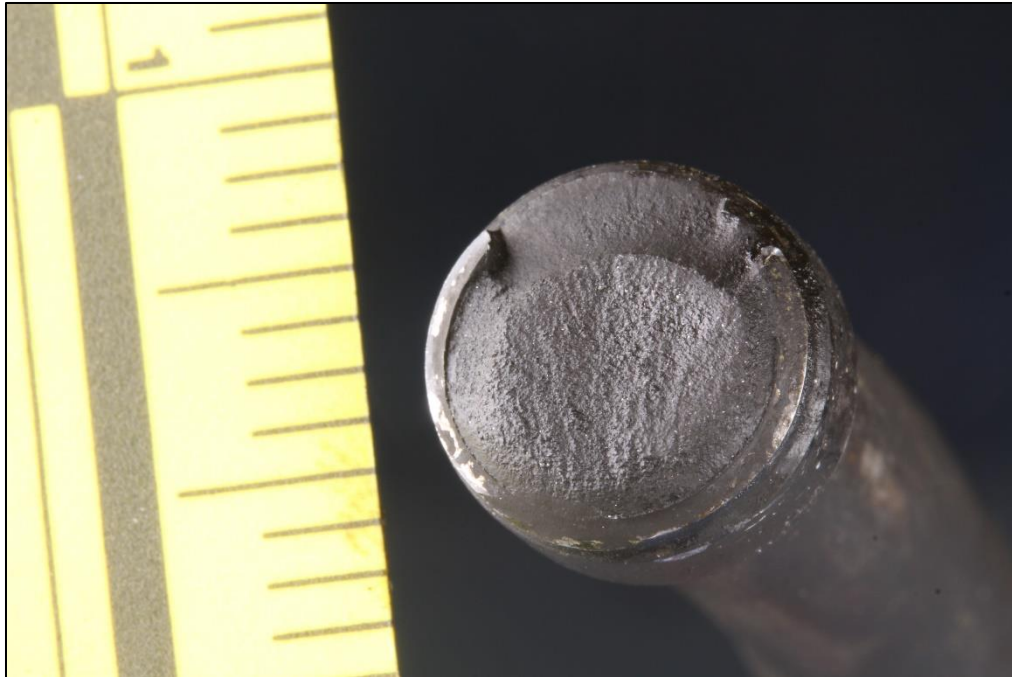
Figure 12. Overstress fracture of upper throughbolt at the forward side of the number 3 cylinder.
