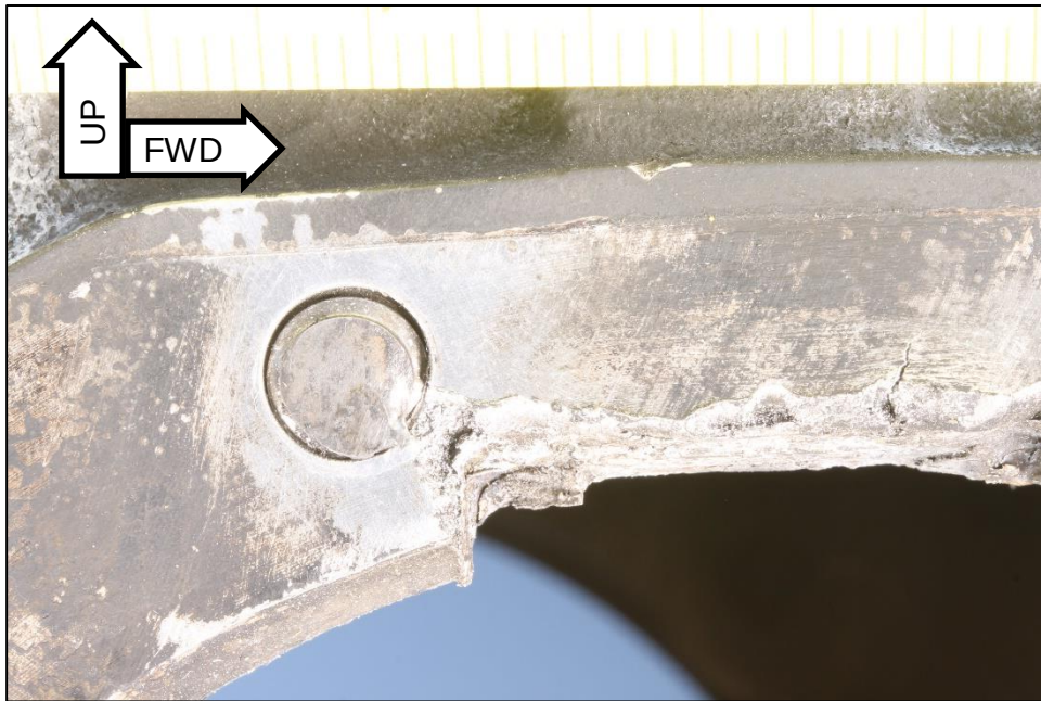
Figure 7. Close view of the stud fracture at the upper middle aft attachment location for the number 3 cylinder.
