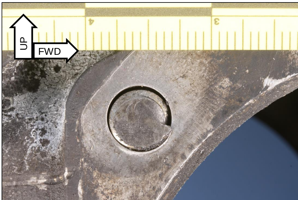
Figure 8. Close view of the stud fracture at the upper aft attachment location for the number 3 cylinder.
