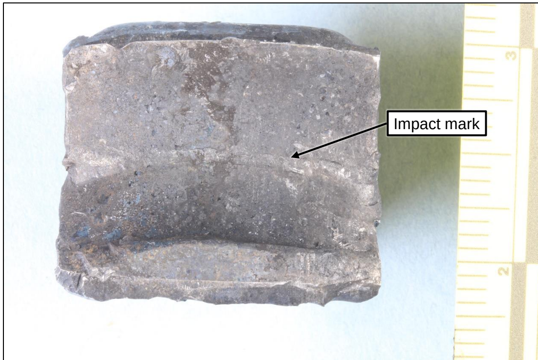
Figure 21. Connecting rod from the number 3 cylinder. The outboard end shown in the lower image had a curved impact mark with a geometry consistent with contact with the inboard end of the cylinder barrel skirt.
