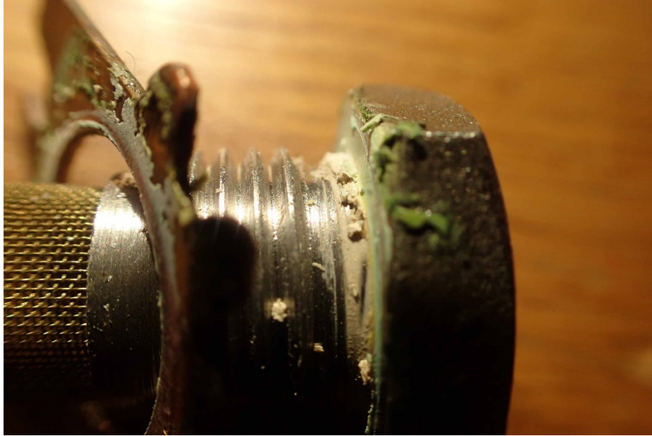
Photo 7- Fuel Inlet Screen Sealant
