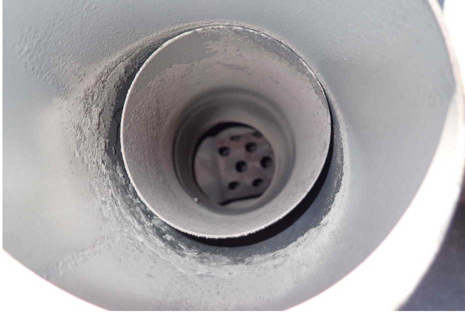
Photo 7- Internal Muffler Baffling after the Engine Run
