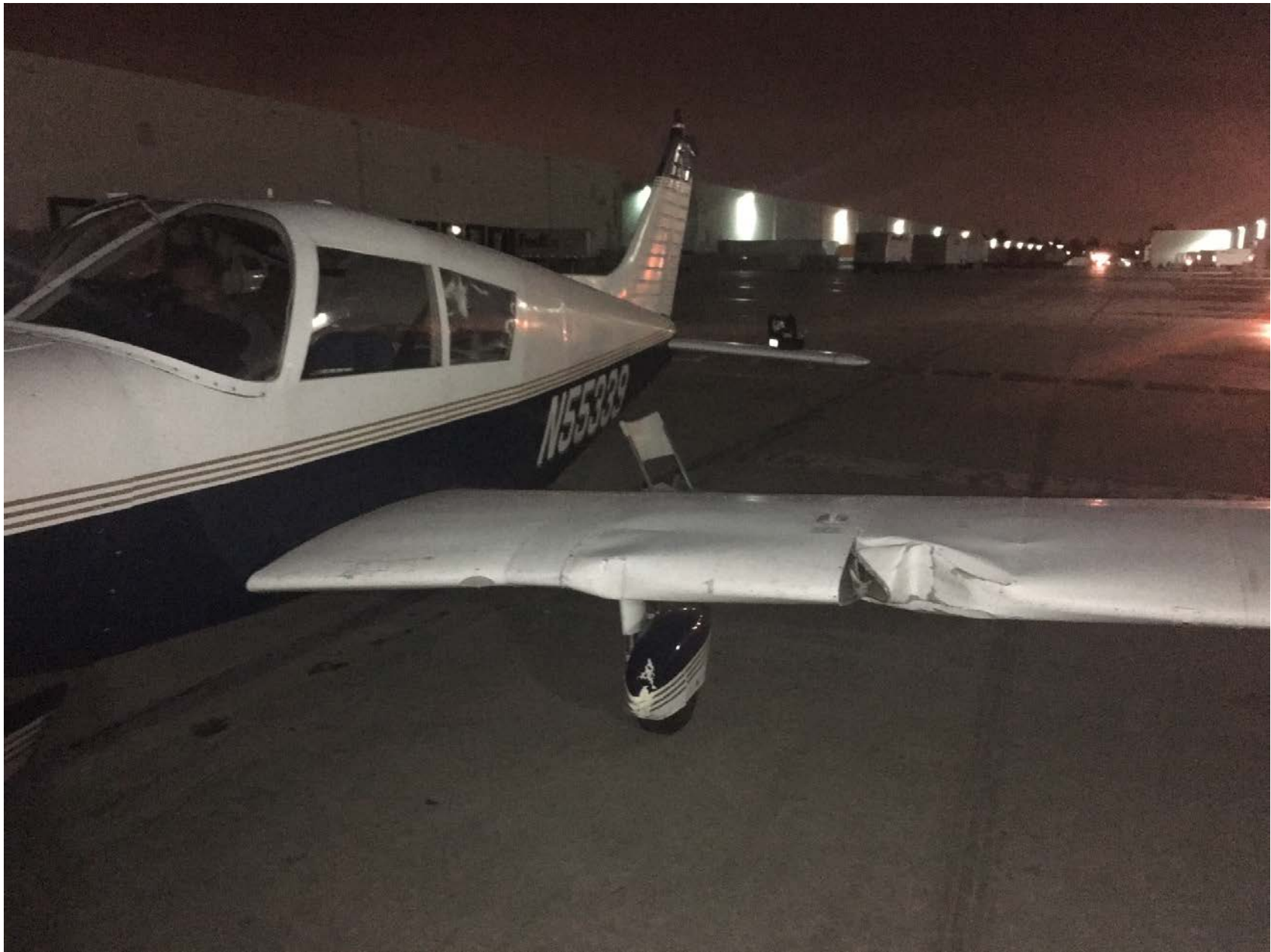
Photo 1 – Damage to the Airplane’s Left Wing
