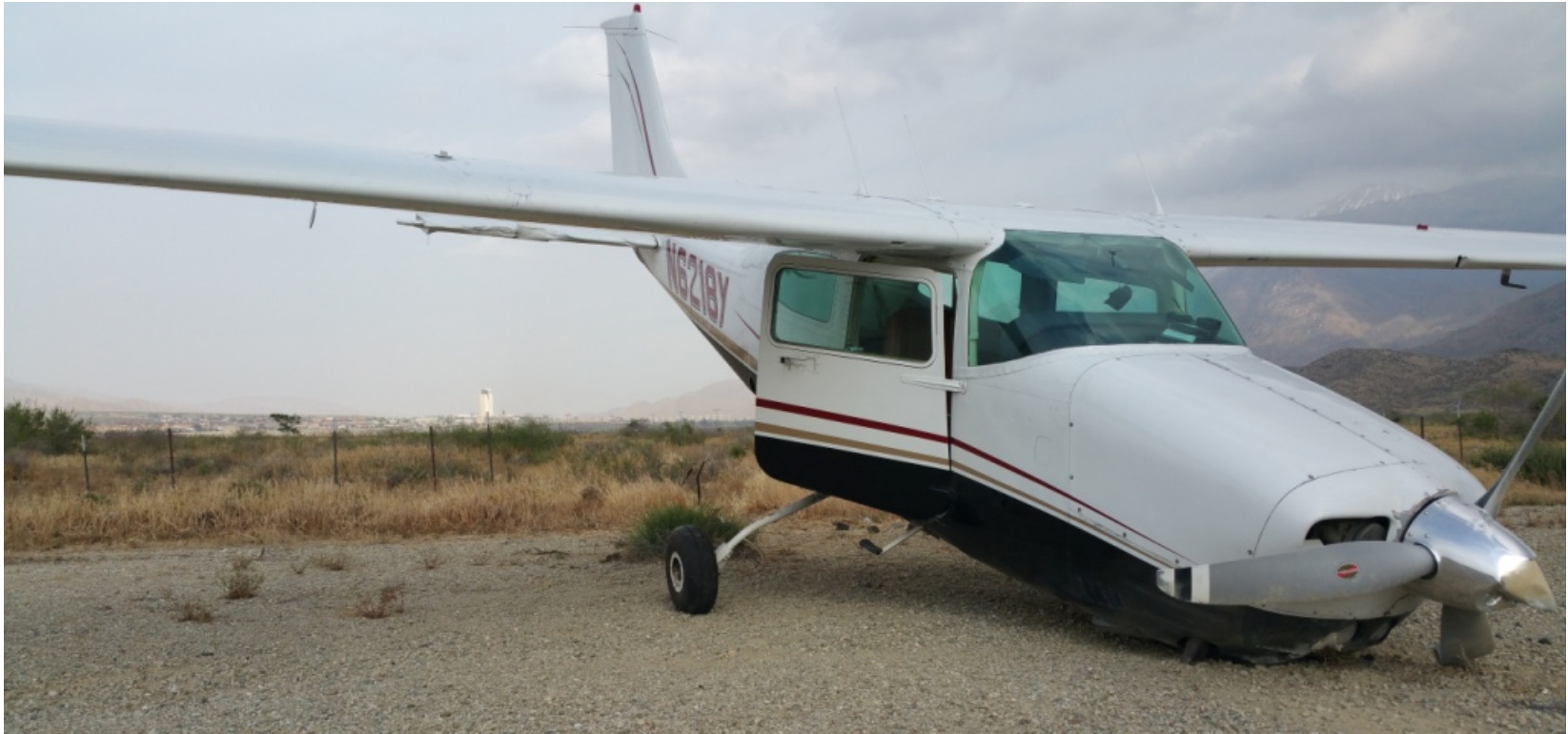
Figure 1 - Airplane with Collapsed NLG at Final Stopping Point
