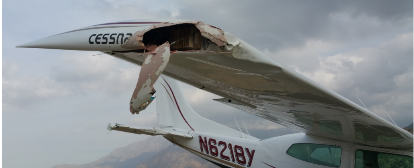
Figure 2 - Damaged Right Wing Outboard Section
