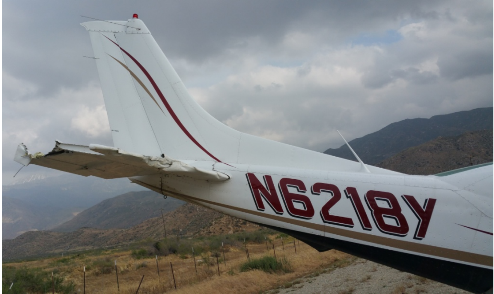
Figure 3 - Damaged Tailcone and Right Horizontal Stabilizer
