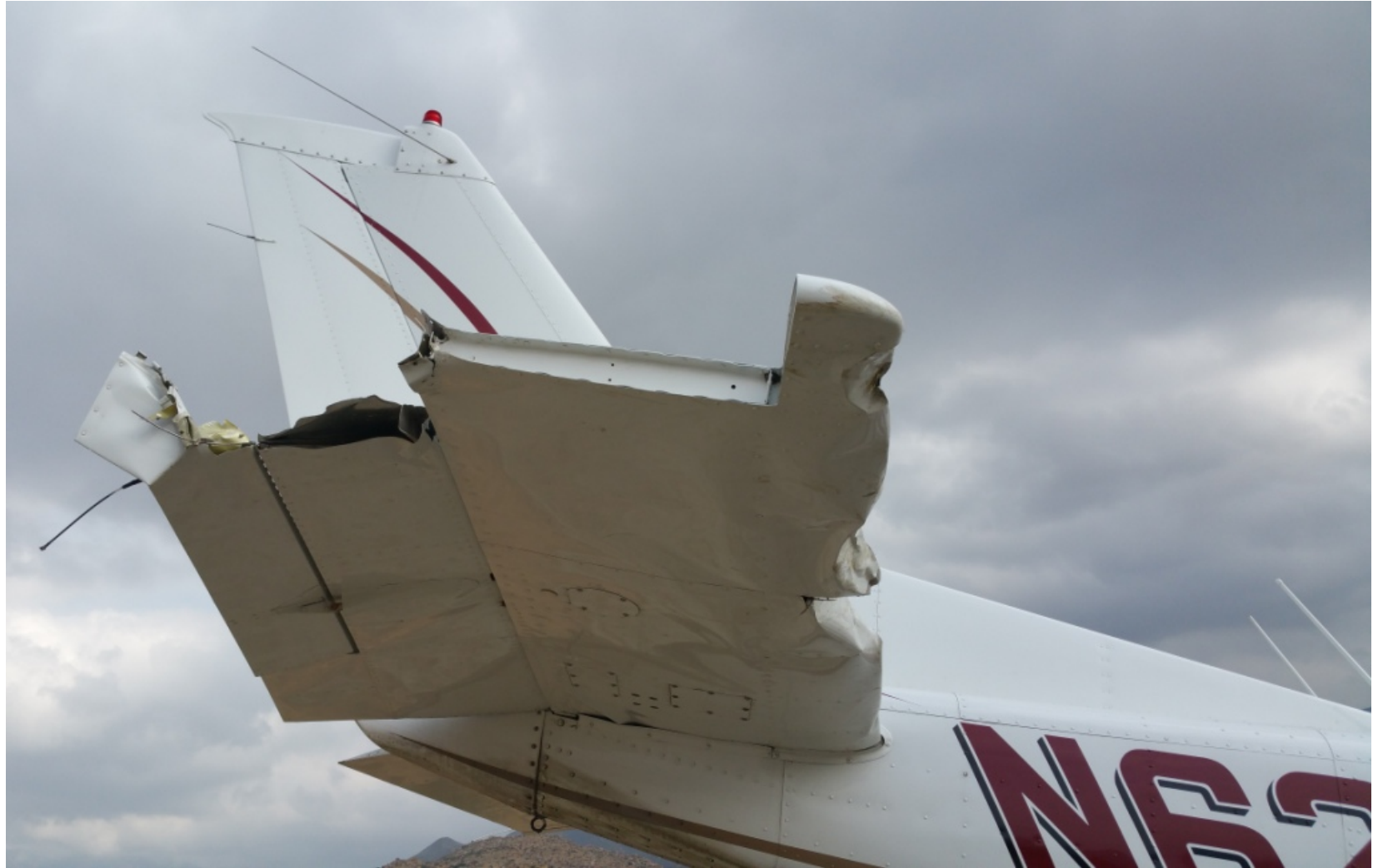
Figure 4 - Damaged Right Horizontal Stabilizer and Elevator
