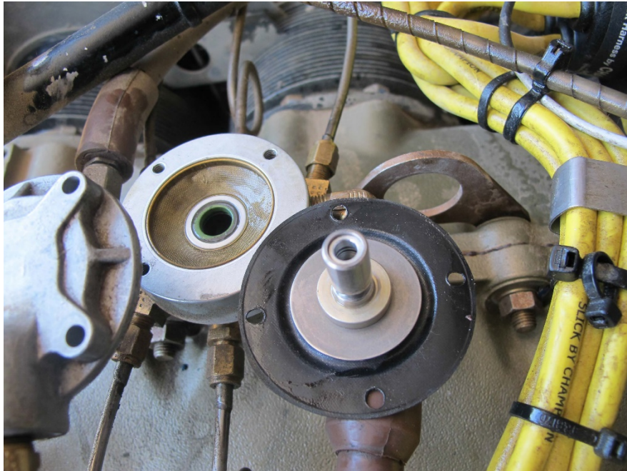
Figure 5 - Screen and Diaphragm of Fuel Manifold Distribution Valve
