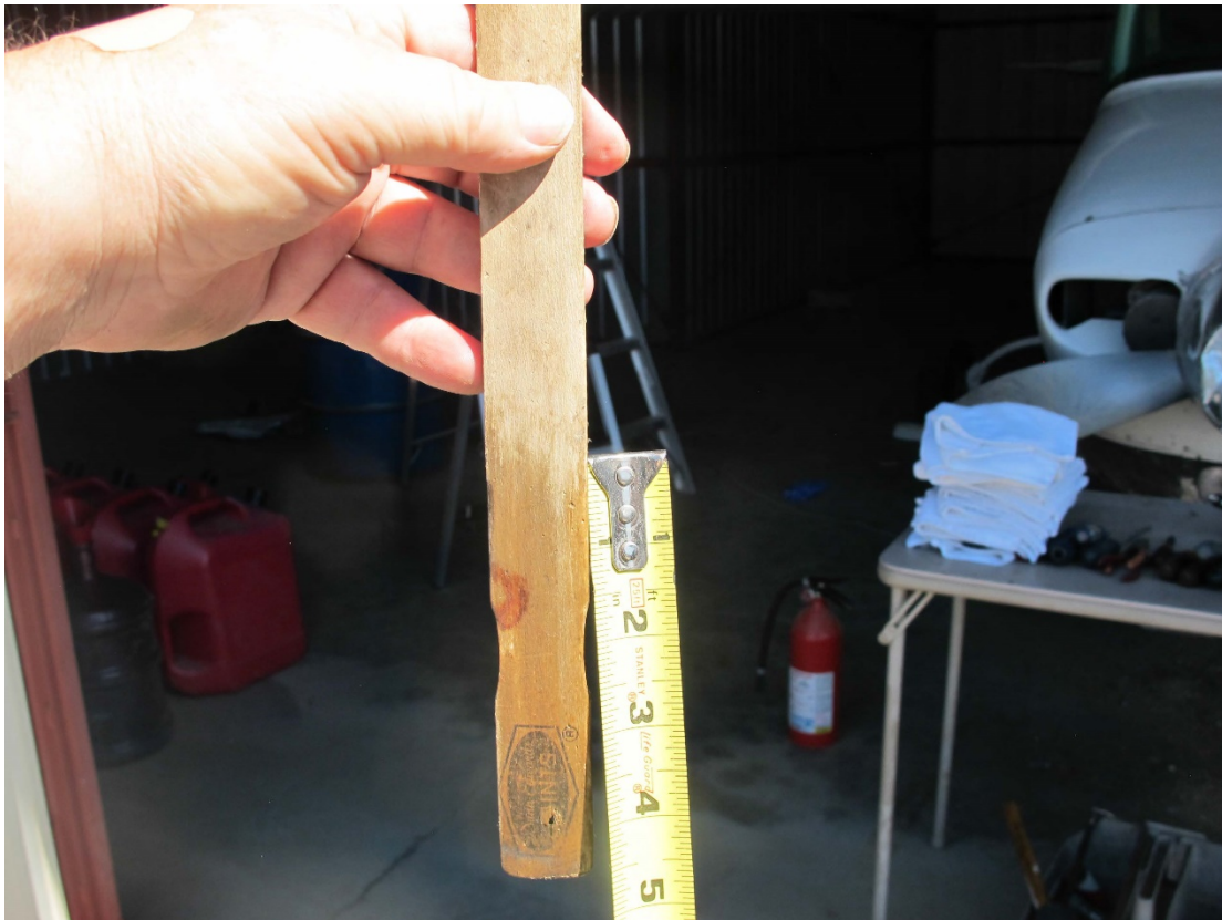
Figure 4 - Right Wing Fuel Measurement
