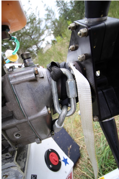
Figure 3: View of parachute line wrapped around propeller shaft.
