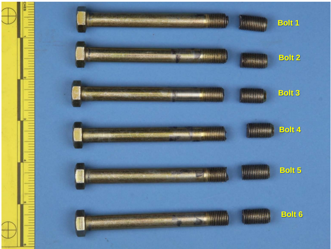
Figure 1 – The six fractured propeller bolts, as received.
