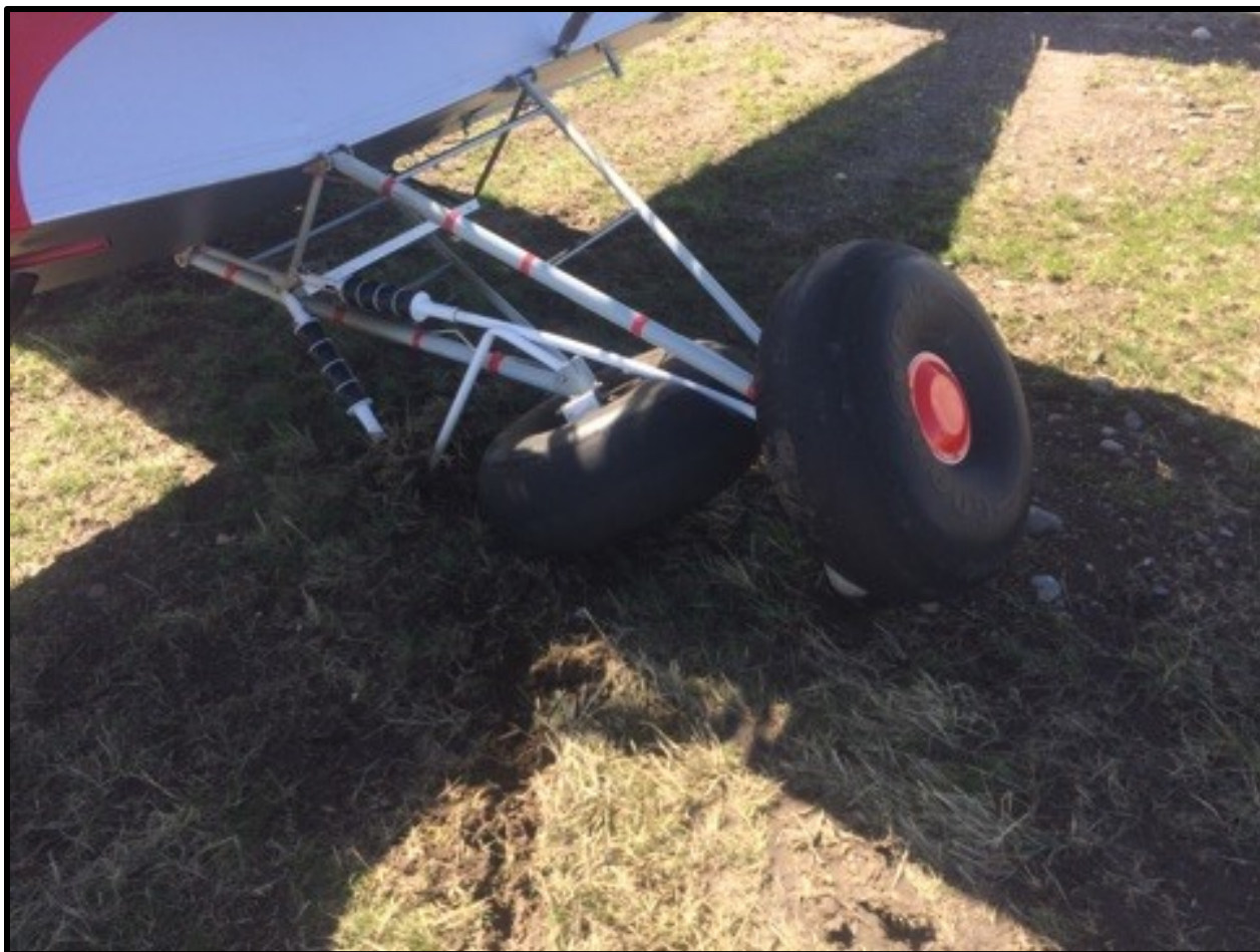
Figure 1: Left side view of airplane, showing the right gear assembly (long and extended design) collapsed.
