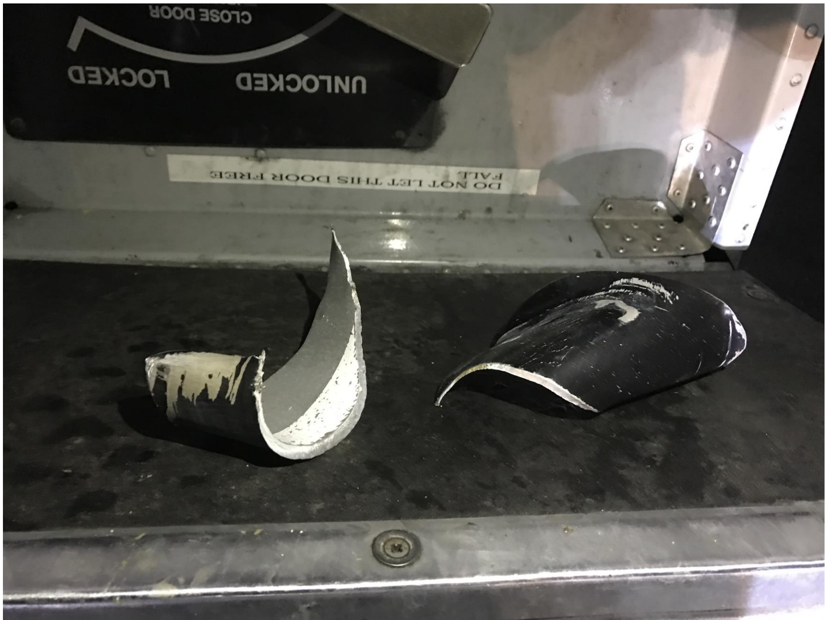
Photo 3 – remnants of blade tip at rest in cabin of airplane
