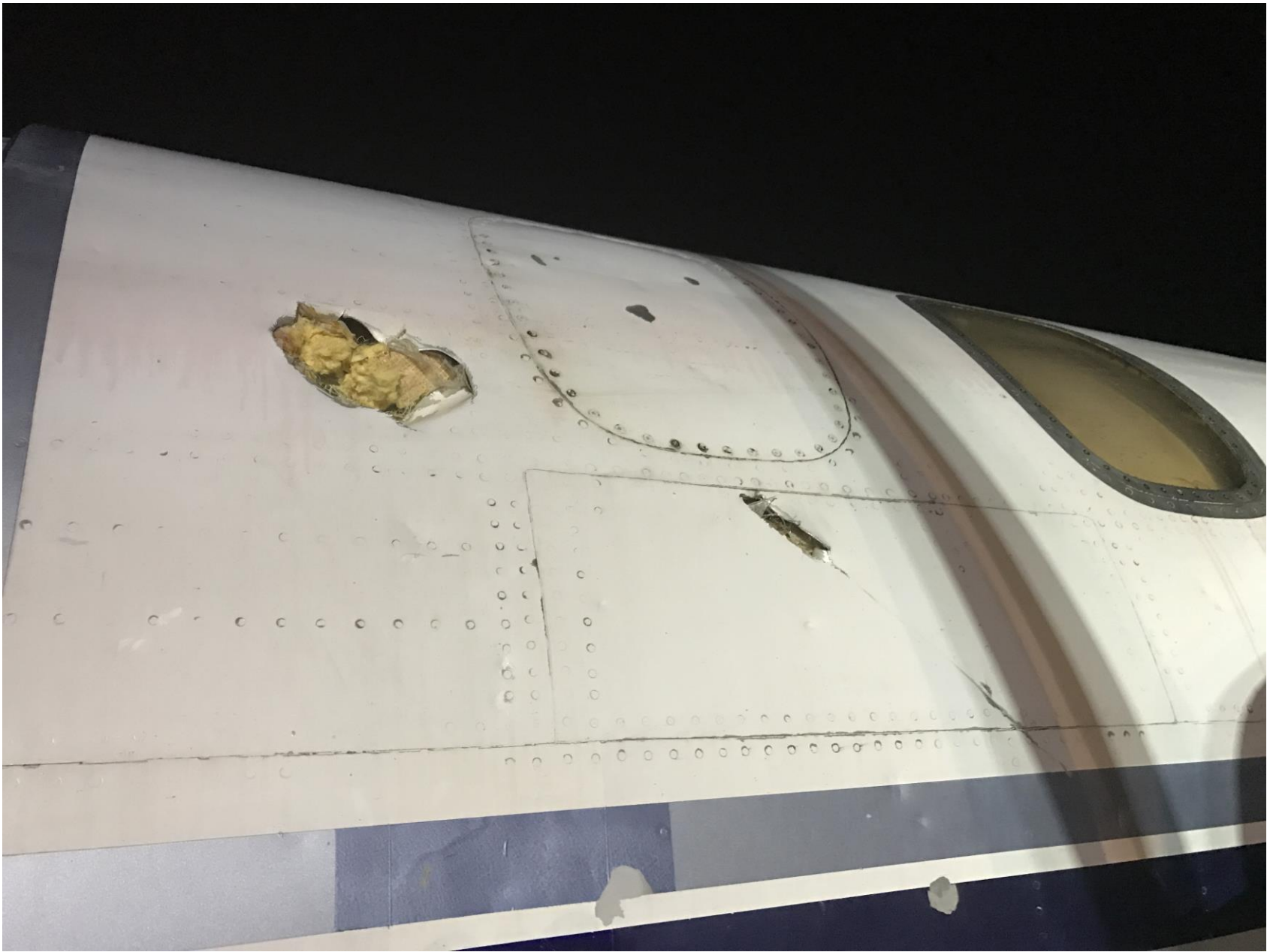
Photo 2 – view of fuselage damage penetration
