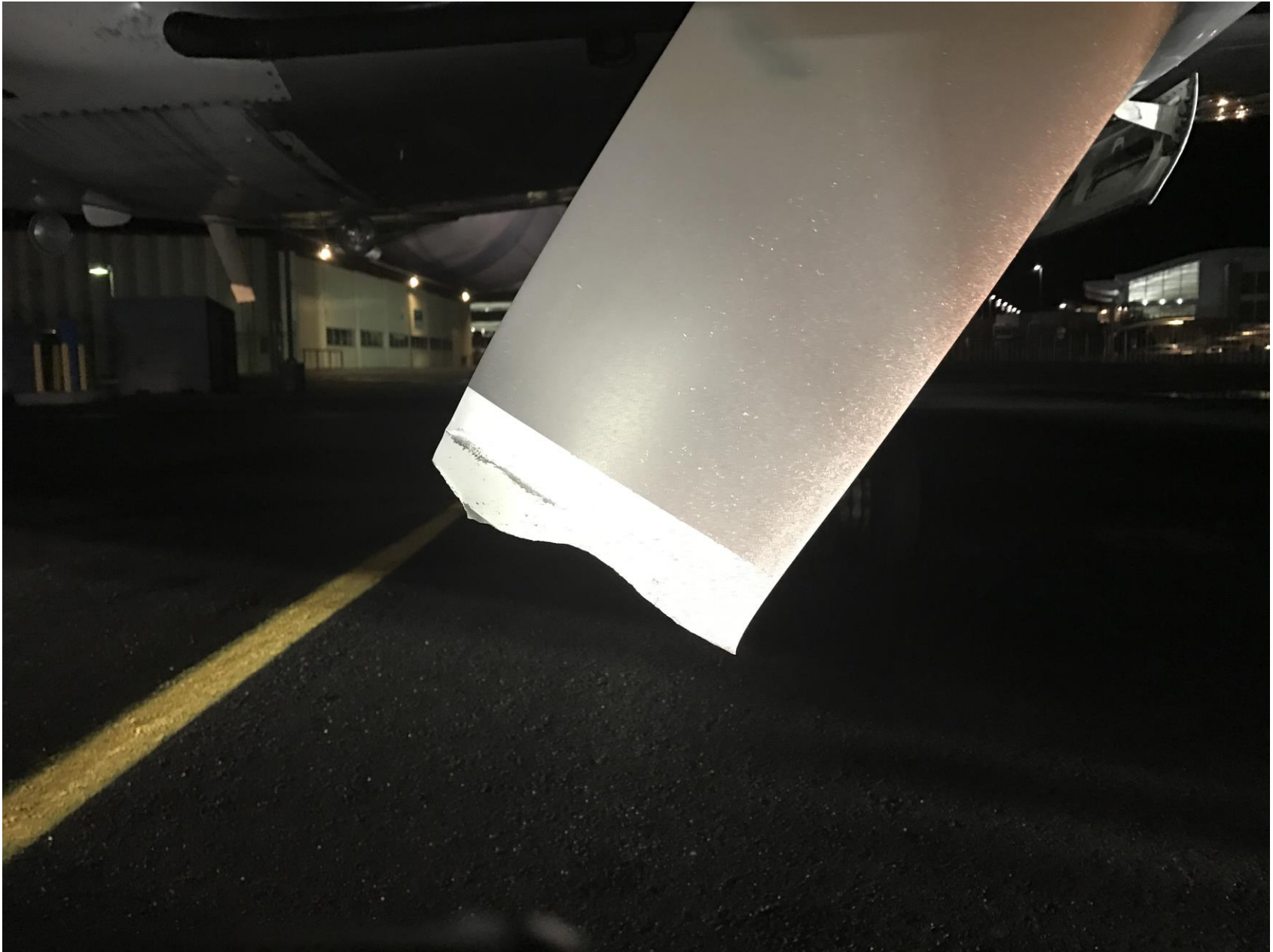
Photo 1 – view of damaged left propeller blade tip
