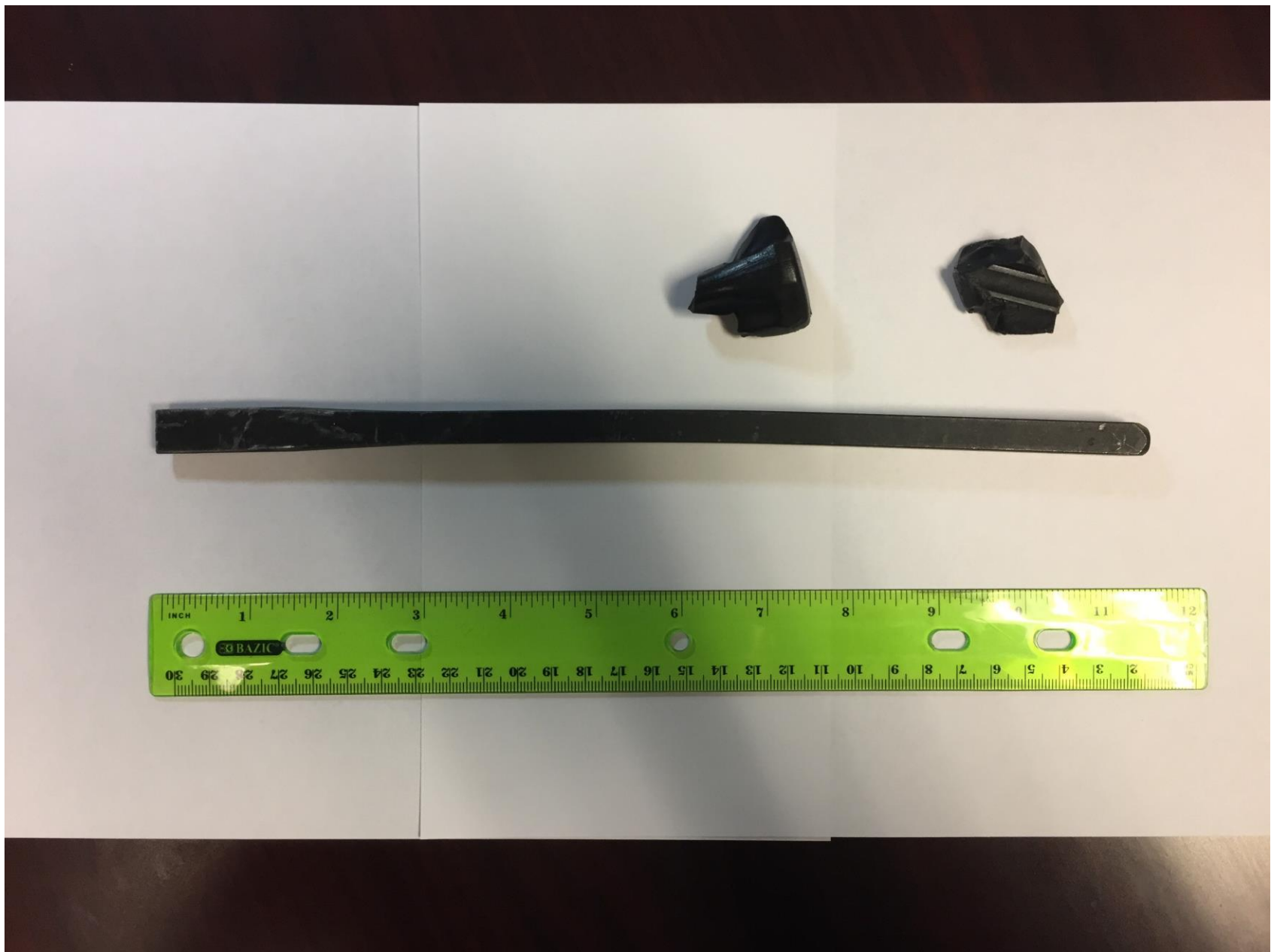
Photo 4 – screwdriver as recovered from departure runway
