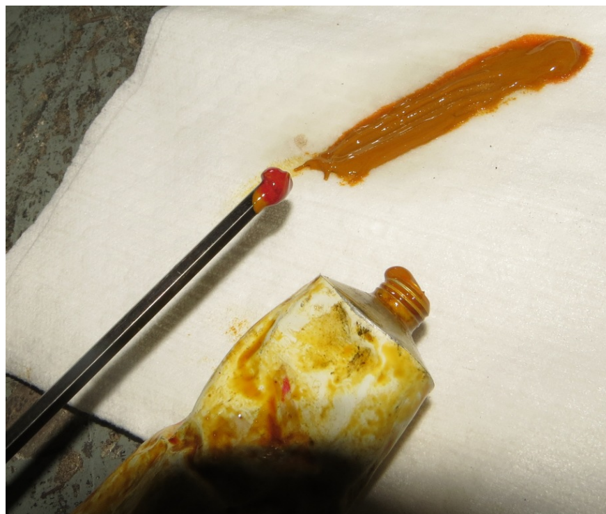
Figure 21 - Positive Water Indication via Water Detecting Paste from Fuel Line Sample
