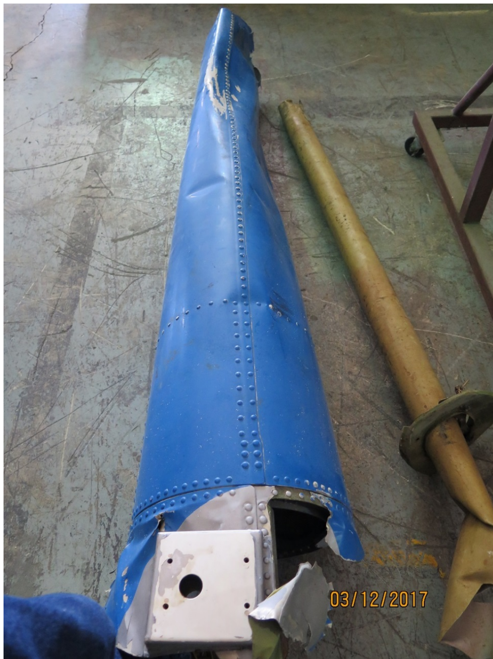
Figure 5 - Recovered Tailboom Section (~FS 197 to ~FS 258)
