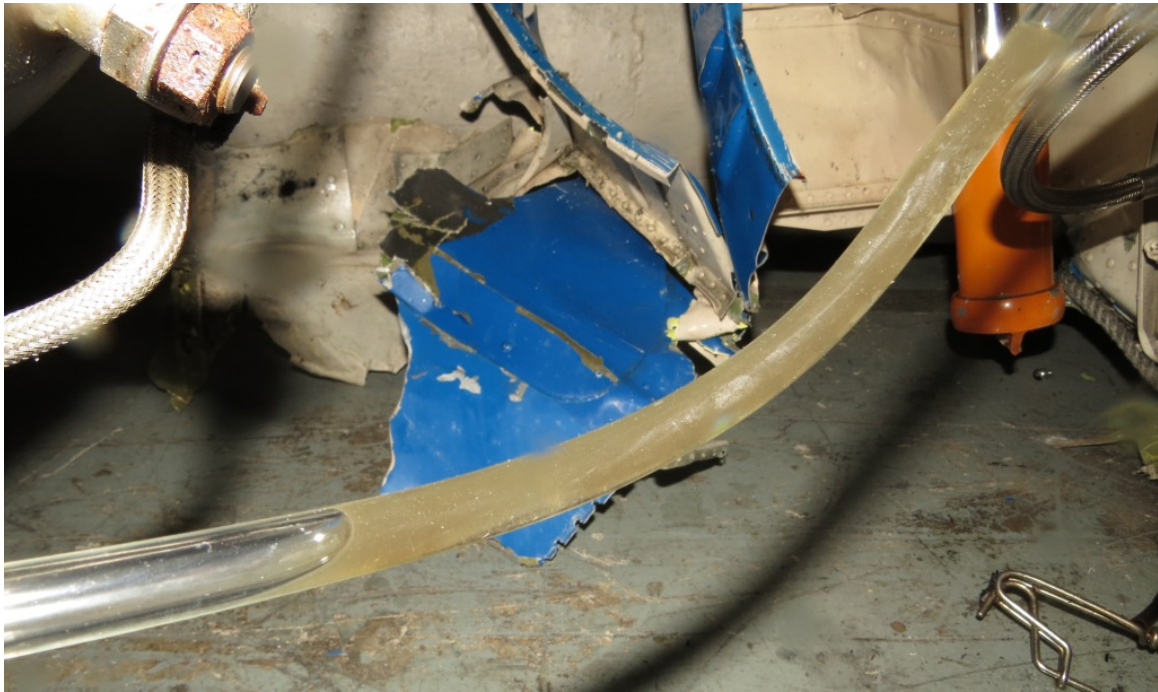
Figure 22 –Fuel/Water Mixture Captured from Fuel Pump Fuel Filter Bowl
