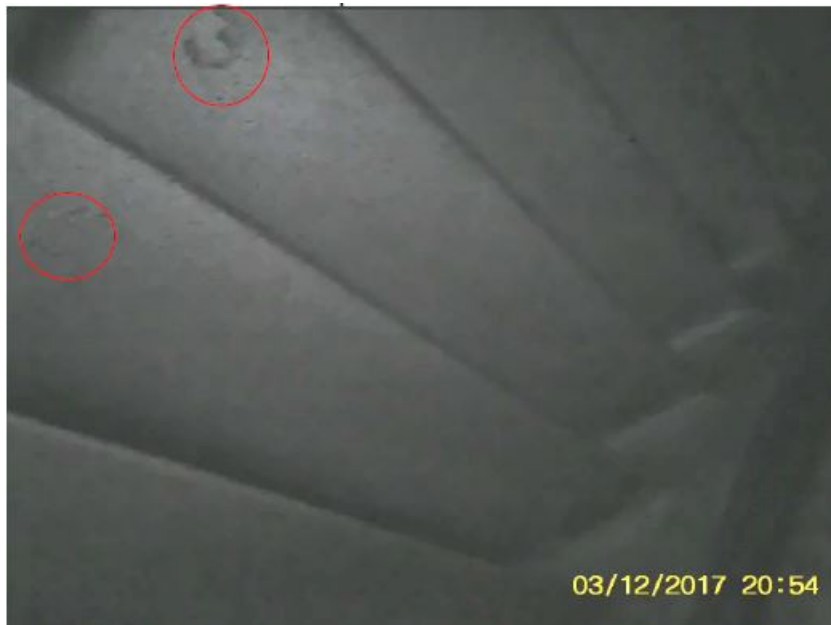
Figure 19 - 4th Stage Turbine with Engraved Serial Numbers Circled
