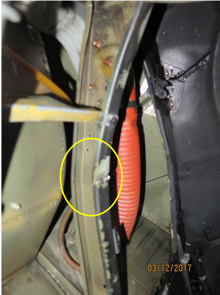
Figure 9 - Damaged Aft Left Mast Support Channel
