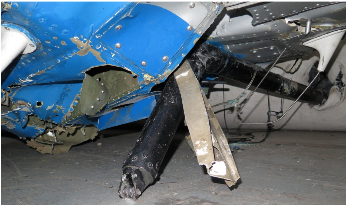
Figure 7 - Landing Gear Strut/Brace Damage
