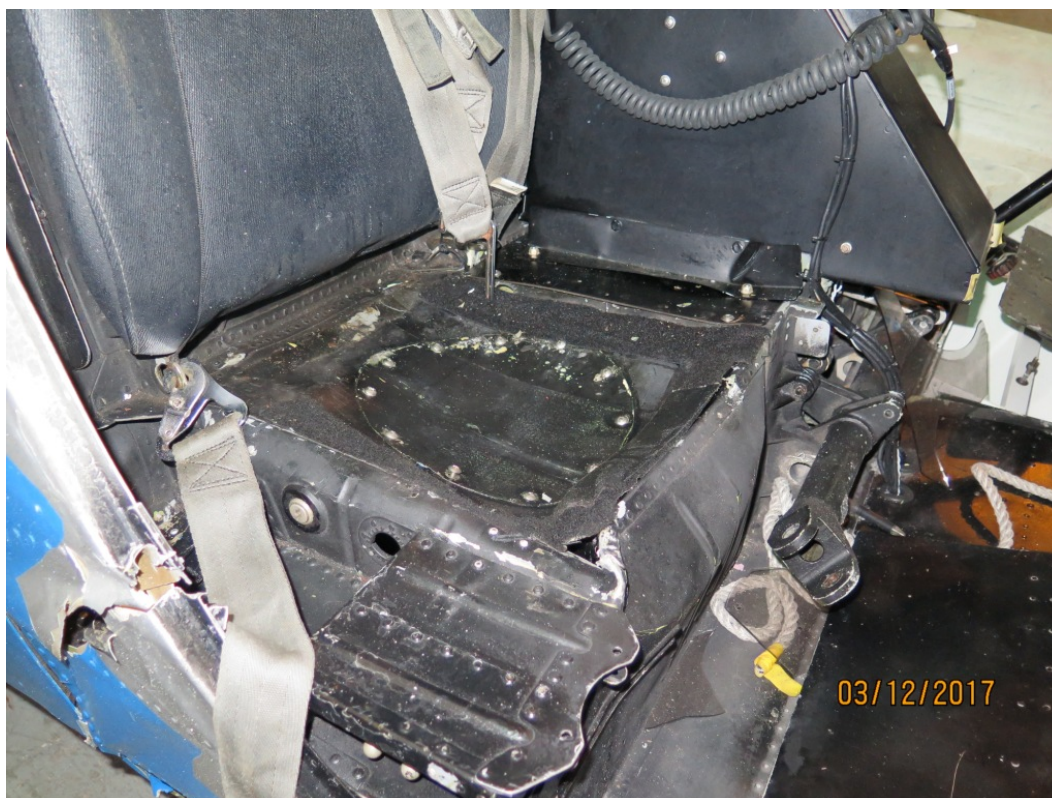
Figure 11 - Crushed Right (Observer) Seat Bottom
