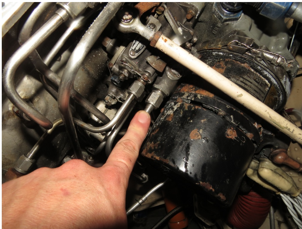
Figure 17 - Small Vacuum Leak Traced to this B-nut at Engine Fuel Control
