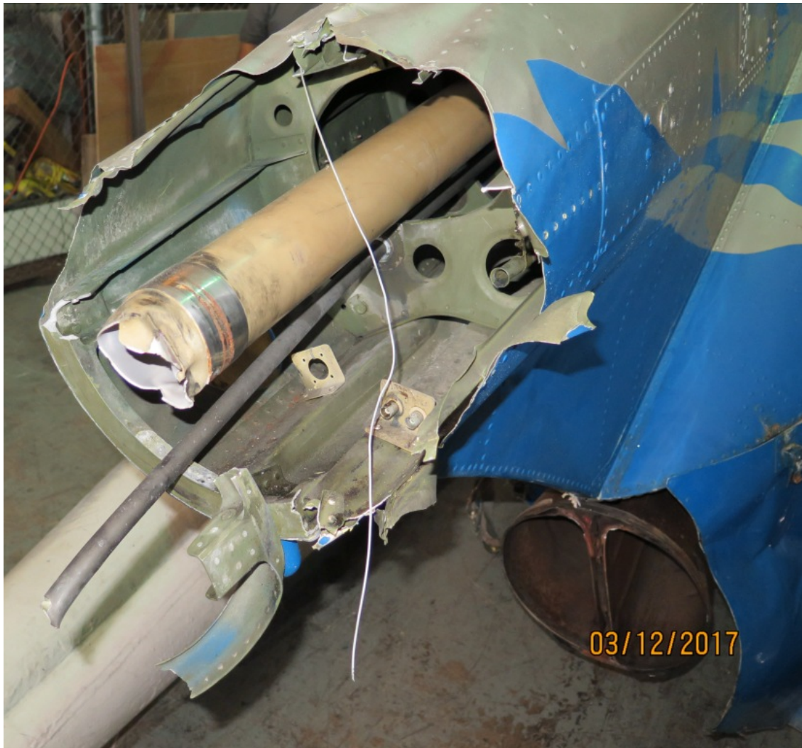
Figure 4 - FS 197.78 Tailboom Separation Location
