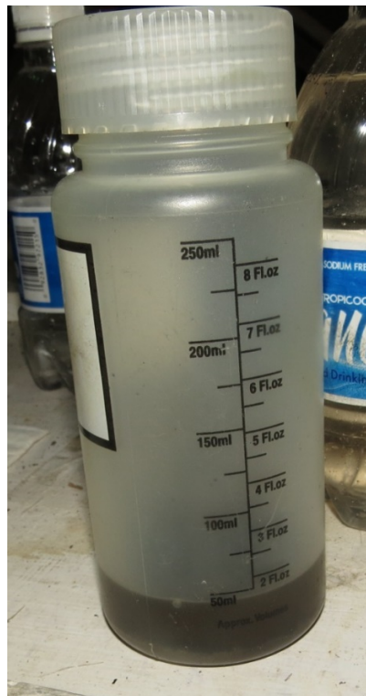
Figure 23 – Fuel/Water Mixture Captured from Fuel Pump Fuel Filter Bowl
