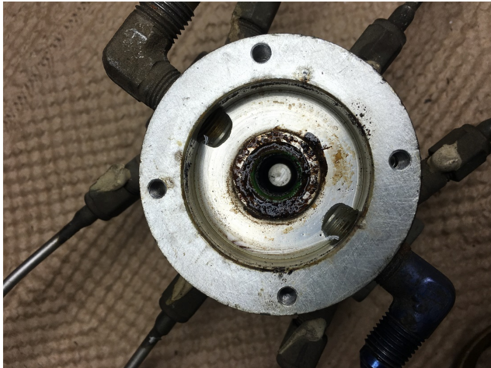
Figure 9: Fuel Manifold Valve Lower Housing
