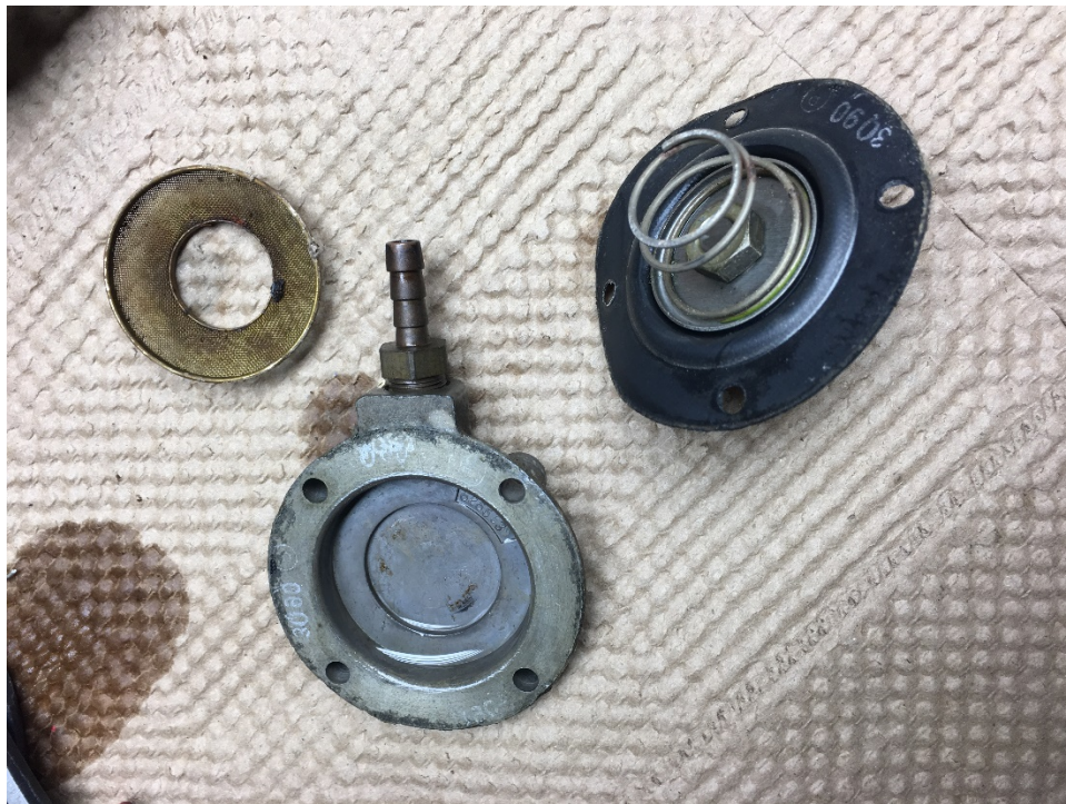
Figure 11: Manifold Valve "Dry" Section
