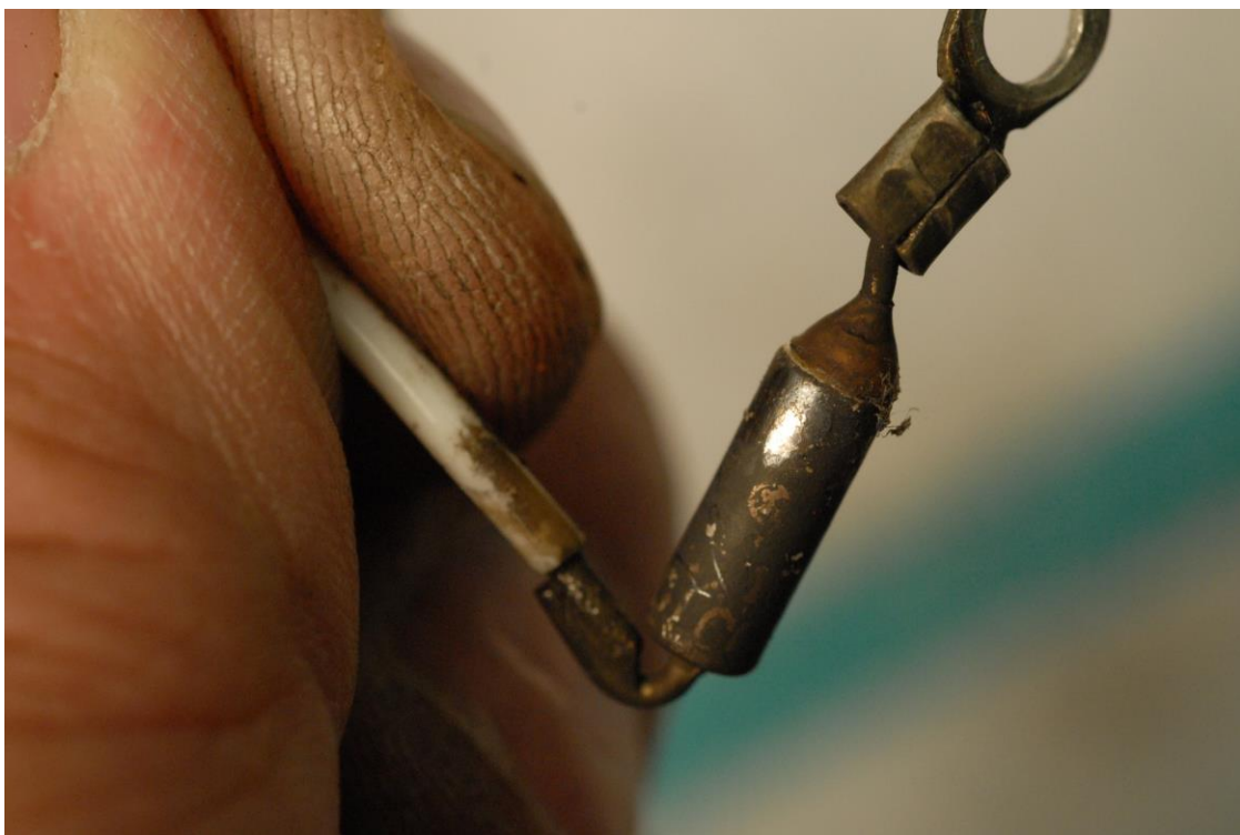
2C27-1 4H234 31Aug17_076 - Contact Mark from Armature Rubbing Thermal Fuse
