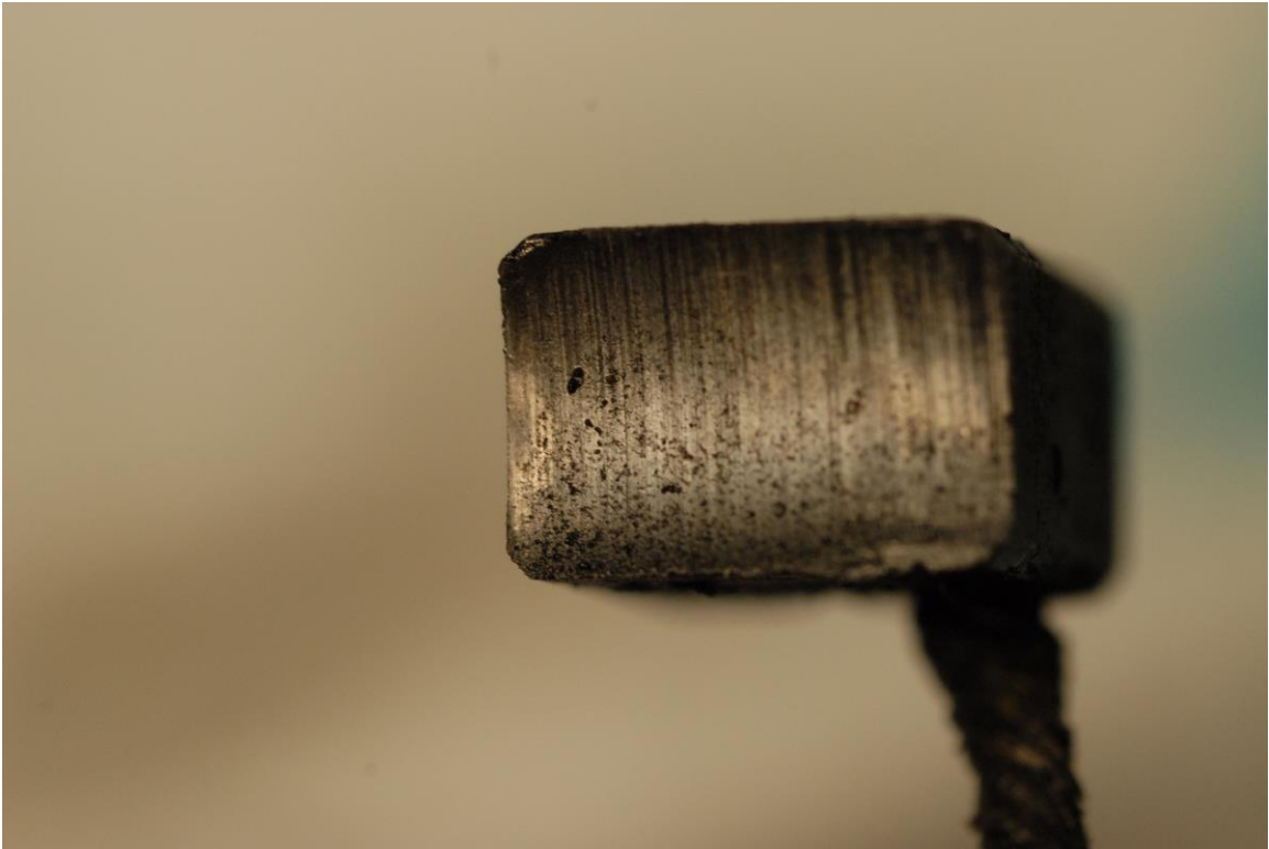
2C27-1 4H234 31Aug17_037 - Motor Brush Wear Pattern - OK
