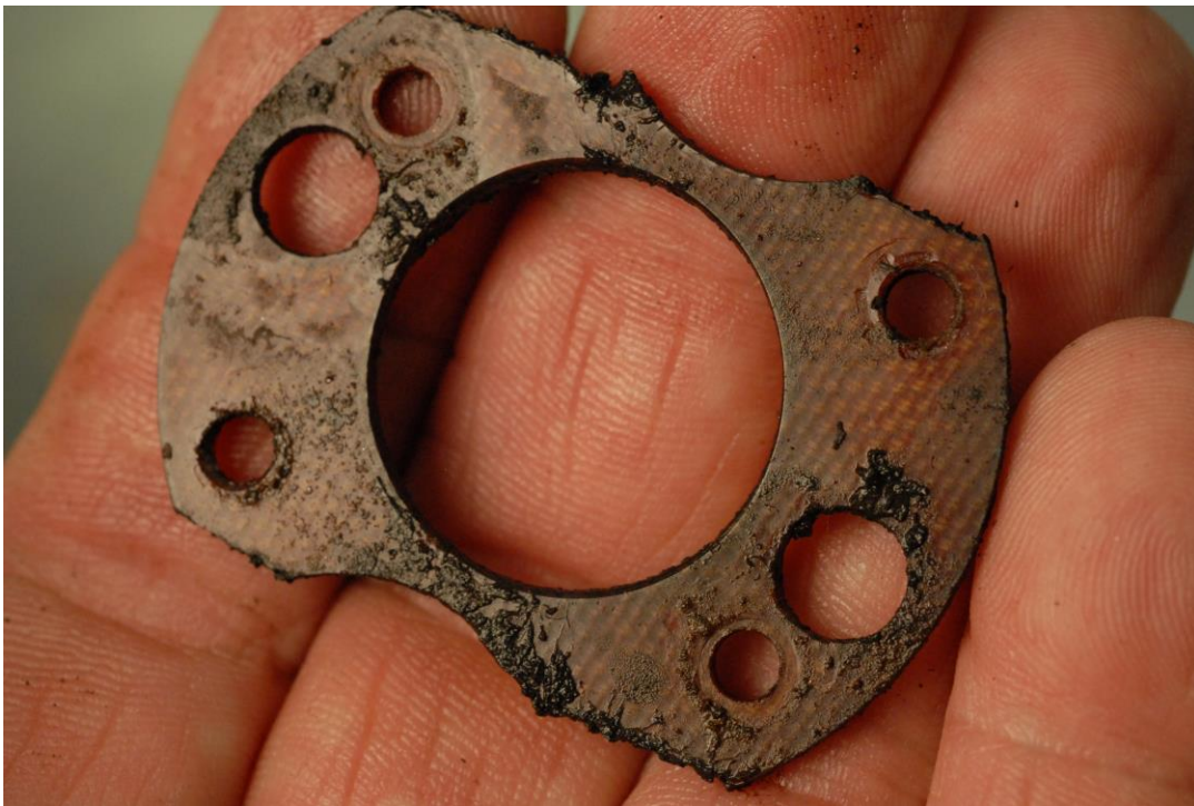
2C27-1 4H234 31Aug17_032 - Brush Card Phenolic Insulator
