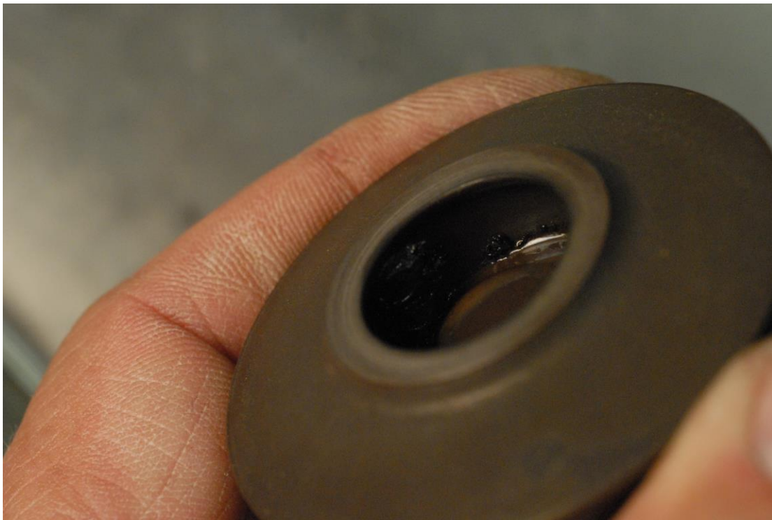
2C27-1 4H234 31Aug17_072 – Debris across 1 st Impeller Blade Inlet
