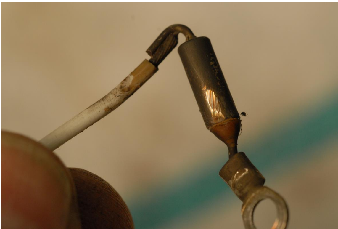
2C27-1 4H234 31Aug17_077 - Contact Mark from Armature Rubbing Thermal Fuse
