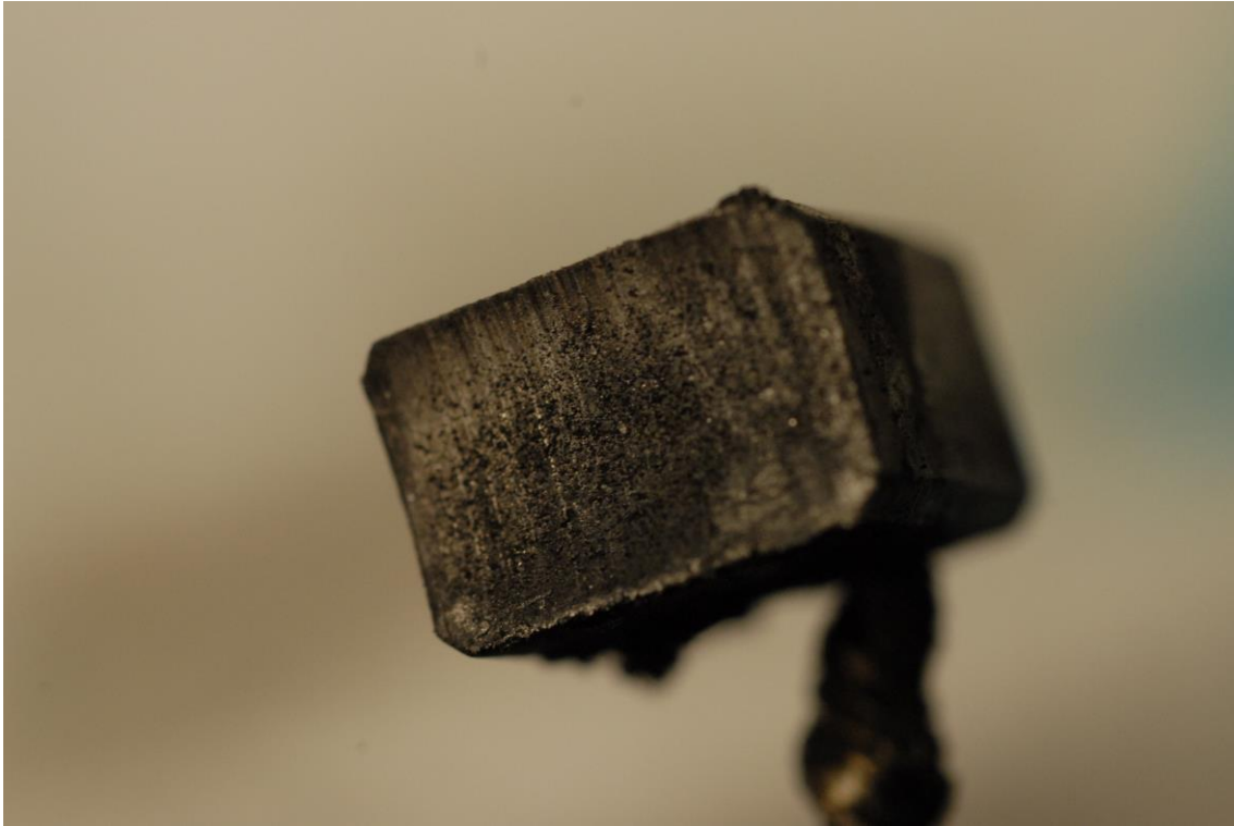
2C27-1 4H234 31Aug17_039 - Motor Brush Signs of Arcing
