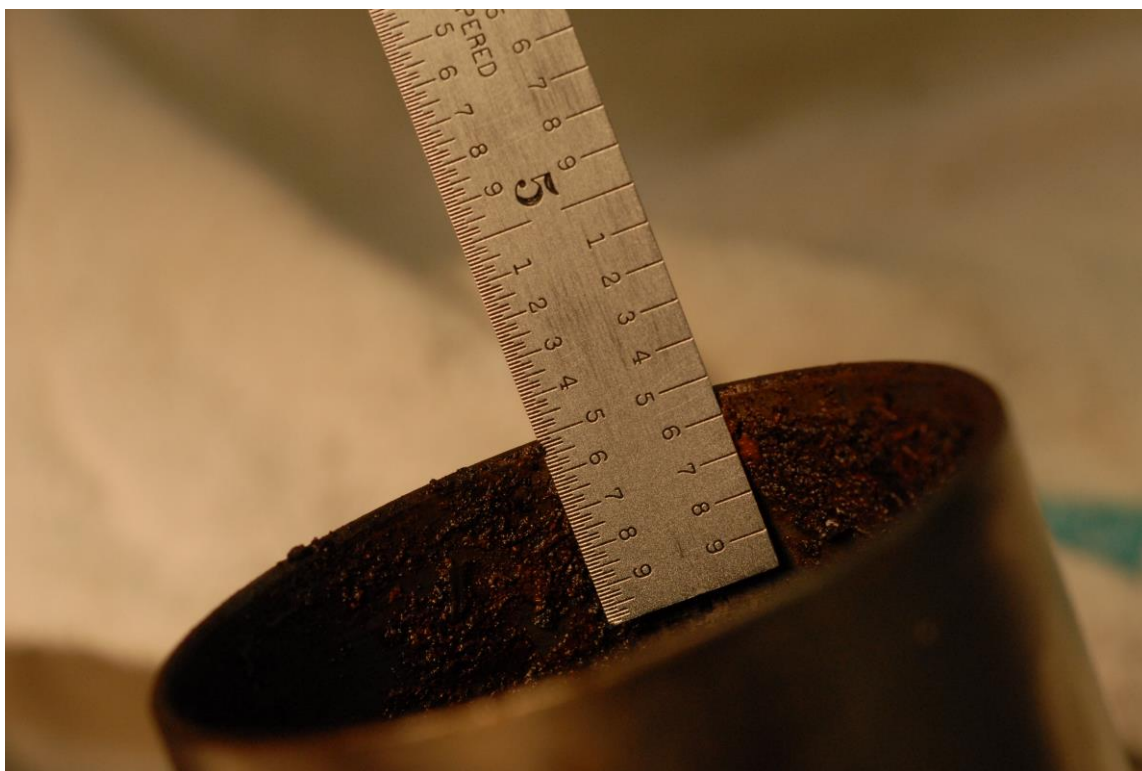
2C27-1 4H234 31Aug17_043 – Field Tube Heavy Corrosion
