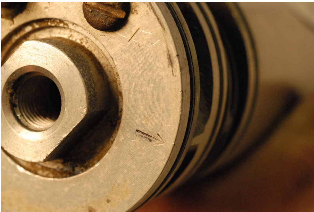
2C27-1 4H234 31Aug17_021 - Cartridge Clocking Mark
