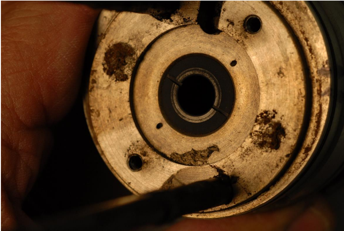
2C27-1 4H234 31Aug17_079 - Debris on Pump Housing
