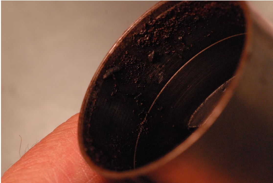
2C27-1 4H234 31Aug17_047 – Field Tube Heavy Corrosion
