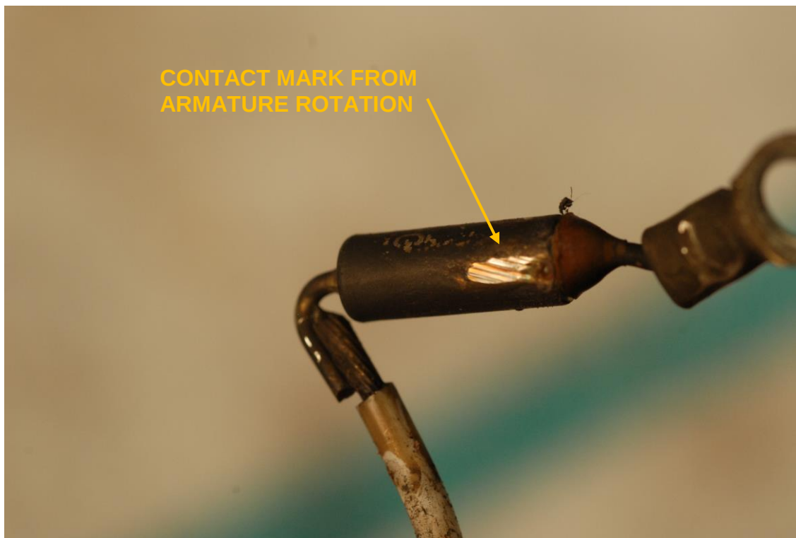
2C27-1 4H234 31Aug17_075 - Contact Mark from Armature Rubbing Thermal Fuse
