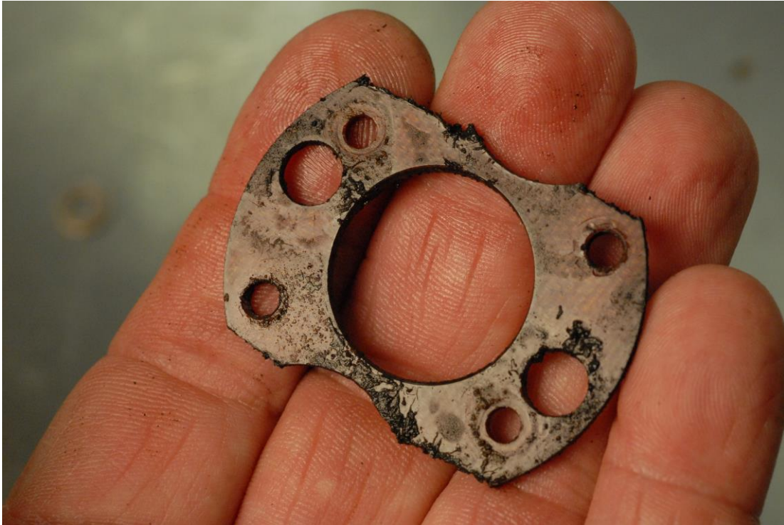
2C27-1 4H234 31Aug17_031 – Brush Card Phenolic Insulator
