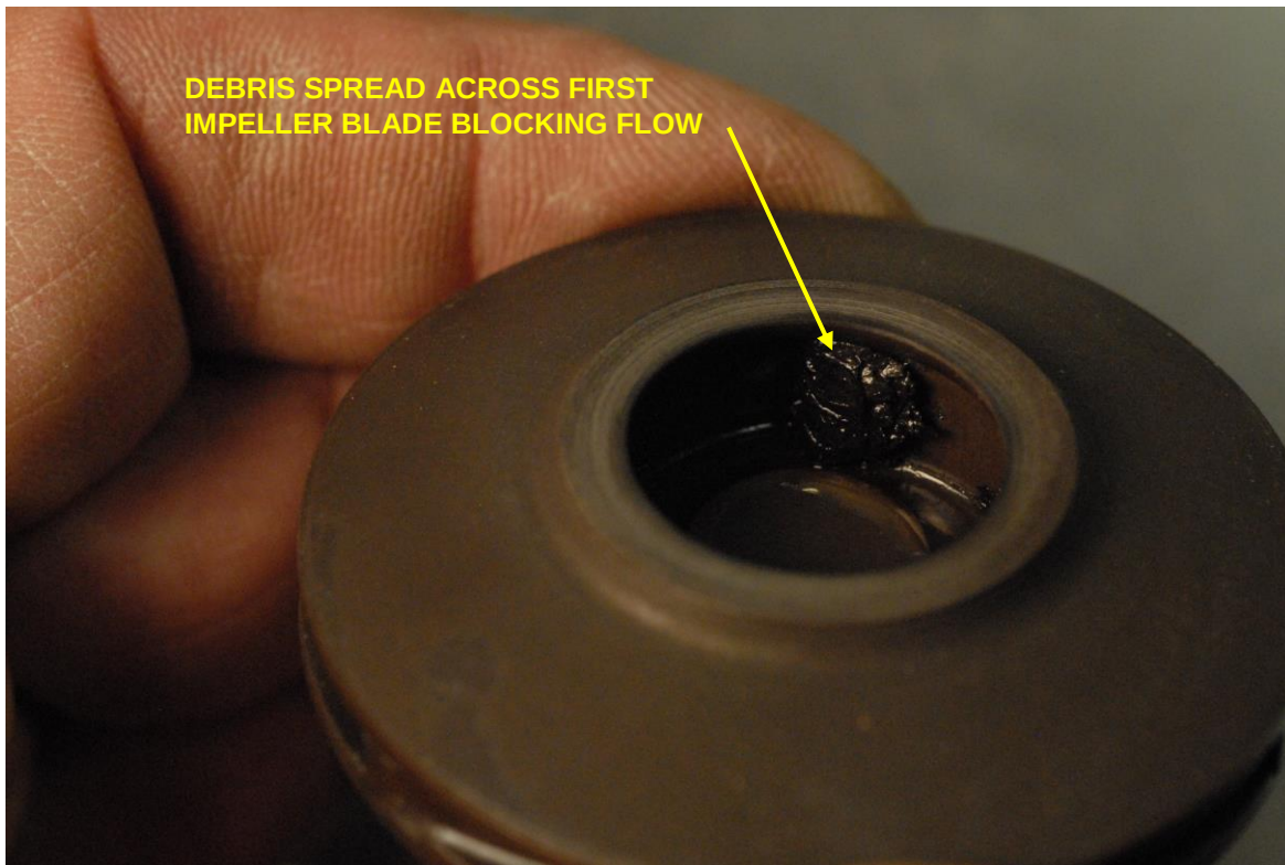
2C27-1 4H234 31Aug17_071 – Debris across 1 st Impeller Blade Inlet
