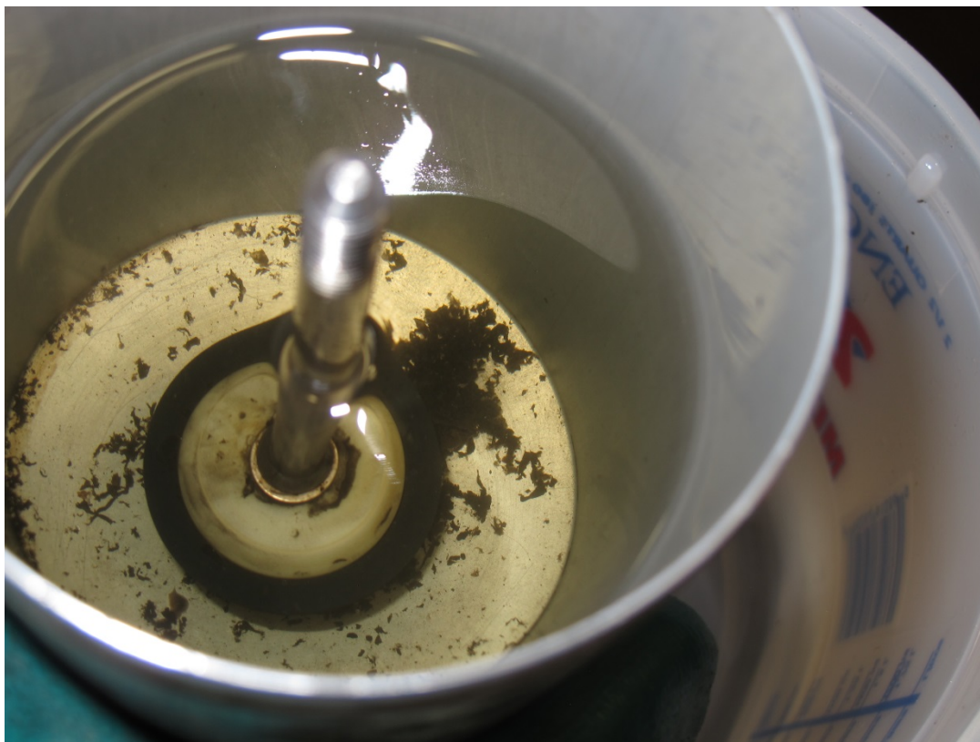
Figure 8. Debris in Aircraft Mounted Fuel Filter Bowl
