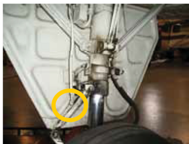
Squat switch disconnect point
